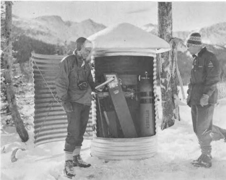
Figure 33. Fall Creek gaging station. The gas purged servo-manometer gaging station is shown.
