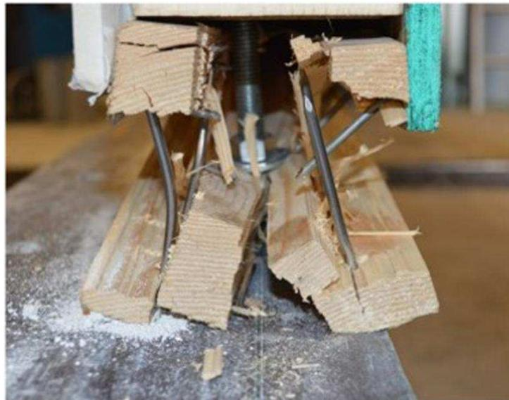
**Figure 3.13:** Commonly observed failure with Wall Types C and D due to the wood splitting around the anchor bolt.
