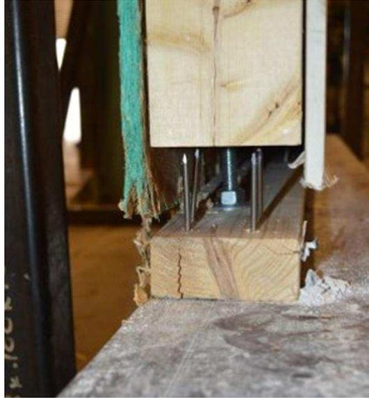
**Figure 3.12:** Commonly observed failure with Wall Types A and B due to nail withdrawal.
