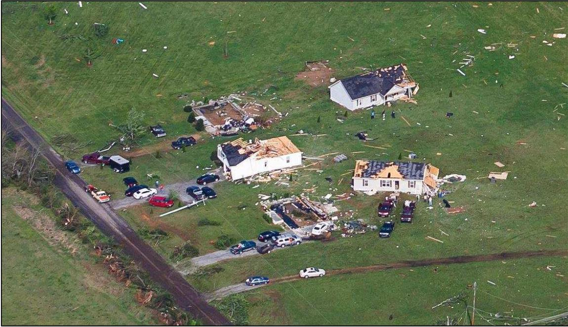
**Figure 1.5:** Two homes translated off their foundation due to inadequate wall-to-foundation connections during the April 28, 2014 Flintville, TN tornado (courtesy of SellersPhoto 2014).
