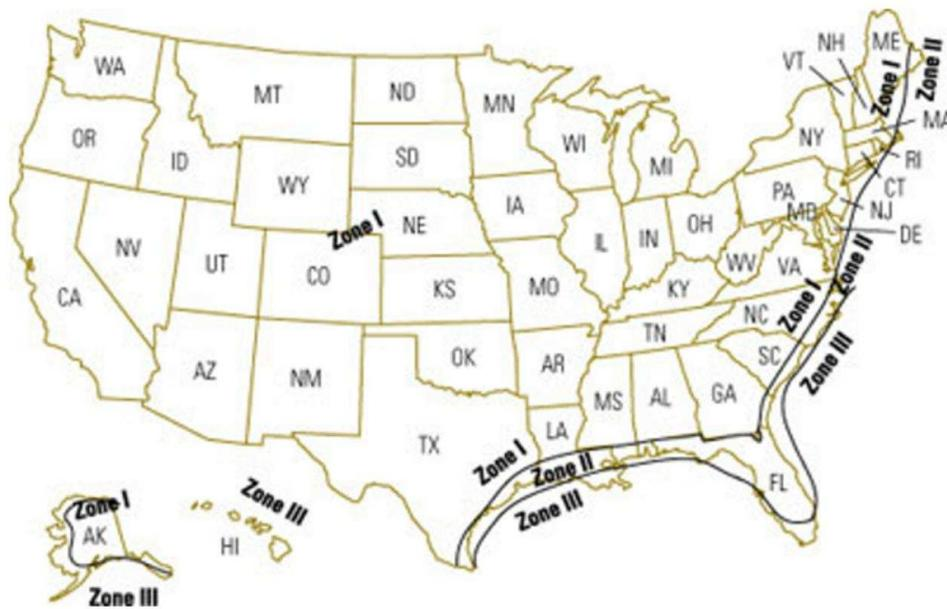
**Figure 5.4:** Basic wind zone map for manufactured homes. Image courtesy of the Manufactured Housing Institute (MHI 2016).
