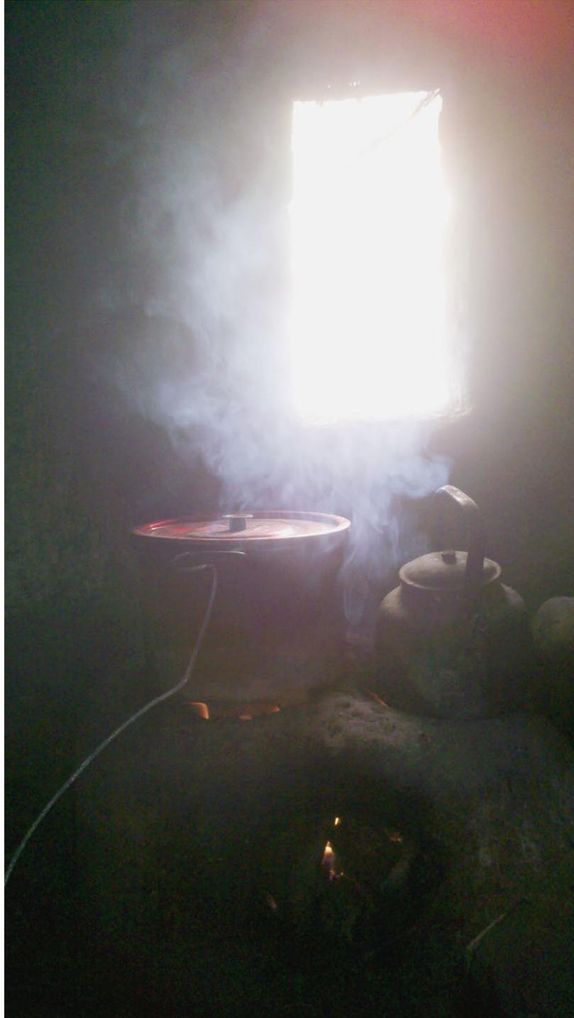
FIGURE 2. Traditional dung-burning stove from the Melgar province in the High Andes of Peru. Stoves are hand-built from adobe and are typically operated in small, poorly ventilated huts.
