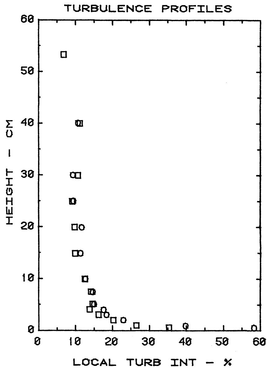
Figure 16. Velocity and Turbulence Profiles Utilized with Negatively Buoyant Plume (LNG)
