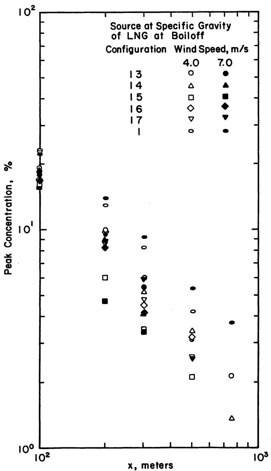
Figure 23. Peak Concentration vs. x (LNG Plume)
