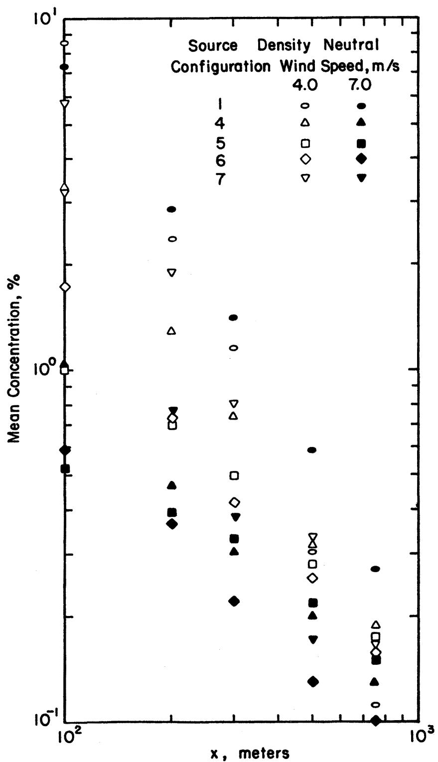
Figure 17. Mean Concentration vs. x (Neutral Density Plume)
