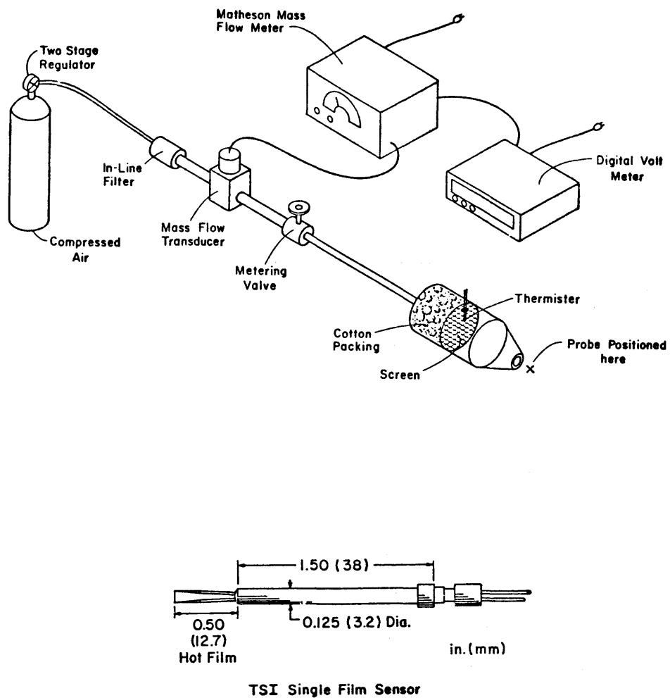
Figure 5. Velocity Probes and Velocity Standard
