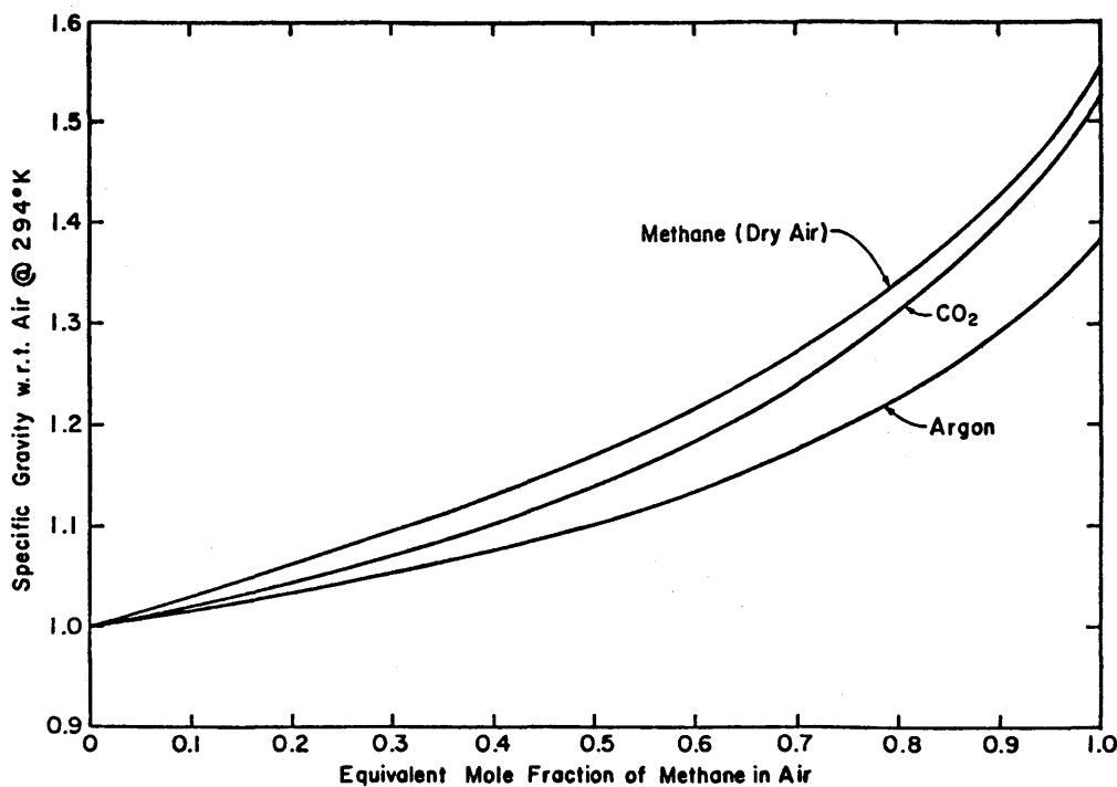
Figure 2. Specific Gravity of Gas-Air Mixtures
