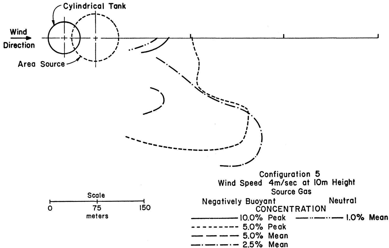
Figure 33. Concentration Isopleths for Configuration 5 and Wind Speed 4 m/sec
