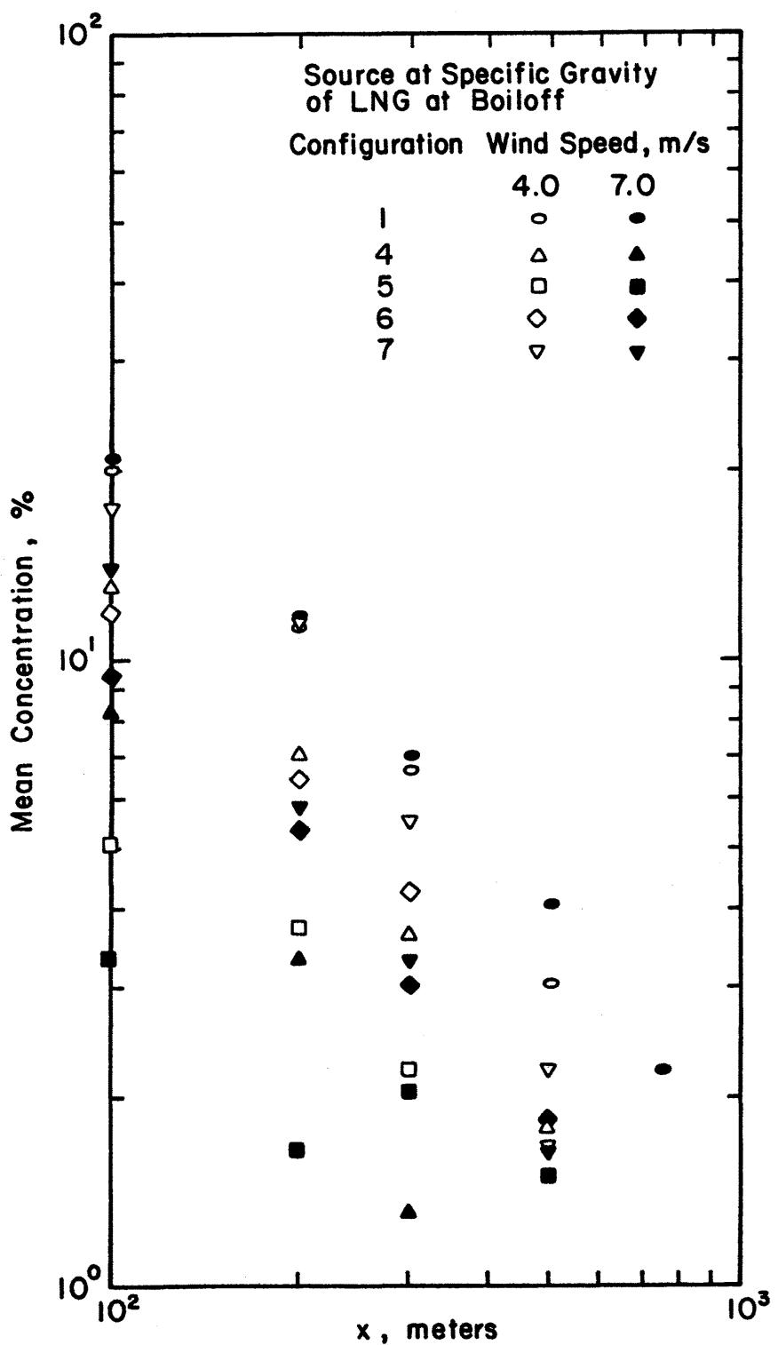
Figure 25. Mean Concentration vs. x (LNG Plume)
