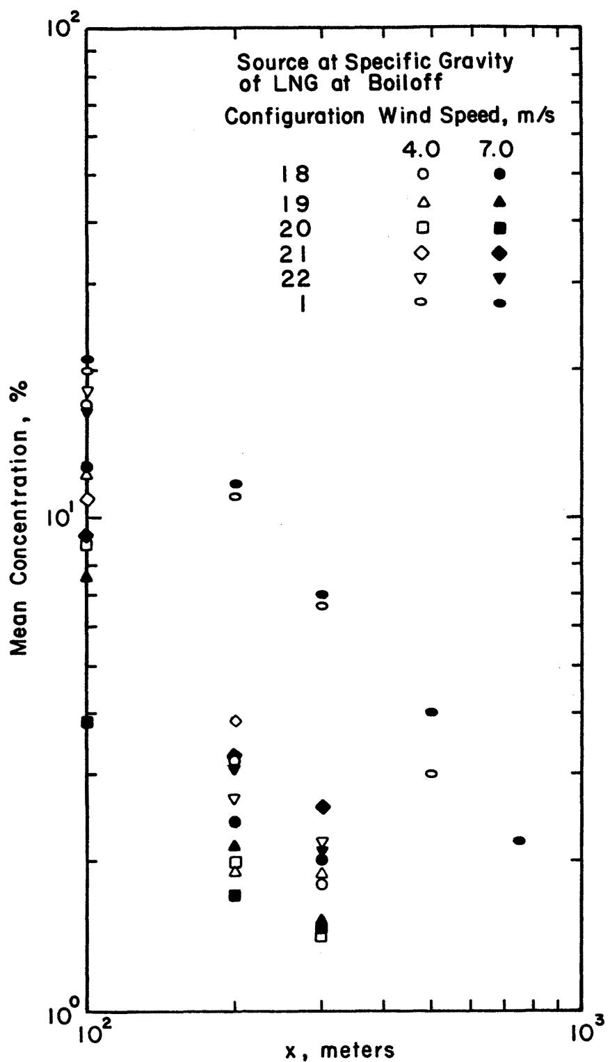
Figure 28. Mean Concentration vs. x (LNG Plume)
