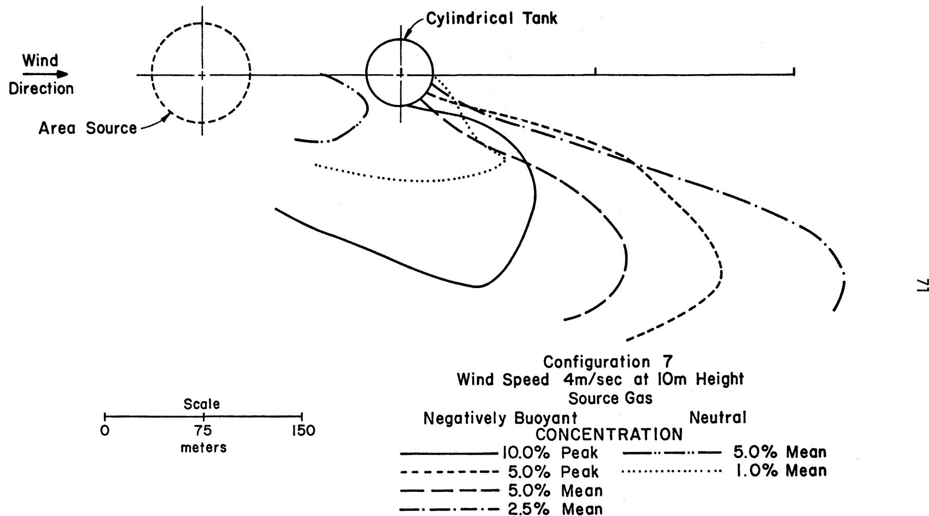
Figure 37. Concentration Isopleths for Configuration 7 and Wind Speed 4 m/sec
