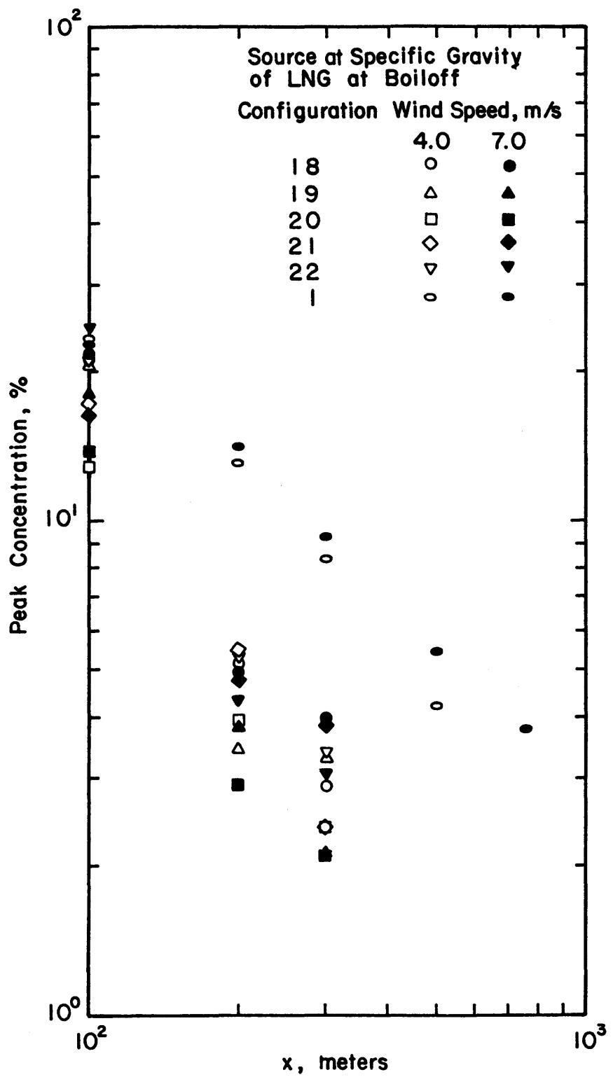
Figure 24. Peak Concentration vs. x (LNG Plume)
