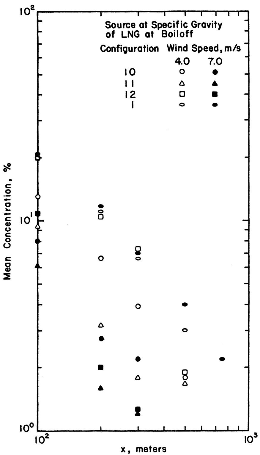
Figure 26. Mean Concentration vs. x (LNG Plume)
