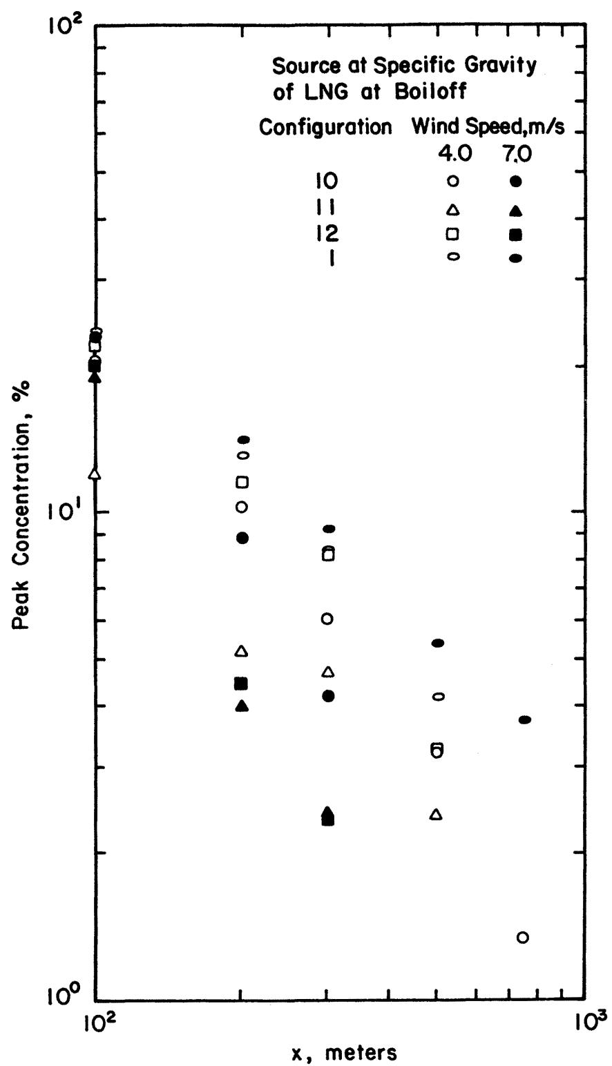
Figure 22. Peak Concentration vs. x (LNG Plume)
