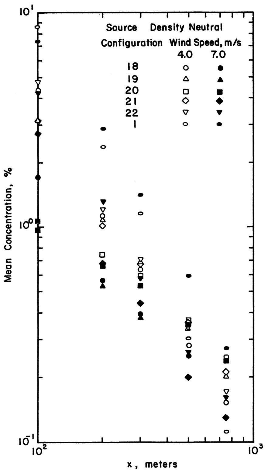
Figure 20. Mean Concentration vs.  $x$  (Neutral Density Plume)
