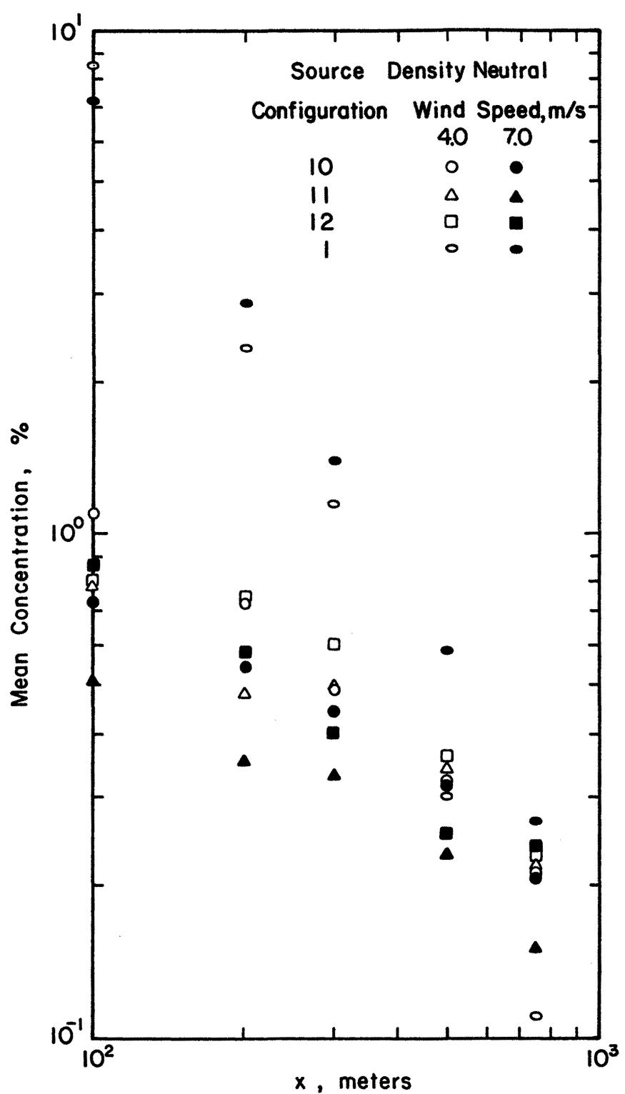
Figure 18. Mean Concentration vs. x (Neutral Density Plume)
