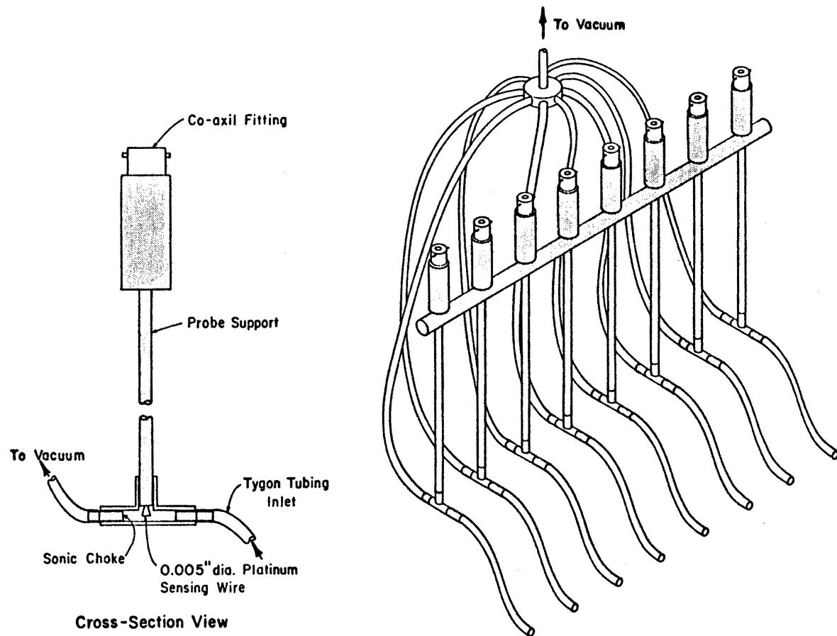
Figure 7. Hot-Wire Katharometer Probes
