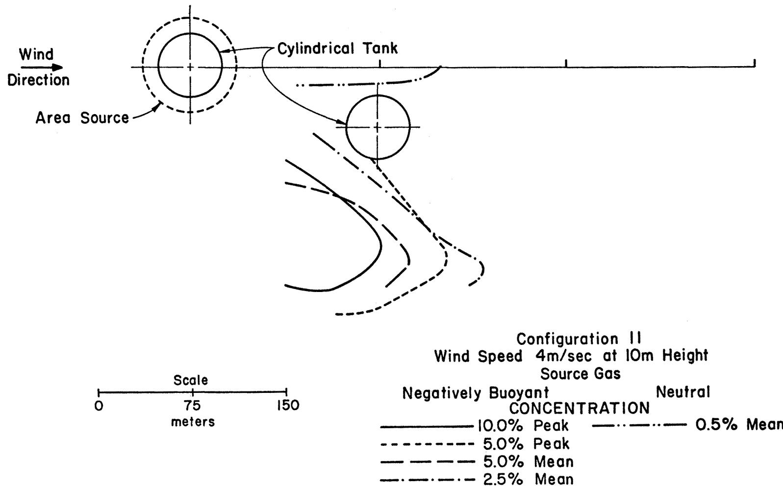
Figure 41. Concentration Isopleths for Configuration II and Wind Speed 4/sec
