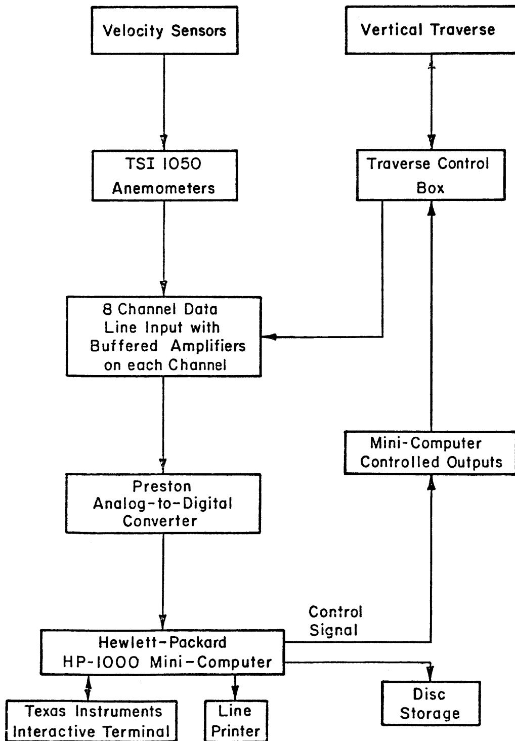
Figure 6. Velocity Data Reduction Flowchart
