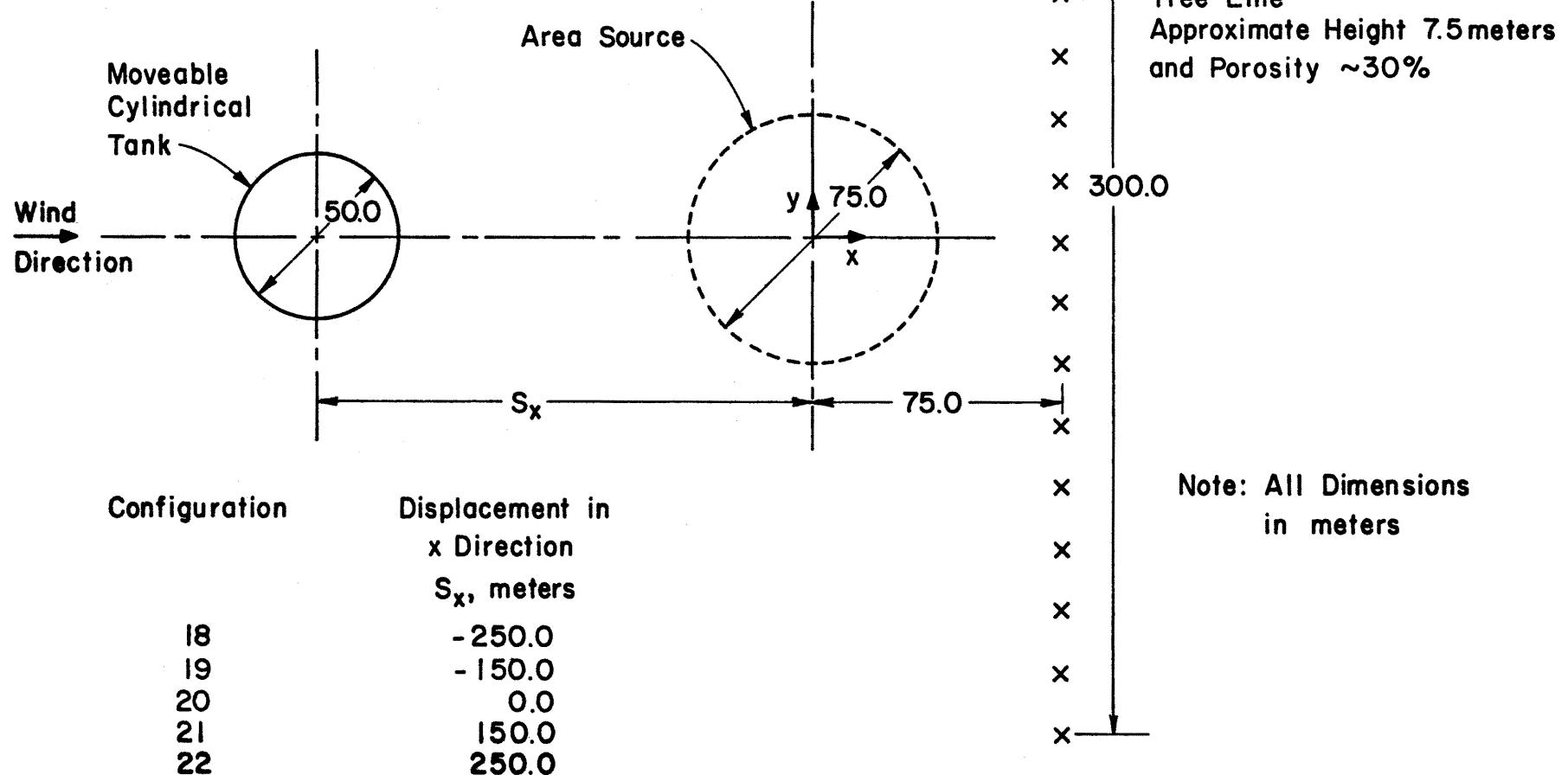
Figure 14. Configurations 18 to 22 Identification
