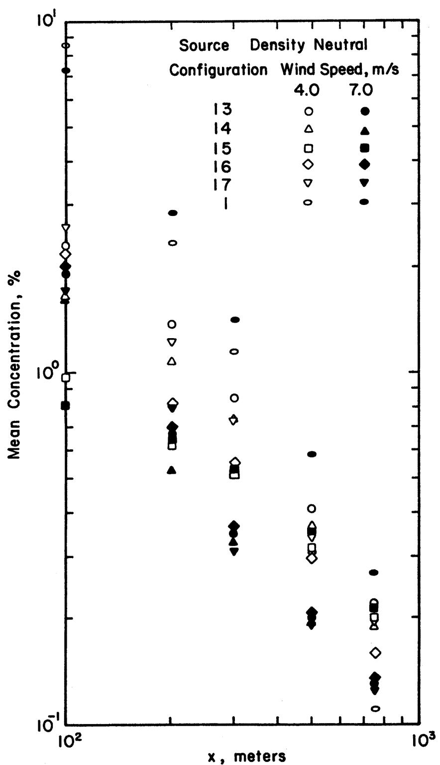
Figure 19. Mean Concentration vs.  $x$  (Neutral Density Plume)
