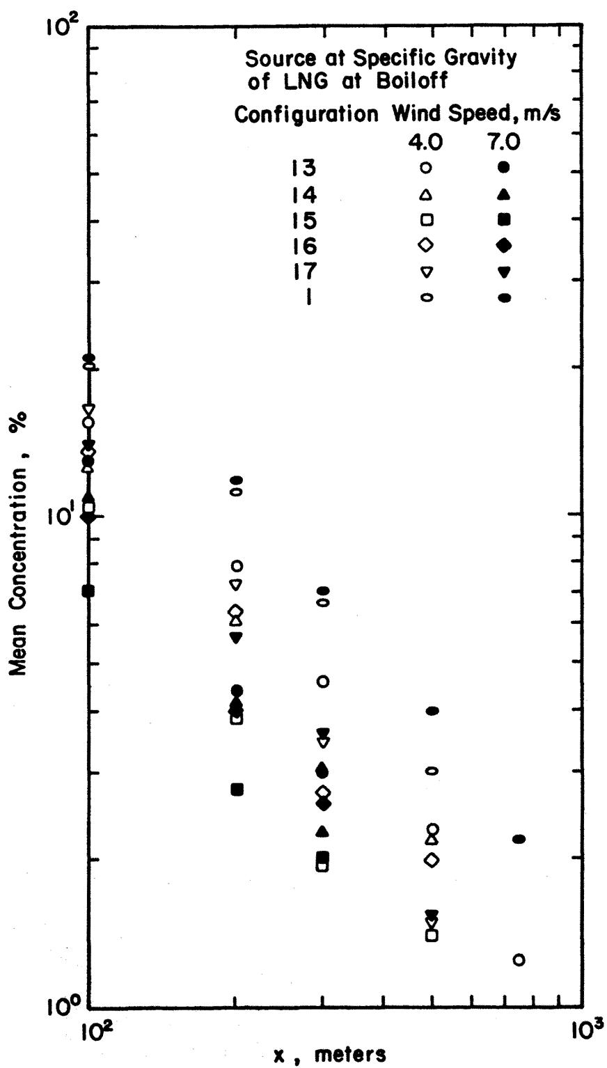
Figure 27. Mean Concentration vs. x (LNG Plume)
