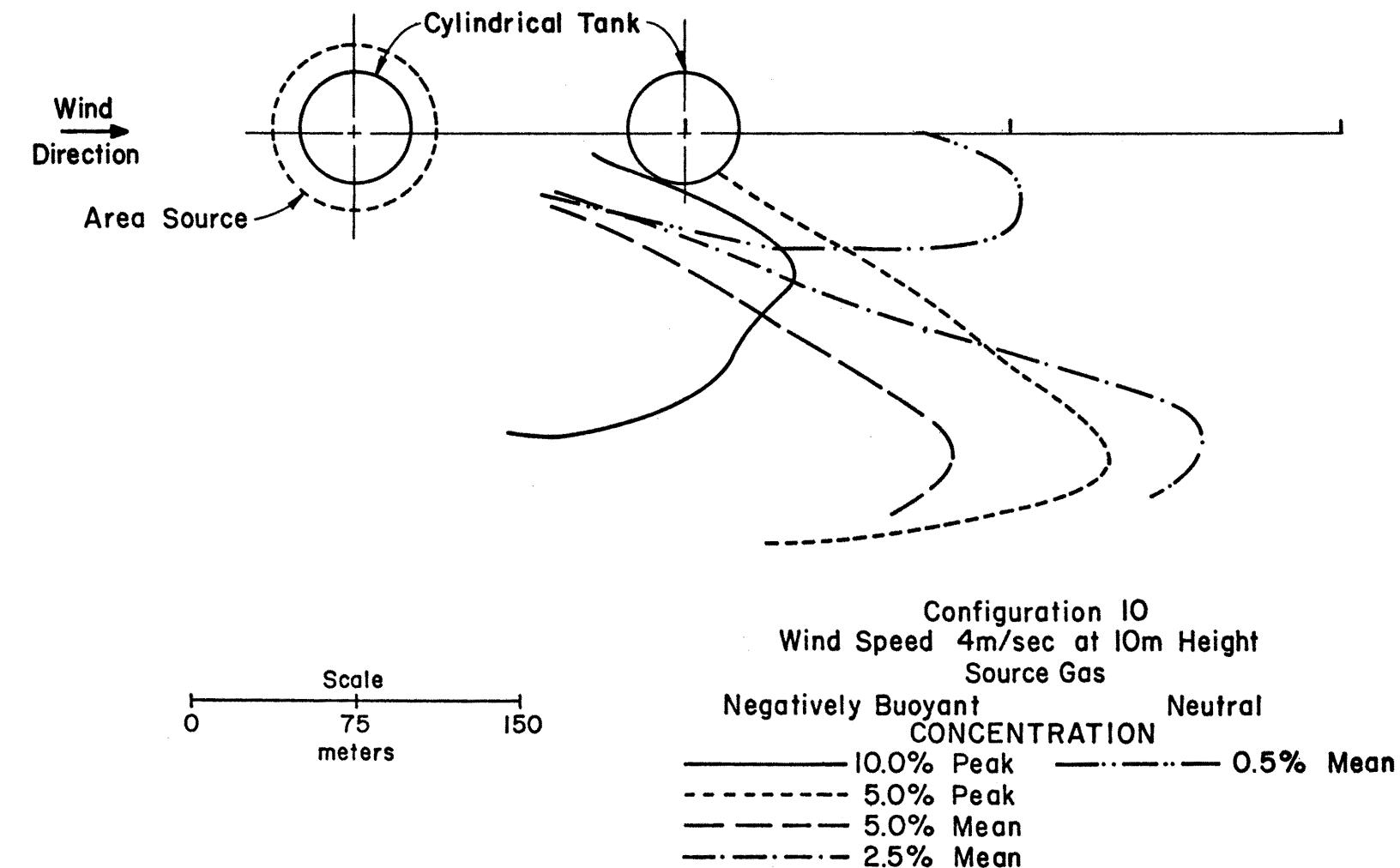
Figure 39. Concentration Isopleths for Configuration 10 and Wind Speed 4 m/sec
