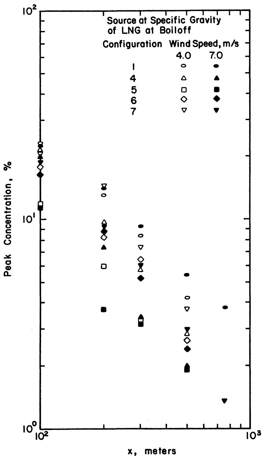
Figure 21. Peak Concentration vs. x (LNG Plume)
