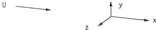
The  $x$  axis is horizontal along the main air stream down the wind tunnel;  $y$  is vertical, normal to the mean flow;  $z$  is horizontal, normal to the mean flow. The origin is 48" downstream from the entrance to the wind tunnel test section and 12" from each wall of the tunnel. The cylinder's center coincides with the origin and its axis is along the vertical  $y$  axis.
