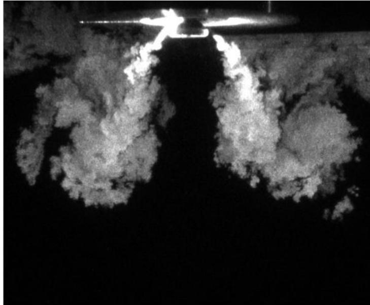
*Figure 1.22: Fuel jet penetration and mixing for low pressure injection [85].*
