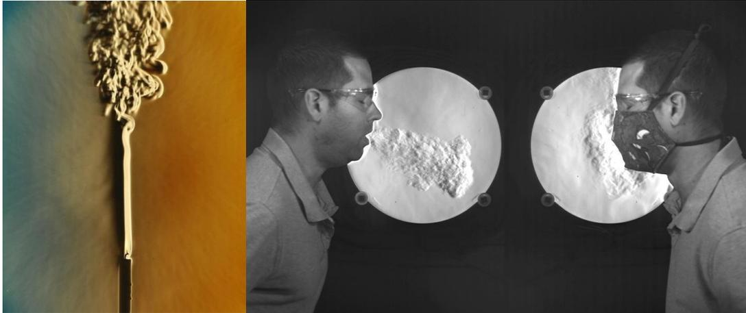
*Figure 1.14: The plume from an ordinary candle transitions from laminar to turbulent flow in this Schlieren photograph [55] (left), and NIST scientist Matthew Staymates used schlieren photography to qualitatively, and graphically, show the difference in how far a plume of breath can spread with and without a face covering (right) [56], [57].*
