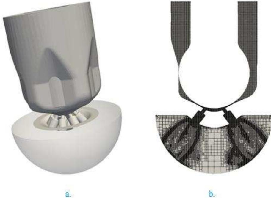
*Figure 2.20: (a) Eulerian nozzle flow CFD domain for the ECN's Spray-G injector, and (b) numerical grid on the centerline at full needle lift.*
