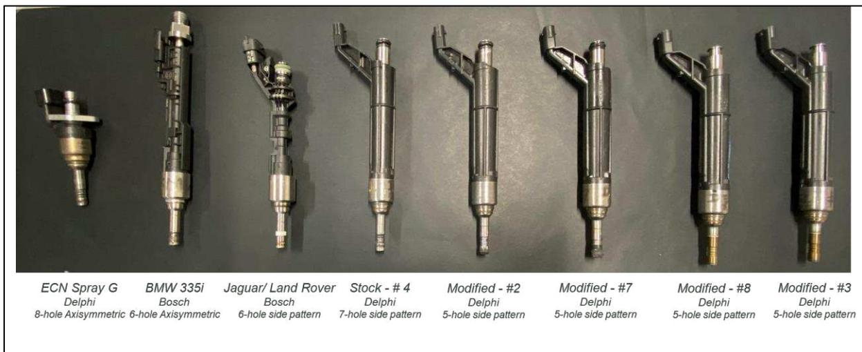
*Figure 2.2: Various injectors, and their manufacturer and hole pattern, tested in the spray chamber for injection testing.*
