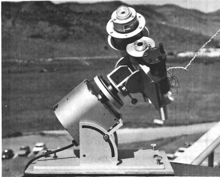
Figure 3. Instrumentation used for the determination of cloud optical depth.
