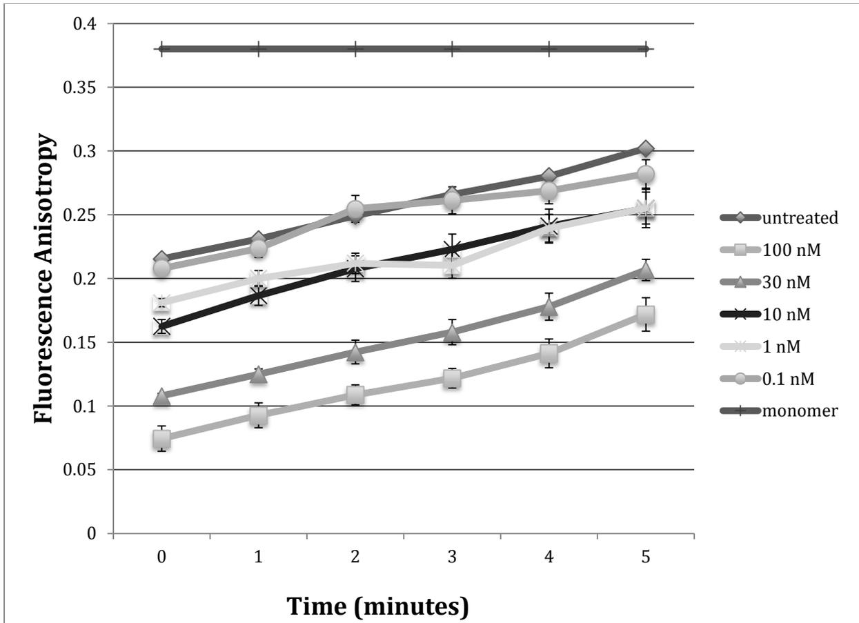
Figure 13: Fluorescence anisotropy upon fluorescence photobleaching for 5 minutes at at vary in concentration of hCG. According to (Chakraborty & Chattopadhyay, 2015), the difference between the monomer anisotropy and extrapolated anisotropy for each condition provides information on the cluster size of LH receptors in plasma membrane. Data shown in tables from tables 1-6
