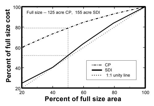
Figure 14. Center pivot sprinkler (CP) and SDI system costs as related to field size. (after O'Brien et al., 1997)
