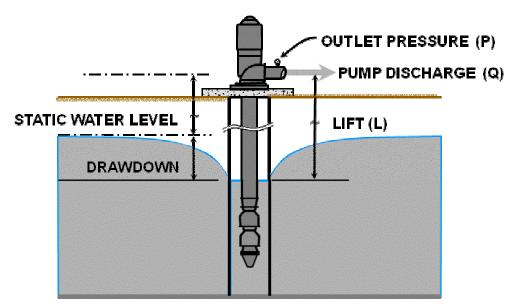
Figure 1. Schematic of factors affecting the pumping plant performance of a deep well turbine pump powered by an electric motor.
