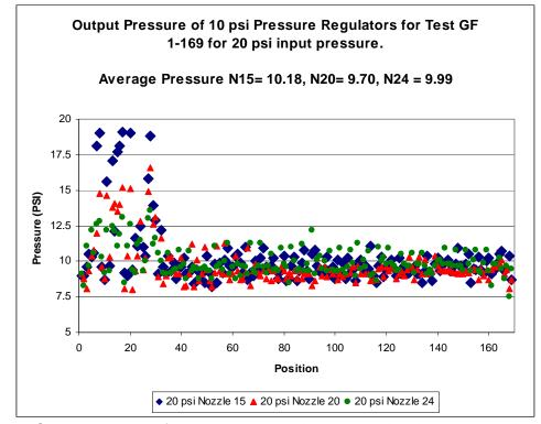
Figure 7. Output pressure of 169 pressure regulators tested at three nozzle sizes. Tests GF 1-169.
