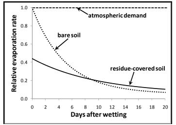
Figure 1. Evaporation rates, relative to atmospheric demand, from bare and residuecovered soil after a single wetting event (irrigation or rainfall) – conceptual diagram.
