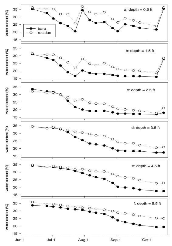
Figure 4. Mean volumetric soil water content in 2008 at six depths in bare-soil plots and in residue-covered plots.
