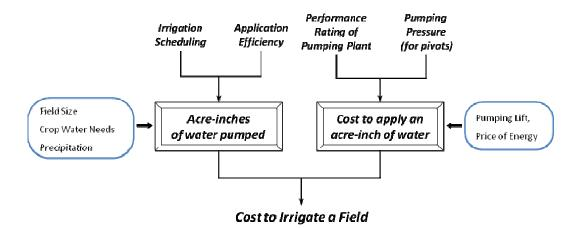
Figure 1. Diagram of factors affecting irrigation pumping costs
