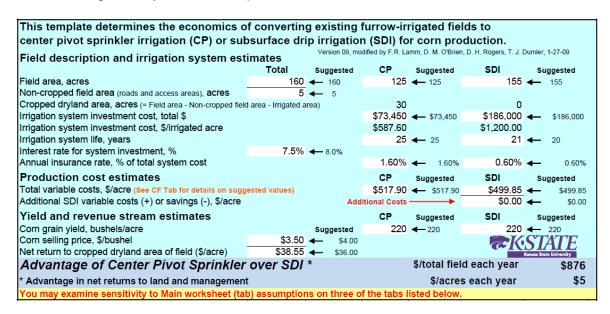
Figure 1. Main worksheet (tab) of the economic comparison spreadsheet template indicating the 18 required variables (white input cells) and their suggested values when further information is lacking or uncertain.
