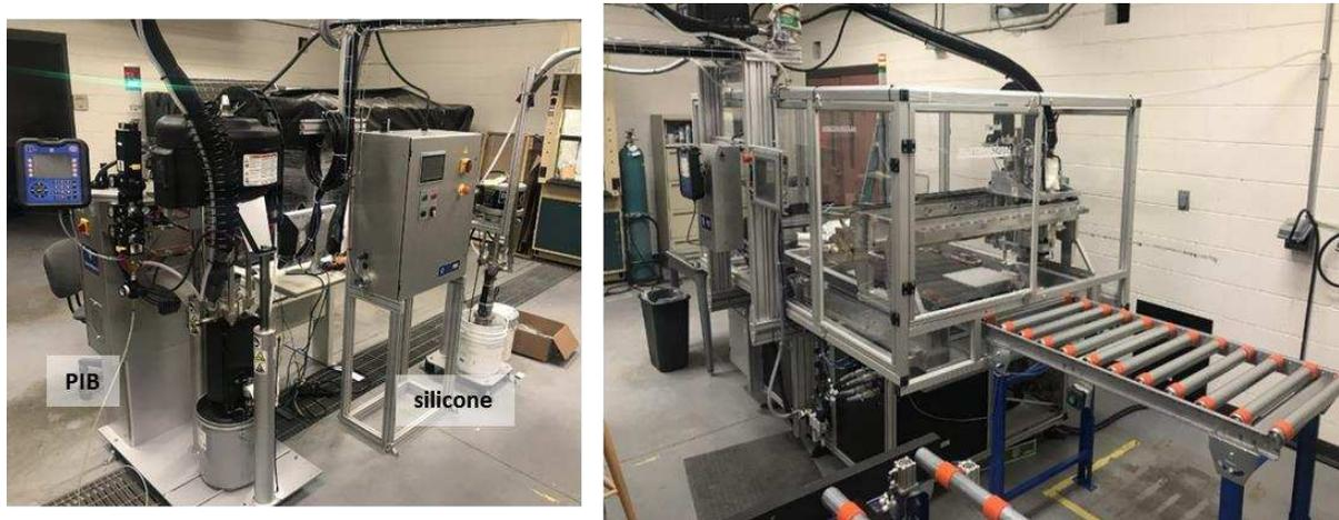
Figure 12: Graco supplied heated PIB pumping system (left) and polymer application tooling shown with 30cm x 30cm adapter plate installed (right).
