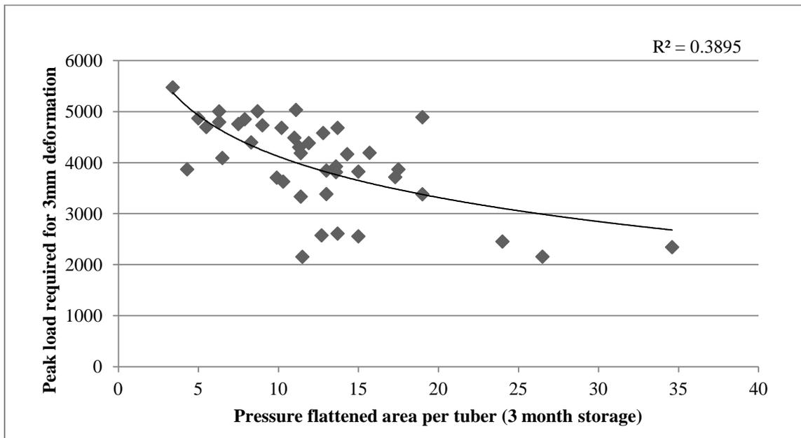
Figure 23. Correlation of at harvest peak load required for 3mm surface deformation with the pressure flattened area per tuber ( $\text{cm}^2$ ) after 3 months storage duration. The R-squared value for the correlation trend line is in the upper right corner of the figure.
