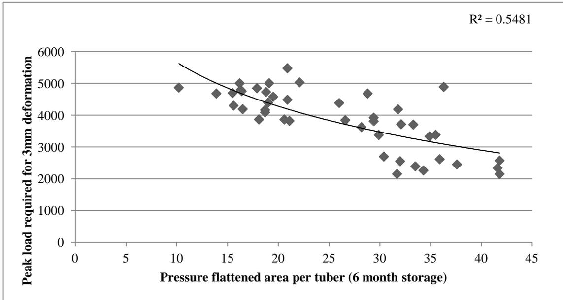
Figure 26. Correlation of at harvest peak load required for 3mm surface deformation with the pressure flattened area per tuber (cm<sup>2</sup>) after 6 months storage duration. The R-squared value for the correlation trend line is in the upper right corner of the figure.
