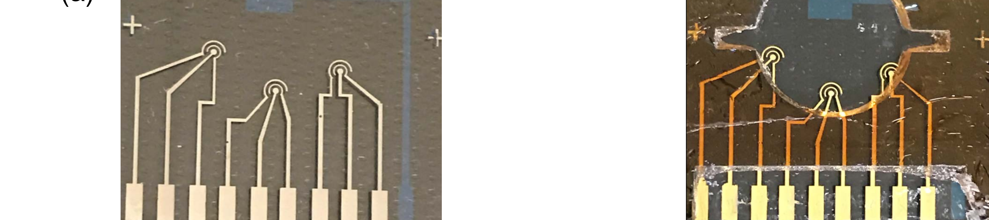
Figure 2: (a) complete electrodes design including: ITO pH electrode and integrated gold electrodes for Glucose, Lactate and DO sensing (b) microfluidic channel integrated with electrodes.
