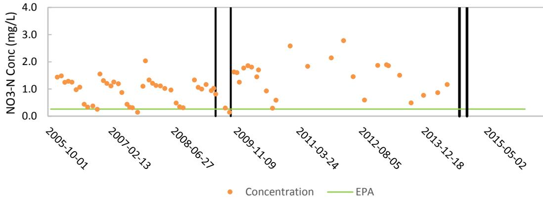
Figure B.4: Time series of NO<sub>3</sub>-N concentrations at NB-6. Black, vertical lines indicate the period of treatment.
