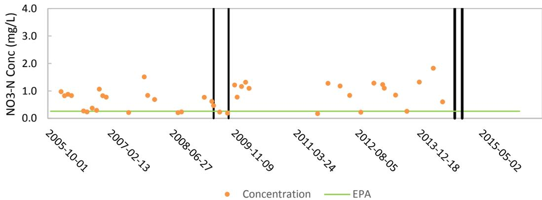
Figure B.6: Time series of NO<sub>3</sub>-N concentrations at NB-2. Black, vertical lines indicate the period of treatment.
