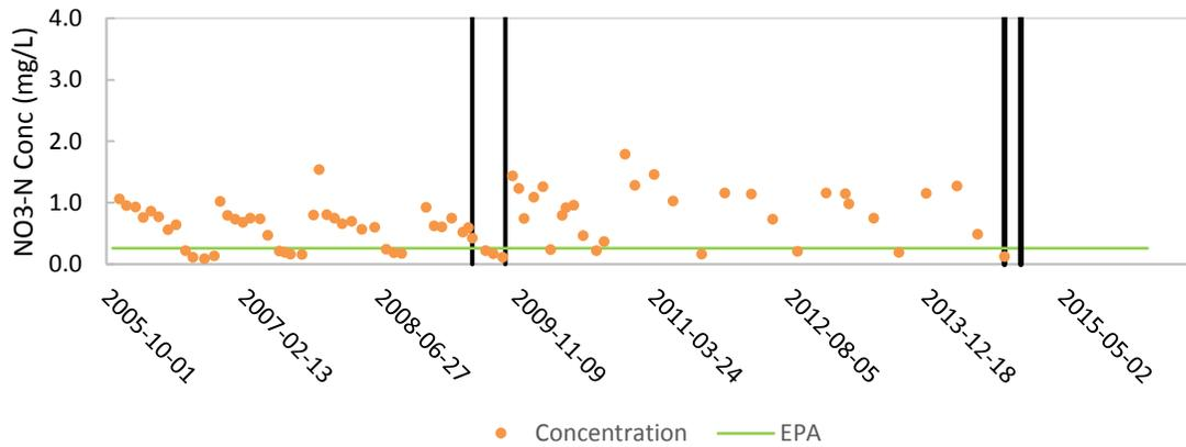
Figure B.7: Time series of  $\text{NO}_3\text{-N}$  concentrations at NB-1. Black, vertical lines indicate the period of treatment.
