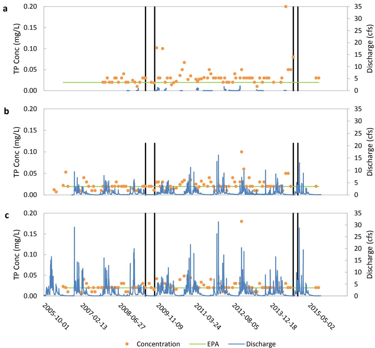
Figure 3.7: TP concentrations and discharge at (a) NBH, (b) NBU, and (c) NBL, and EPA recommended nutrient criteria. Black, vertical lines indicate periods of treatment.
