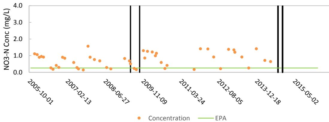
Figure B.5: Time series of NO<sub>3</sub>-N concentrations at NB-4. Black, vertical lines indicate the period of treatment.
