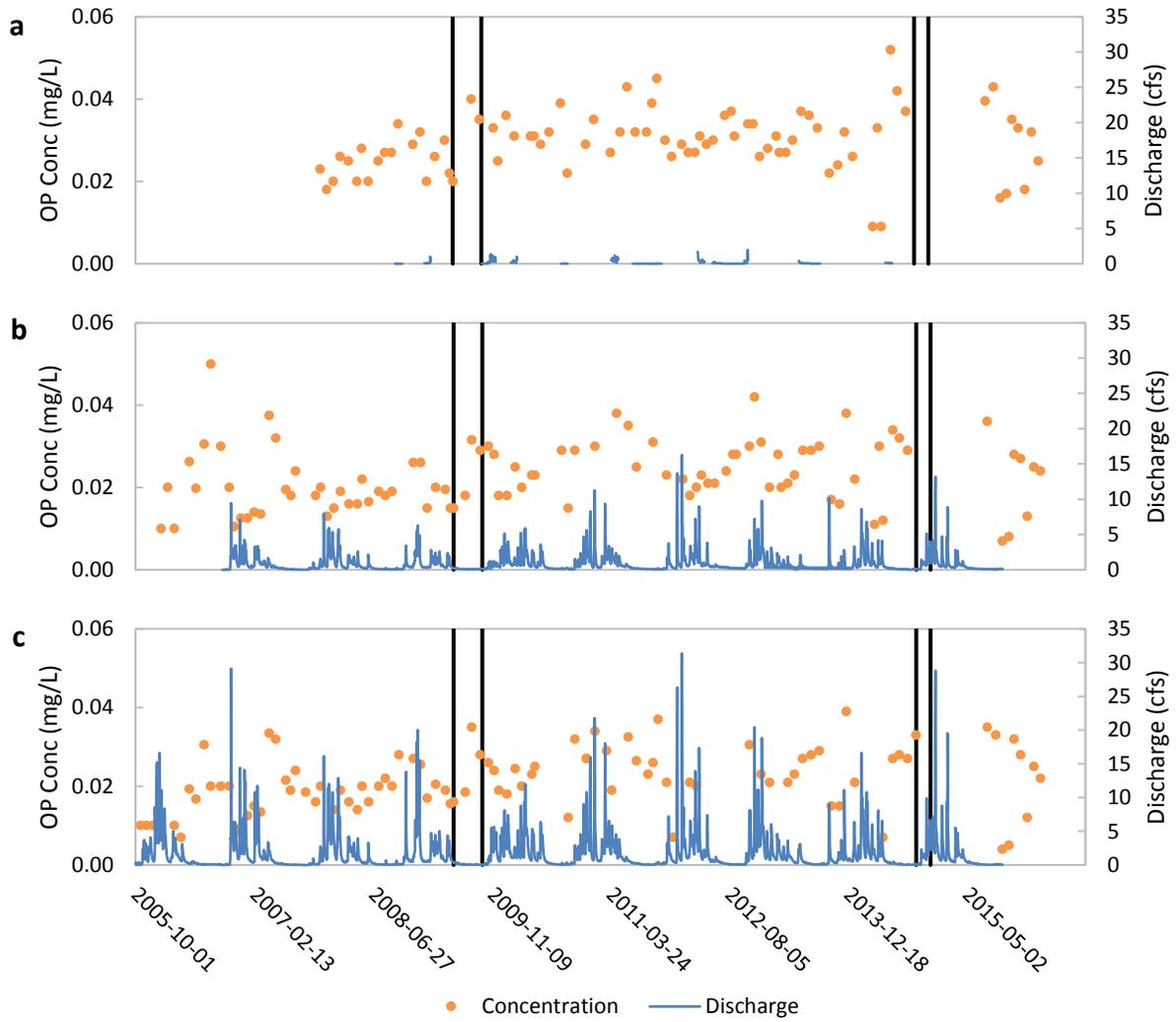
Figure 3.6: OP concentrations and discharge at (a) NBH, (b) NBU, and (c) NBL. Black, vertical lines indicate periods of treatment.
