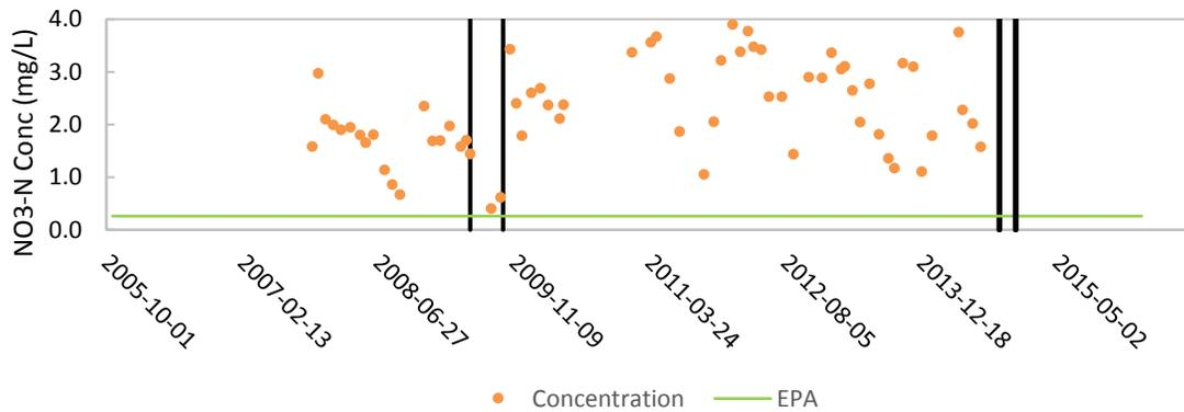
Figure B.1: Time series of NO<sub>3</sub>-N concentrations at UNB-A. Black, vertical lines indicate the period of treatment.
