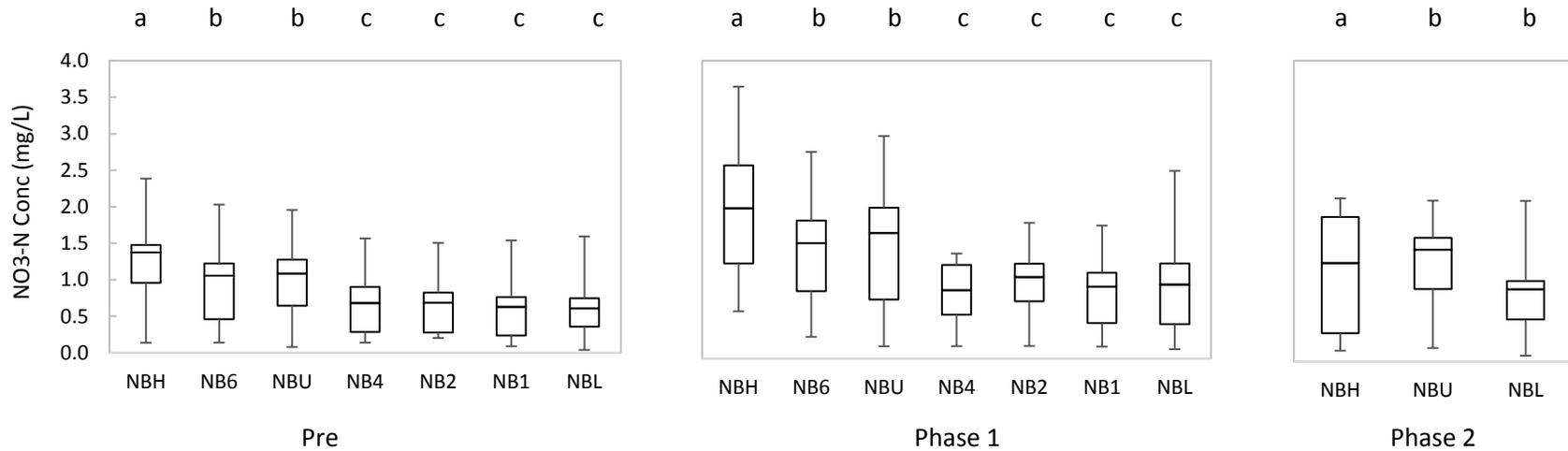
Figure 3.8: NO<sub>3</sub>-N concentrations, along the main stem of Needle Branch, for each phase of treatment. Distributions that do not share a letter are significantly different at  $\alpha = 0.05$ .
