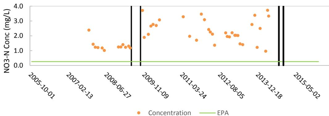
Figure B.3: Time series of NO<sub>3</sub>-N concentrations at UNB-C. Black, vertical lines indicate the period of treatment.
