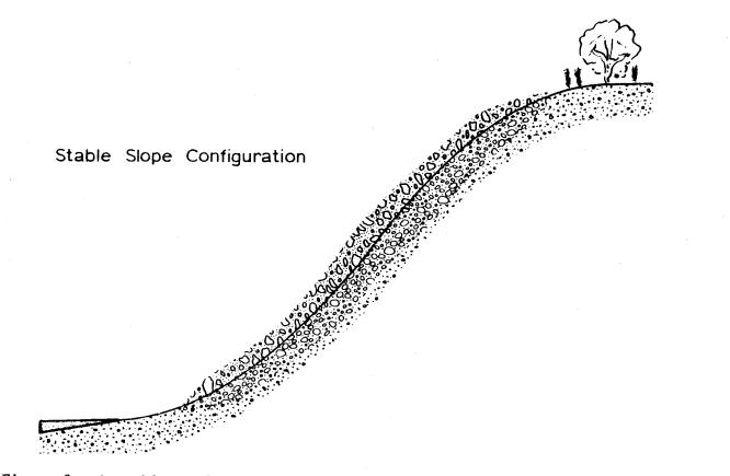
Figure 3. A stable configuration with reduced water velocities that has been roughened deep into the natural ground line at the time of construction offers more potential for revegetation than trying to plow the slope and round it later in the construction phase.
