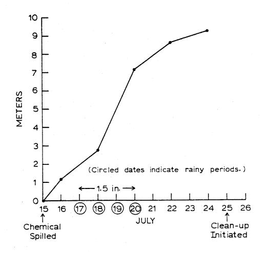
Figure 5. Movement of the copper ammonium chloride as measured by the effects upon *Thalictrum sparsiflorium* (1 m = 3.28 ft).
