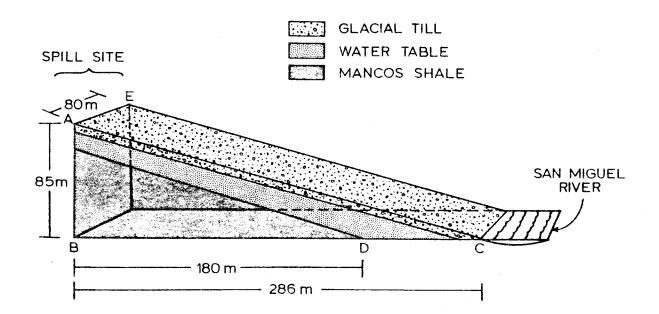
Figure 1. The geology and slope profile of the Lawson Hill site (1 m = 3.28 ft).
