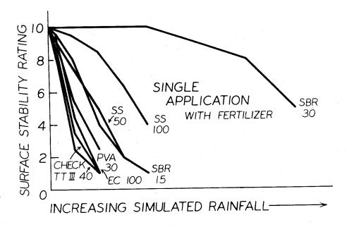
Same treatments as figure 1 except slurry contained fertilizer Figure 2. (16-20-0 at 500 lb/acre).
