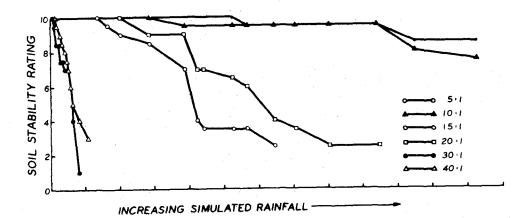
Figure 6. Effect of simulated rainfall on the surface stability of sand treated with 1,000 lb/acre PVA solids at various dilution rates.
