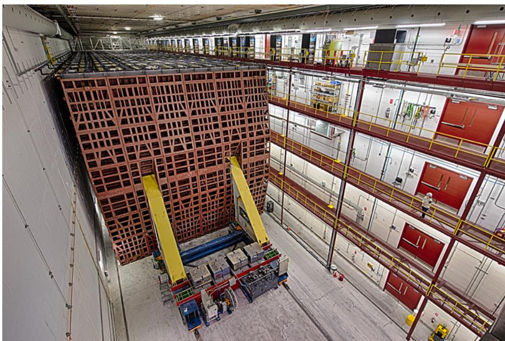
FIGURE 3.5. The fully constructed Far Detector in the Ash River facility. Note the person on the third floor catwalk for a sense of scale.[19]
