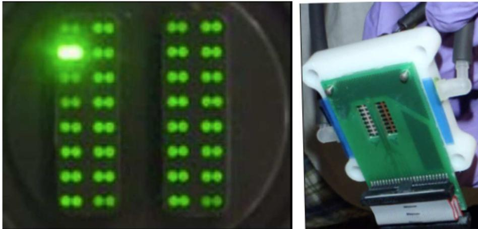
FIGURE 3.9. Photographs of the fiber ends in the connector and the pixel array of the MPPC. The MPPC fits into the connector lining up each pair of fiber ends from a cell to one of the 32 pixels.[19]
