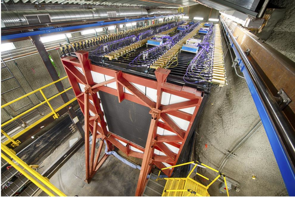
FIGURE 3.6. A picture of the front face of the Near Detector inside the Near Detector Hall at Fermilab. The beam direction is into the visible detector face.[19]
