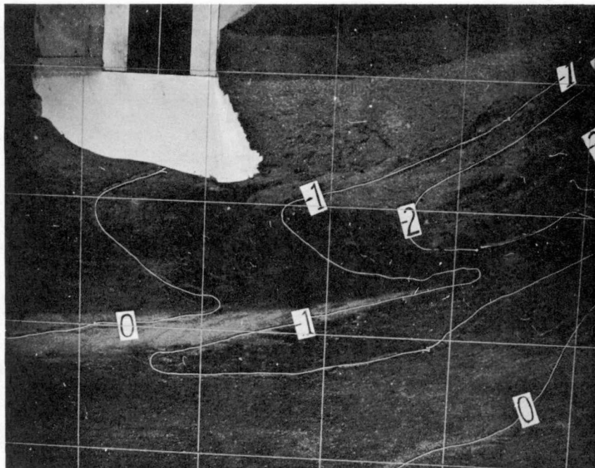
Figure 8 Note the 0 contour is midway along the embankment. There is deposition downstream from this point. \lambda = 3 L_s = 3.41 ft Q_t = 4.80 cfs Q_s = 0 L_o = 8.0 ft.
