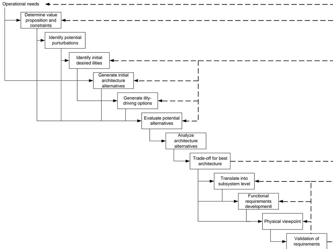
Figure 15. Extended SAI method flow diagram
