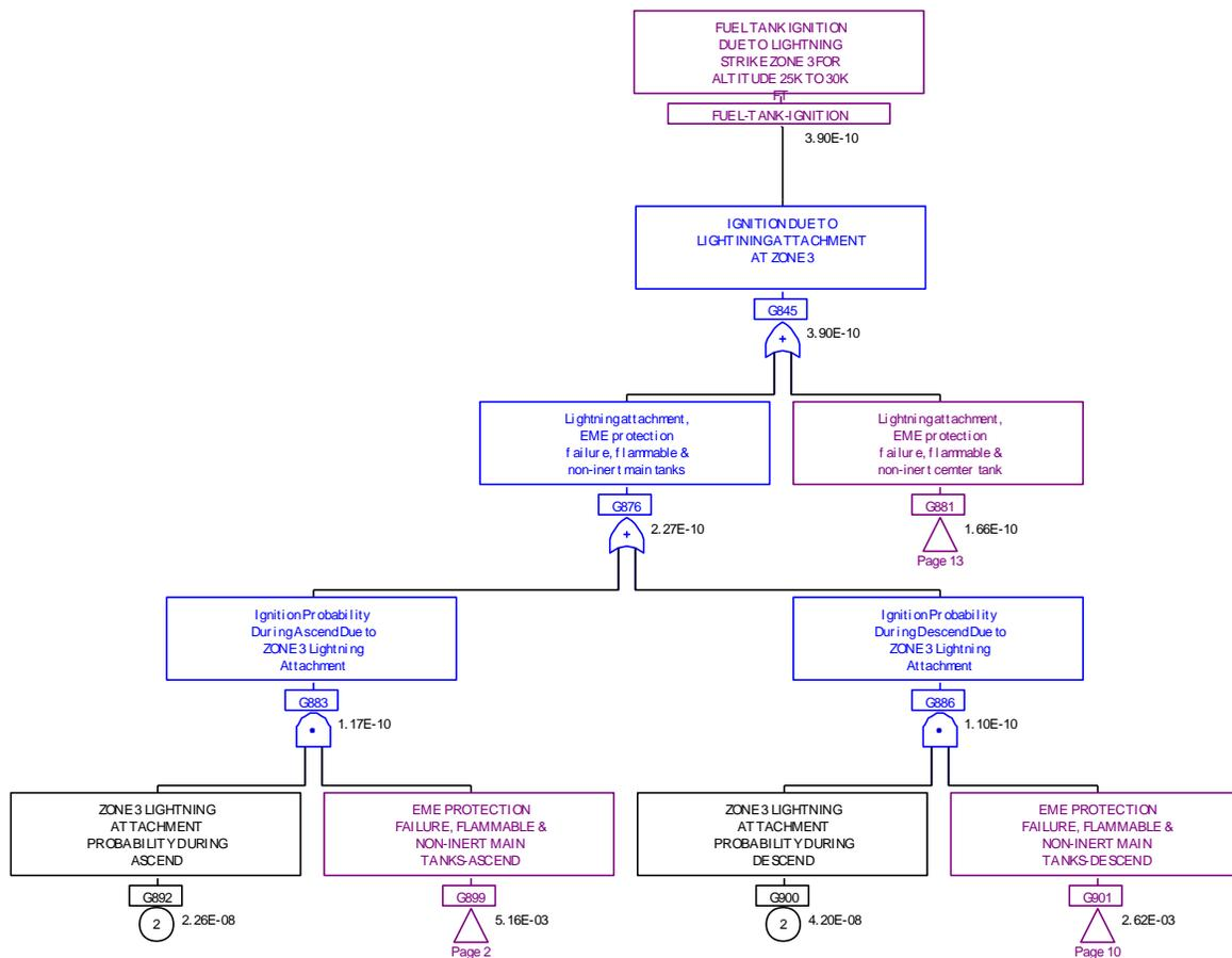
Figure 69. Fault tree for the altitude range from 25,000 to 30,000 ft
