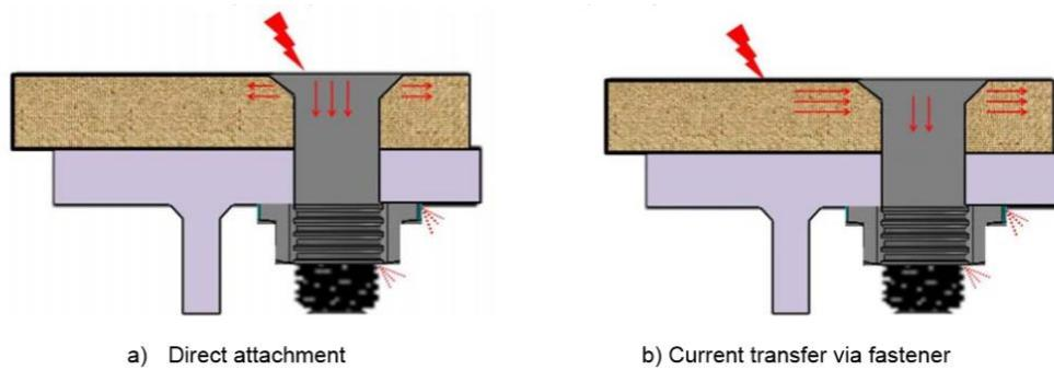
Figure 62. lightning attachment and ignition mechanism
