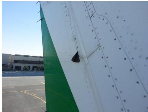
Figure 51. Conductive strip in rudder may get lifted and damaged due to water ingress
