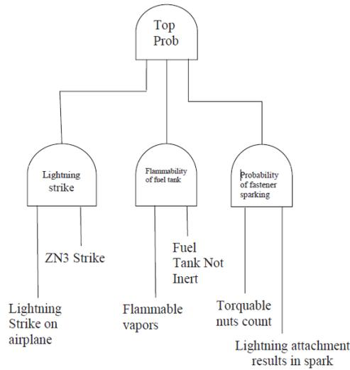
Figure 54. Top probability of lightning strike fault tree analysis
