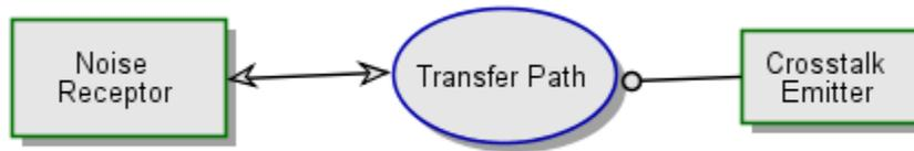
Figure 29. EMI energy coupling diagram with OPM modeling. Note the crosstalk emitter is part of the system with solid lines
