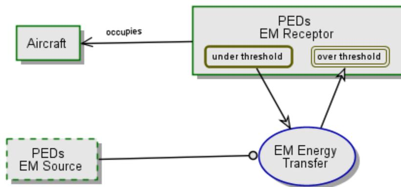
Figure 28. Portable electronic device energy coupling diagram with OPM modeling. PEDs EM sources are part of the environment with dotted lines
