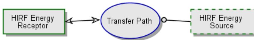
Figure 31. HIRF energy coupling diagram with OPM modeling. HIRF energy source is part of the environment with dotted lines
