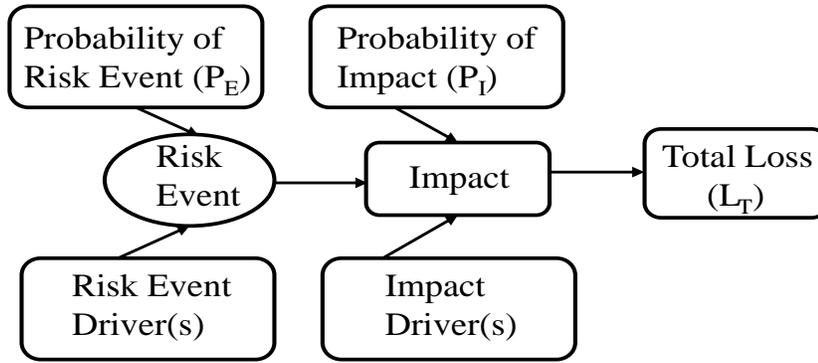
Figure 36. Standard risk model to be used for electromagnetic effects analysis
