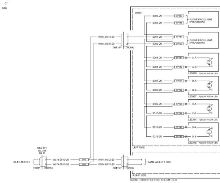
Figure 17. Wiring diagram of emergency floor proximity light system
