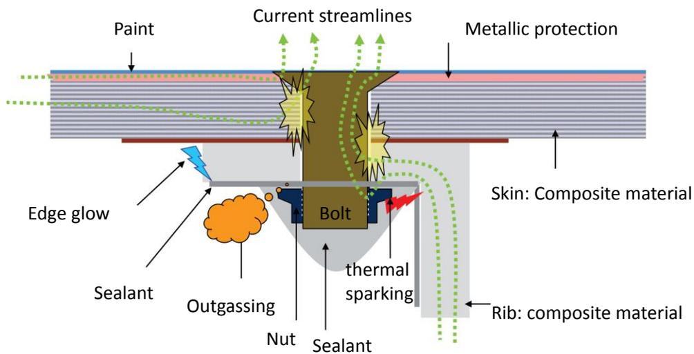
Figure 63. Sparking mechanism due to lightning current
