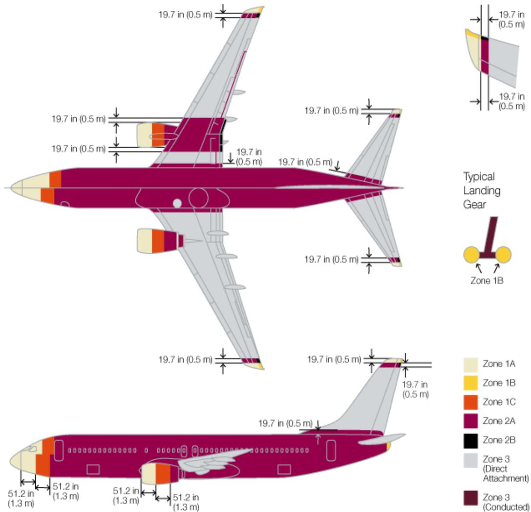
Figure 47. Lightning zone of aircraft
