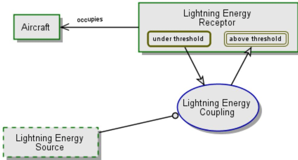
Figure 46. Lightning energy coupling modeling with OPM
