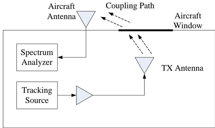
Figure 40. PEDs front door coupling
