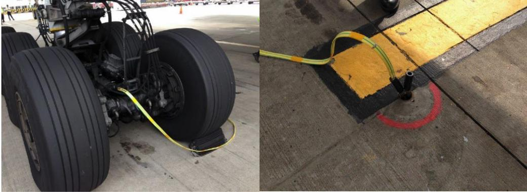
Figure 75. Connection of the grounding cable from the landing gear to ground post in airport
