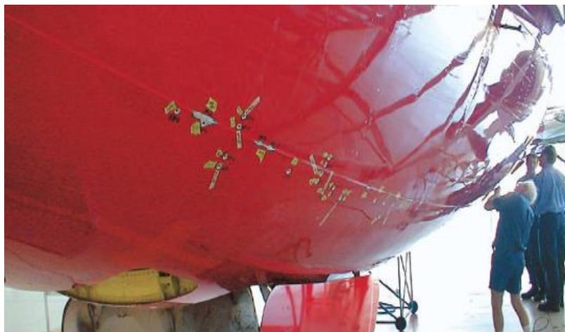
Figure 38. Direct lightning effect due to swept strokes on aircraft
