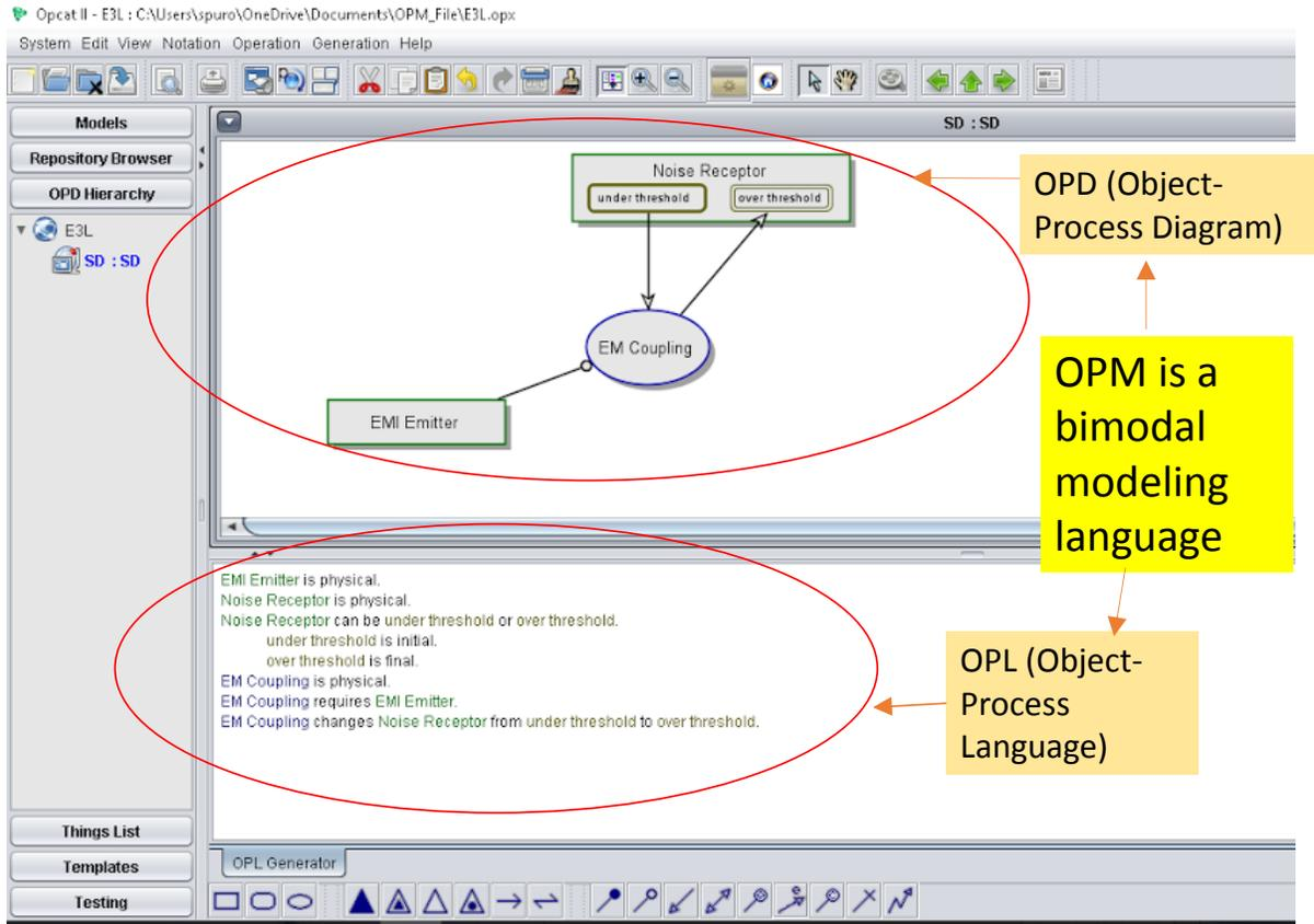
Figure 9. OPCAT suite for EMI energy coupling model
