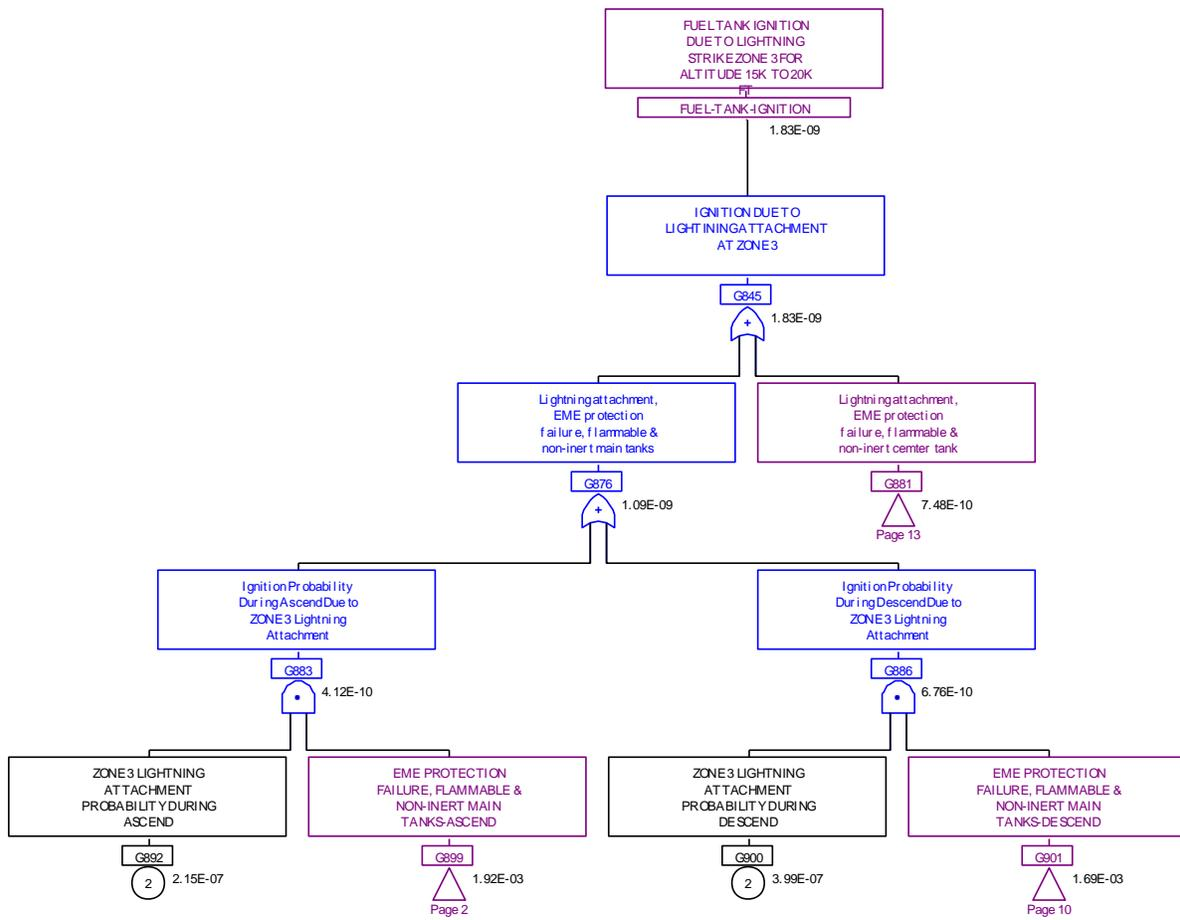
Figure 67. Fault tree for the altitude range from 15,000 to 20,000 ft
