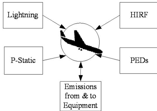
Figure 27. Aircraft electromagnetic effect context diagram
