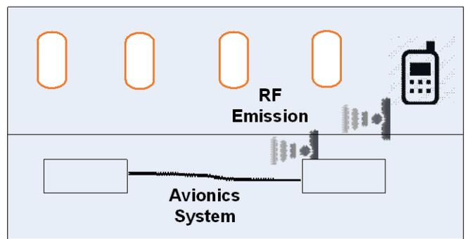
Figure 41. PEDs back door coupling
