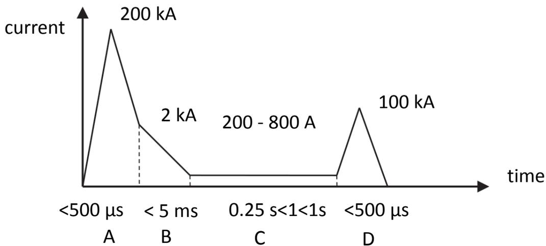
Figure 56. Lightning current waveform as a function of time
