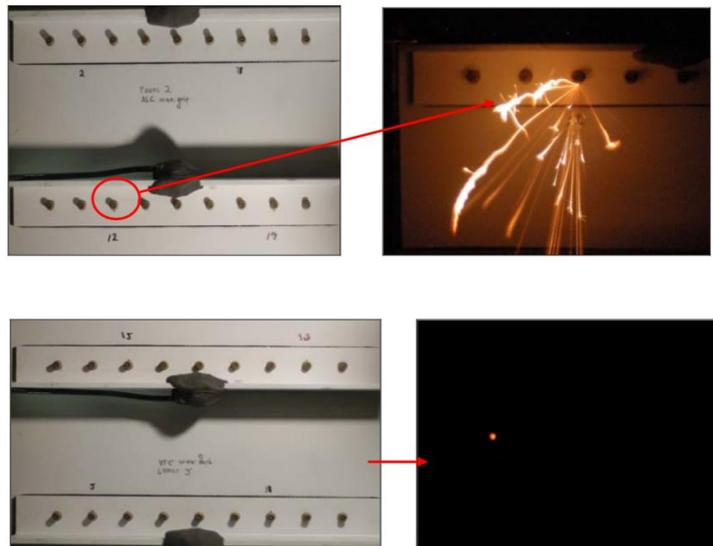
Figure 61. Test pass or fail criteria of light on film (LOF)
