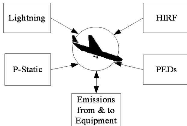
Figure 13. Aircraft electromagnetic context diagram
