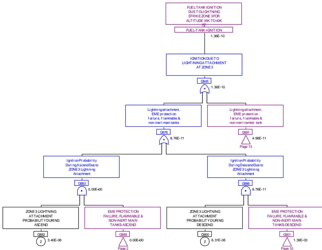
Figure 71. Fault tree for the altitude range from 35,000 to 40,000 ft
