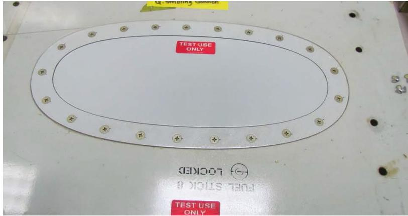
Figure 57. Typical fuel tank door configuration
