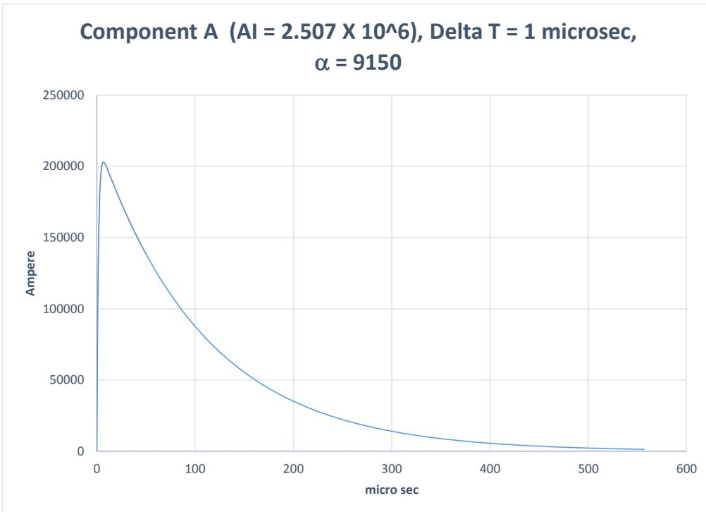
Figure 55. Design of lightning waveform for component A
