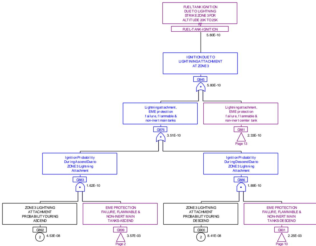
Figure 68. Fault tree for the altitude range from 20,000 to 25,000 ft
