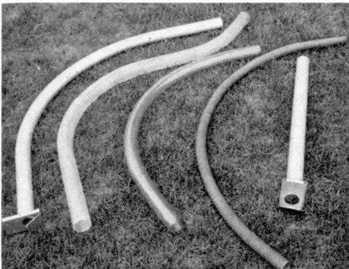
Some of the common shapes and materials used in siphon tubes and spiles found on the market. From left to right: a single-bend aluminum siphon tube with adjustable gate, a double-bend plastic tube, a single-bend plastic tube, a flexible coiled-wire reinforced rubber tube, and an aluminum spile with adjustable gate.
