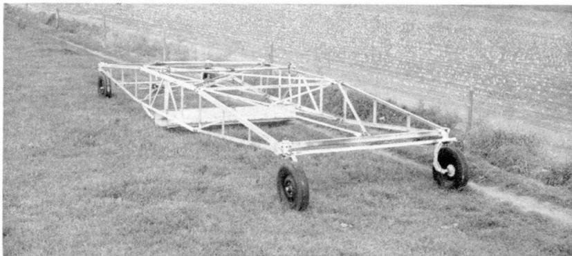
The land plane is the sandpapering equipment used after the deep cuts and fills have been made. It is useful each spring to smooth out irregularities caused by tillage operations.
