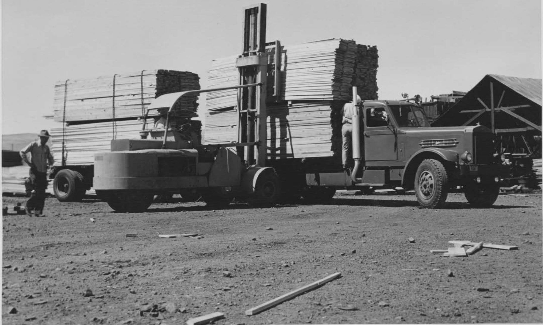
Plate XIX: Loading lumber truck with lift truck.
