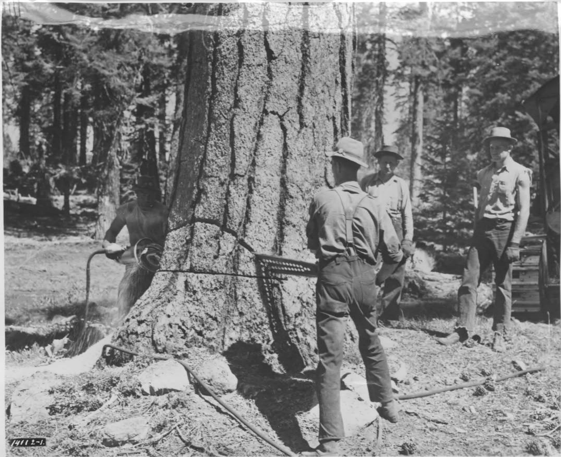
Plate VI: Undercutting with Atkins electric power saw and Caterpillar tractor.
