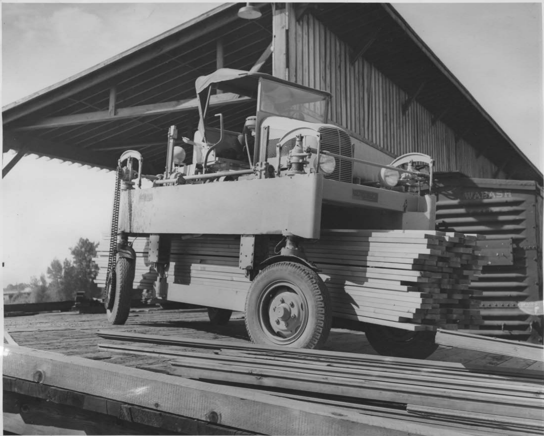
Plate XVI: Moving lumber with straddle carrier.
