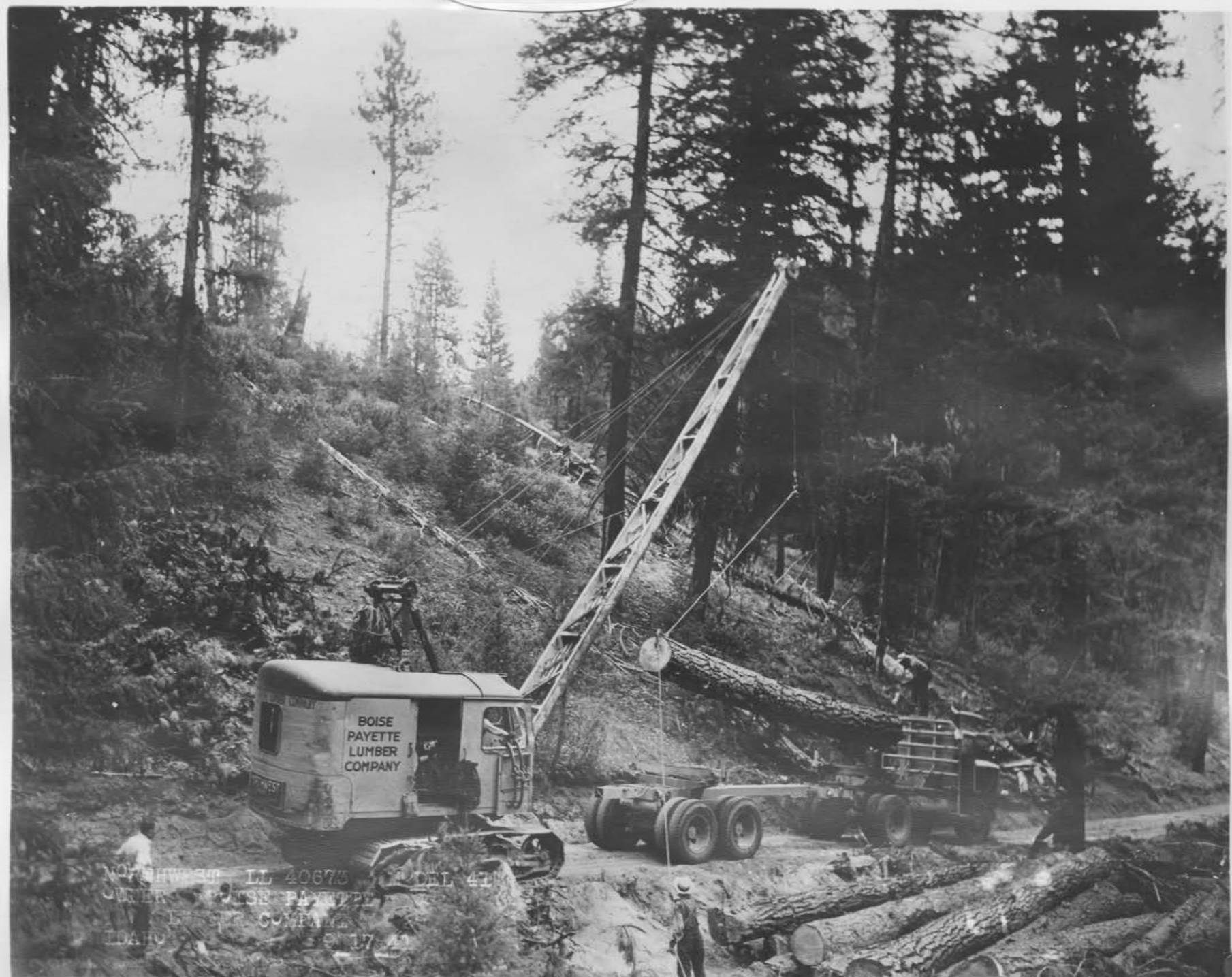
Plate XII: Loading with Northwest crawler shovel equipped with crotch line and bell hooks.
