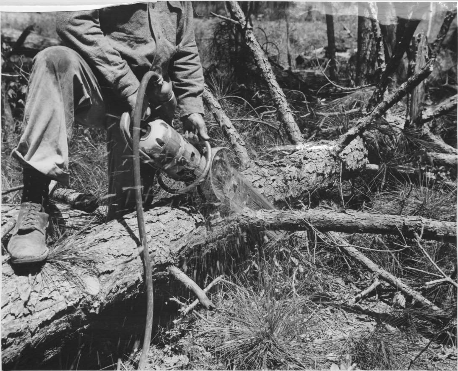
Plate IX: Limbing with Atkins electric power saw.
