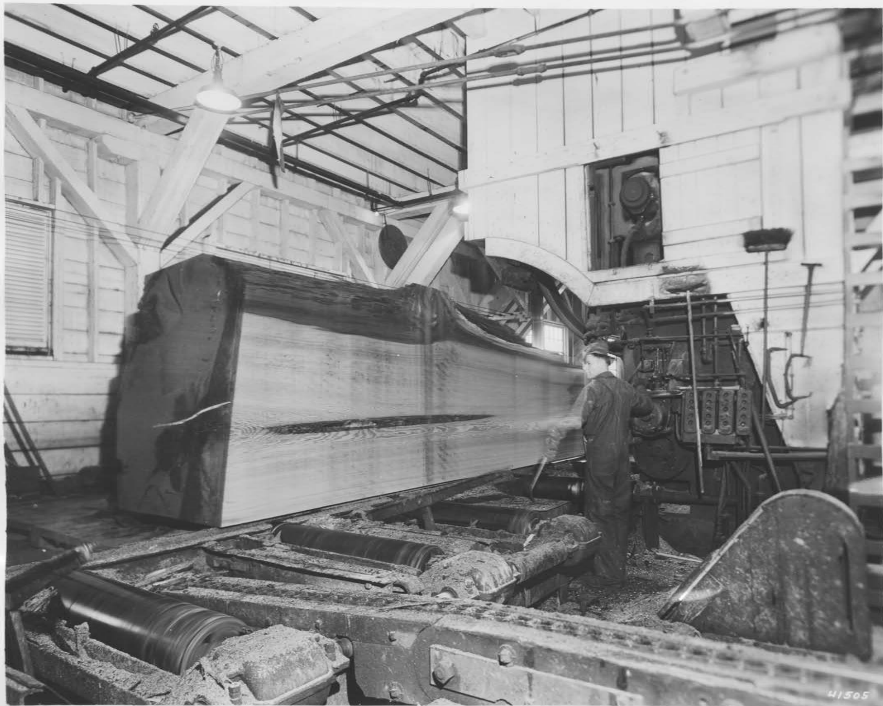
Plate XIV: Sawing lumber with hand head saw.
