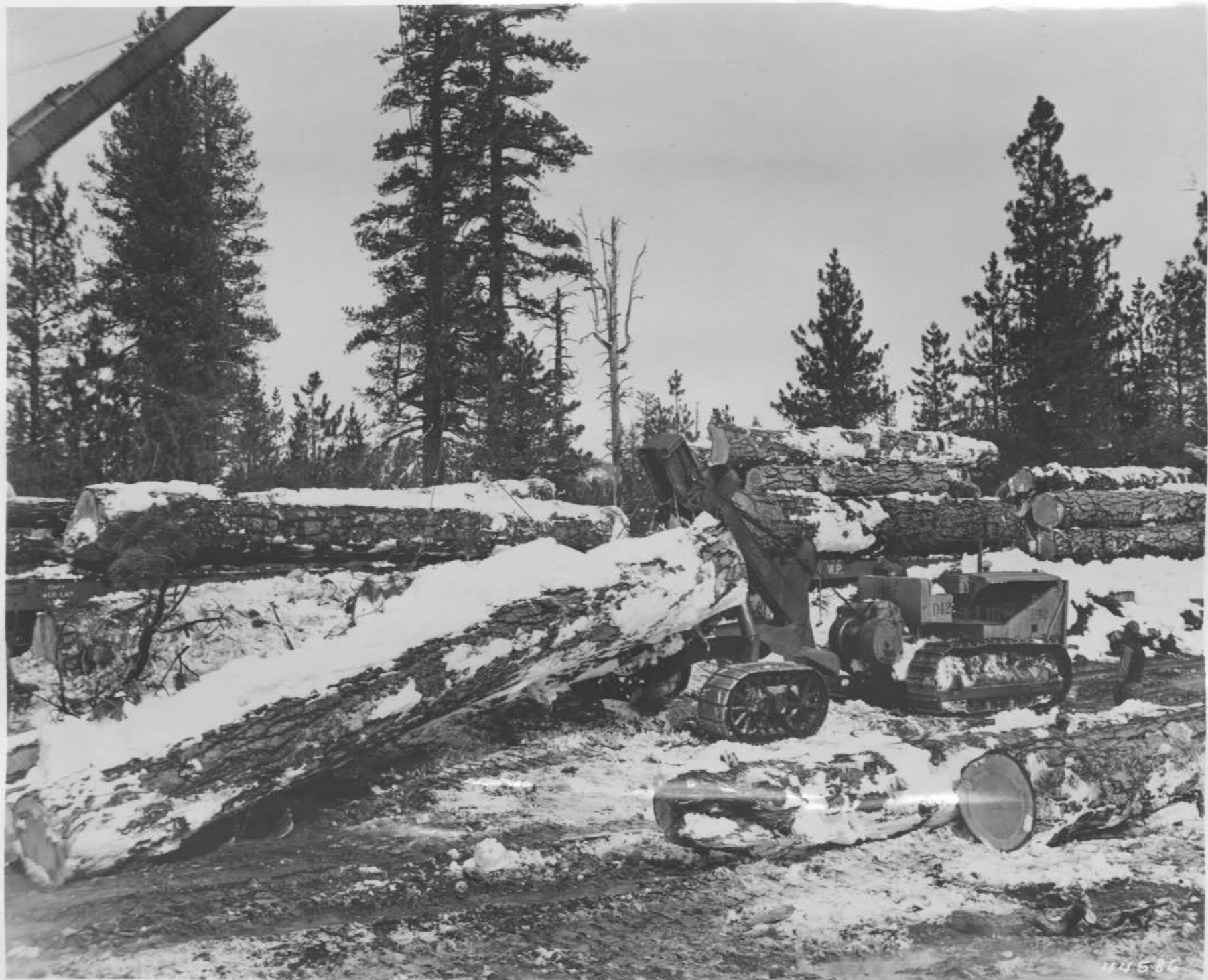
Plate XI: Arch skidding with Caterpillar tractor and Hyster arch.
