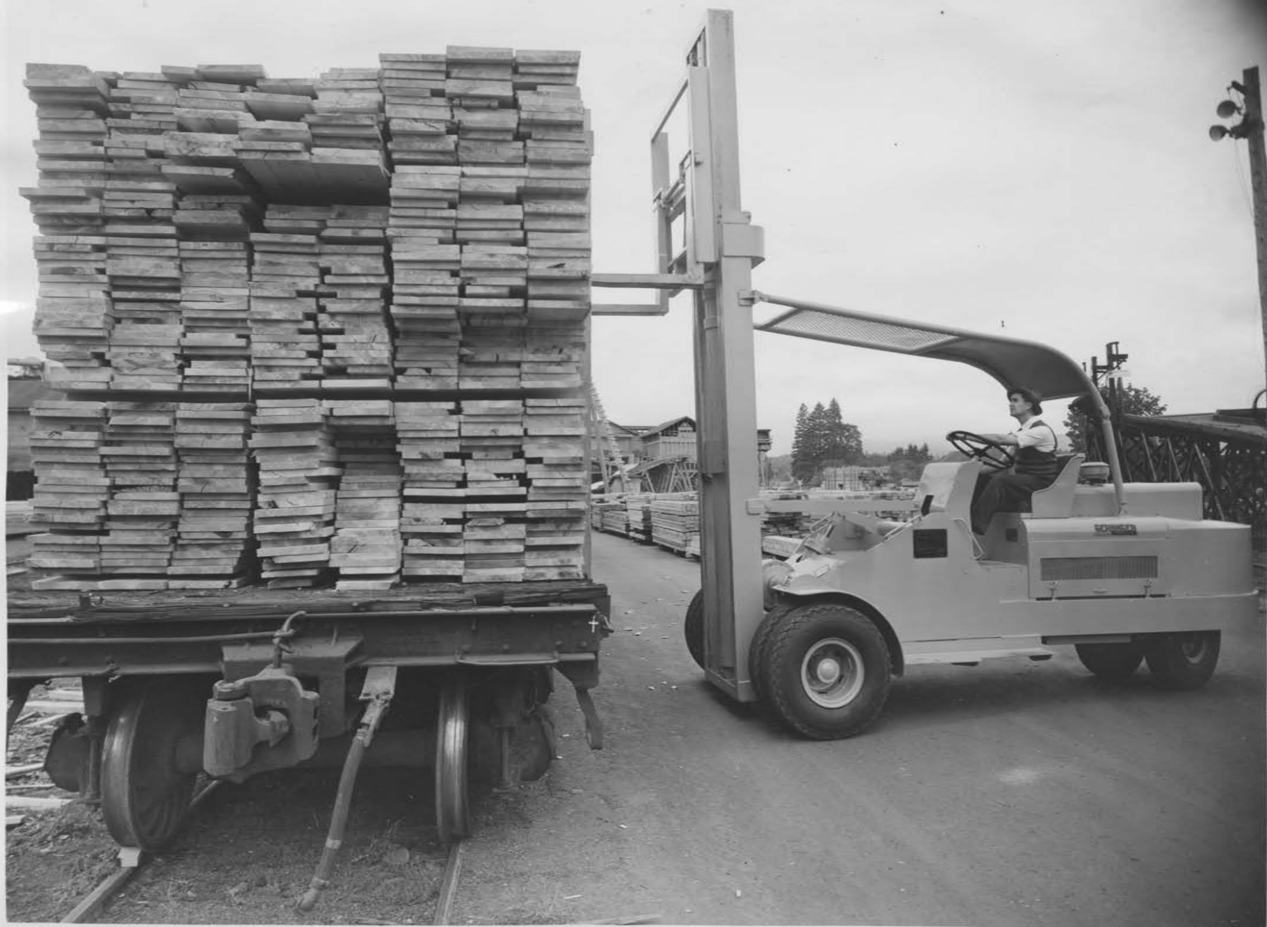
Plate XVIII: Loading flat car with lift truck.
