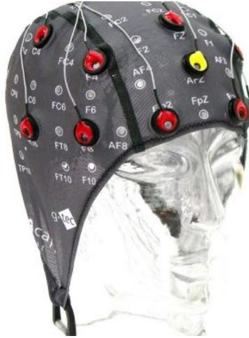
FIGURE 3.1. g.Tec g.GAMMMAsys EEG recording cap with electrodes
