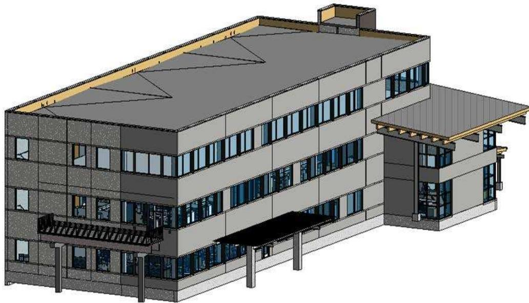
Figure 12: BIM model of precast using sandwich panels
