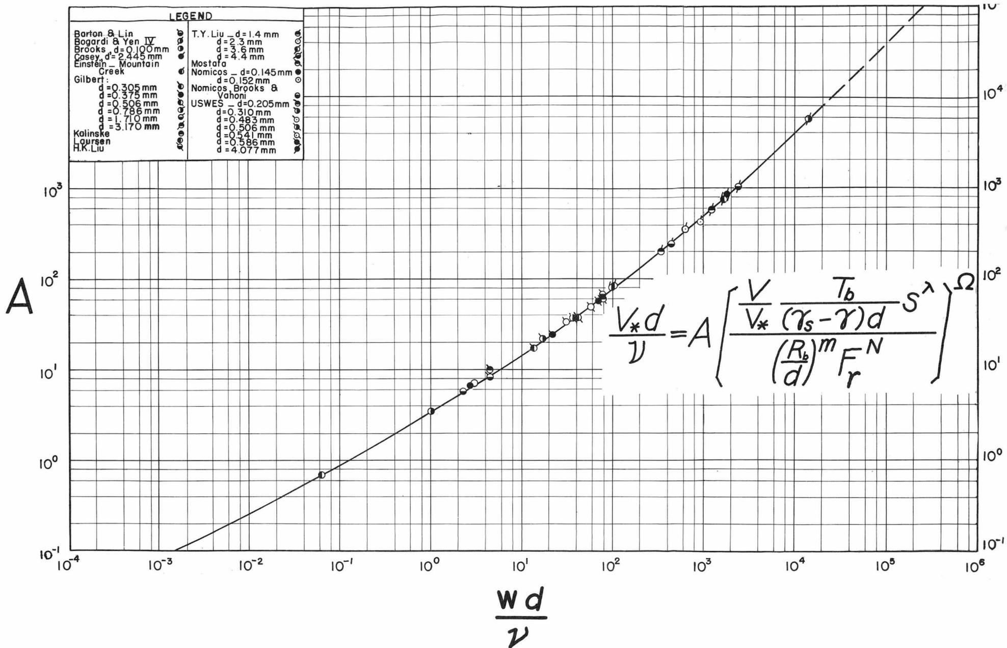
FIG. 8 VARIATION OF A WITH  $\frac{wd}{\nu}$  FOR ALLUVIAL DUNE BED
