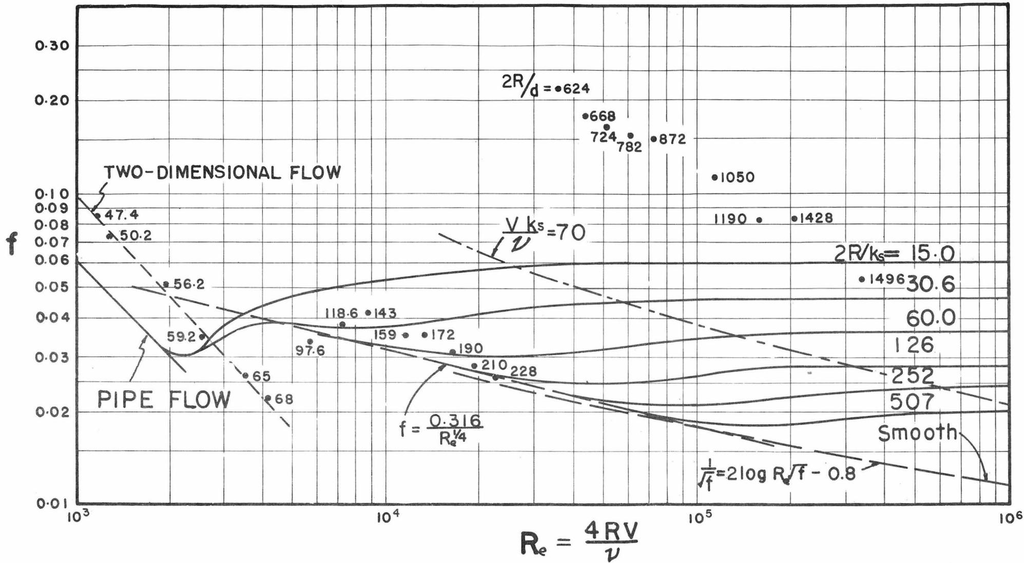
FIG. 2 VARIATION OF  $f$  WITH  $\frac{4RV}{\nu}$  FOR ALLUVIAL BED
