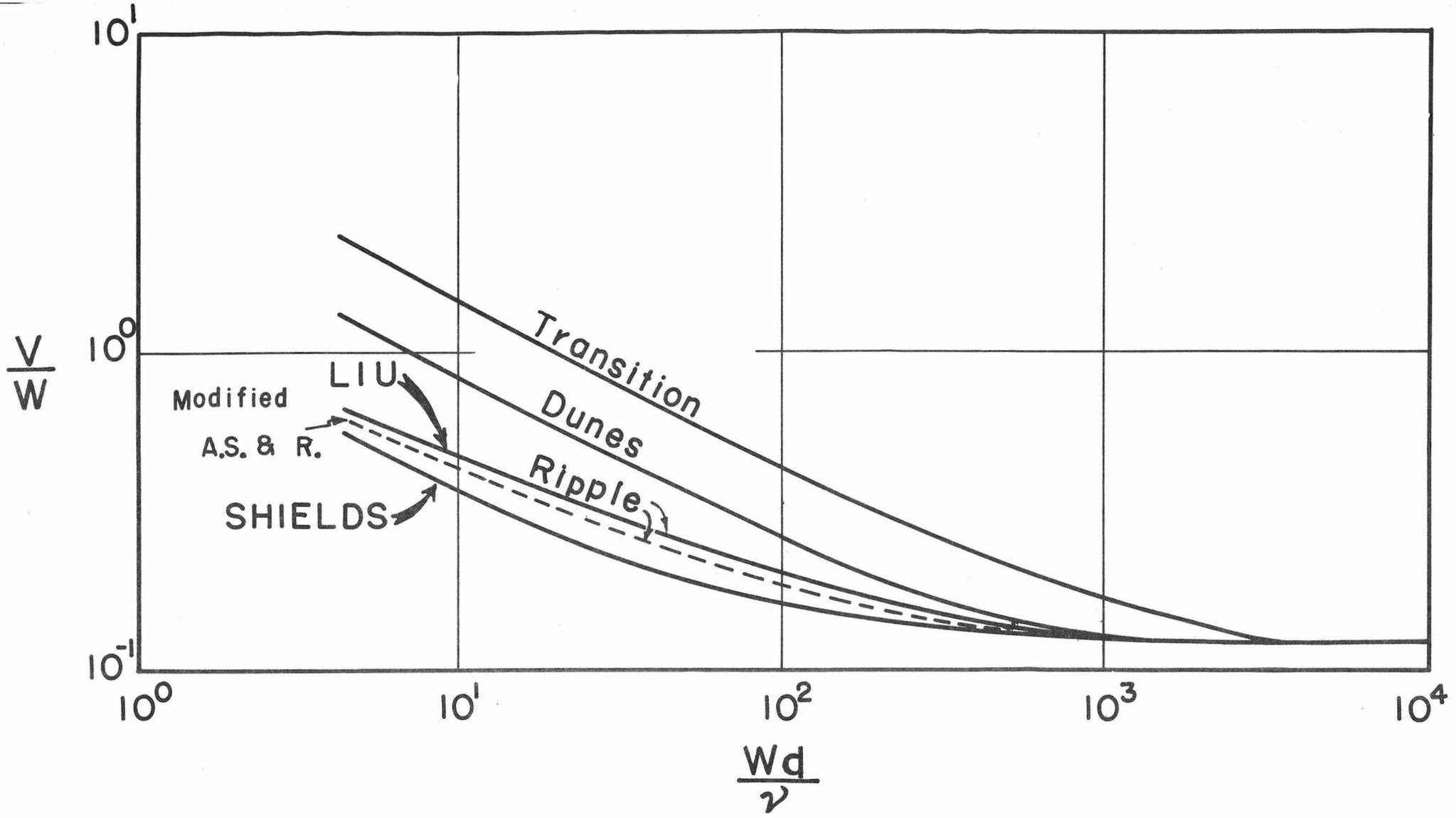
FIG. 1 CLASSIFICATION OF THE CONFIGURATION OF ALLUVIAL BED
