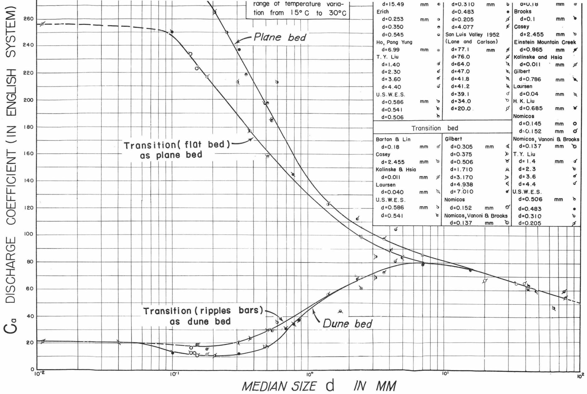
FIG. 11 VARIATION OF  $C_a$  (IN ENGLISH SYSTEM) WITH  $d$  FOR FLOW OVER ALLUVIAL BED
