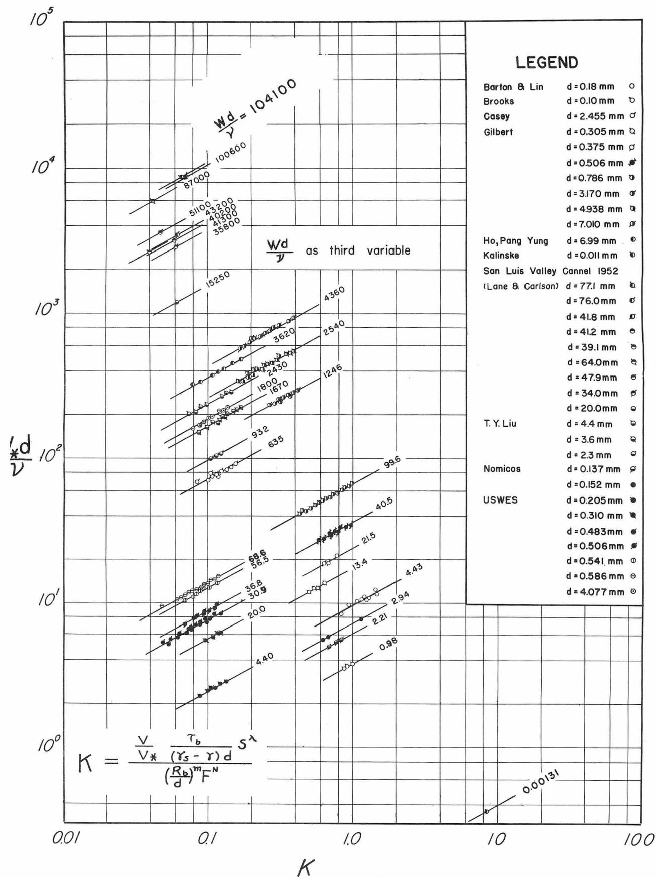
FIG. 4 CHARACTERISTICS OF FLOW OVER ALLUVIAL PLANE BED
