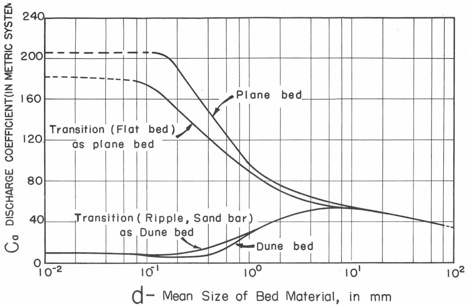
FIG. 12 VARIATION OF  $C_d$  (IN METRIC SYSTEM) WITH  $d$  FOR FLOW OVER ALLUVIAL BED
