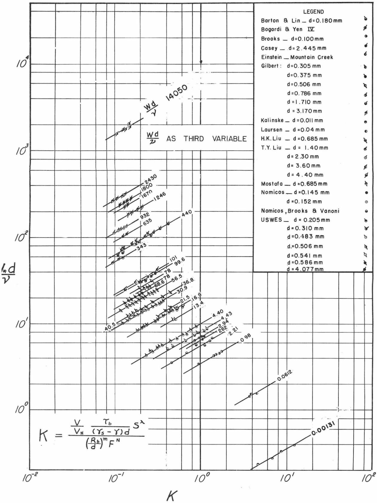
FIG. 7 CHARACTERISTICS OF FLOW OVER ALLUVIAL DUNE BED
