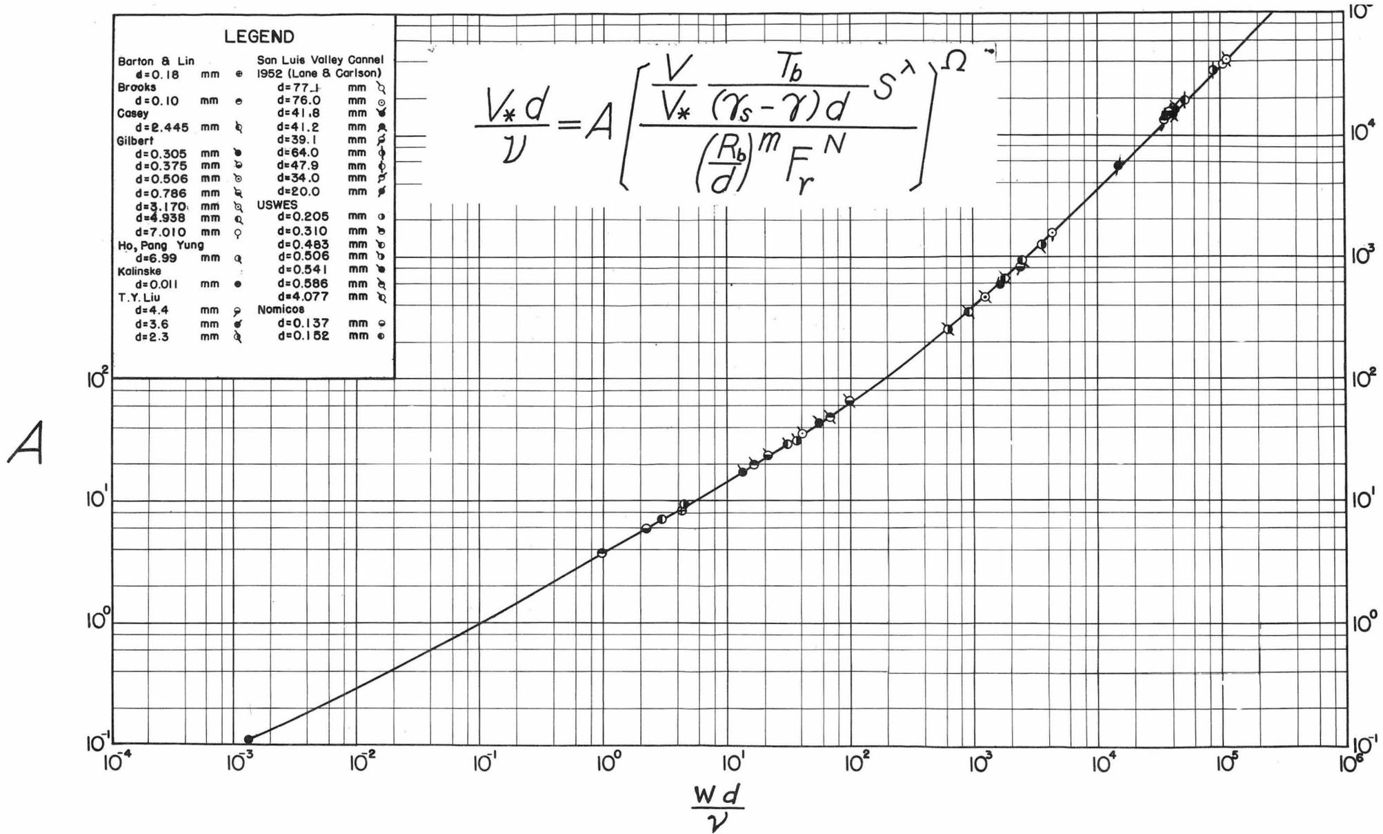
FIG. 5 VARIATION OF A WITH  $\frac{Wd}{\nu}$  FOR ALLUVIAL PLANE BED
