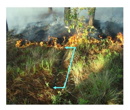
Figure 3.5. A direct method of measuring the rate of spread and of estimating flame height, when it is possible to work safely next to the flames. In this example, we utilized a meter-long metal tube, visible in the photograph to the left of the blue line, plus an ordinary stop watch. An estimate of the average flame length in this photo would be 10 centimeters.
