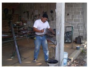
Blacksmith cutting meter-long pipes for measuring fire rate of spread.
