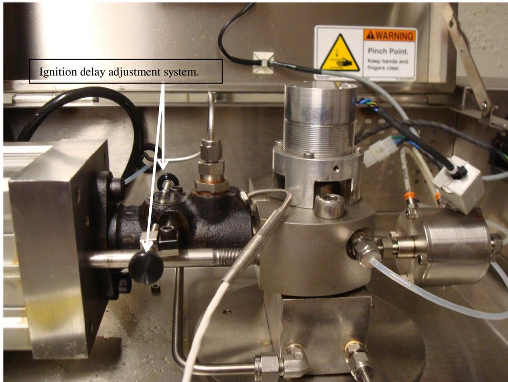
**Figure 2.7. FIT fuel injection system.**
