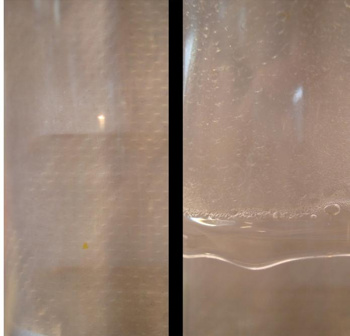
**Figure 2.5. Measuring vessel before (left) and after (right) Rancimat test.**
