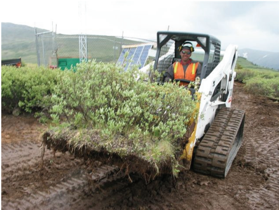
Figure 1. Conventional Track Mounted Skid Steer Loader with 4 Feet Square Piece of Tundra Sod
