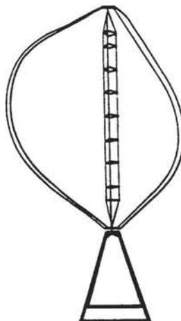
A vane-axial type wind machine.
