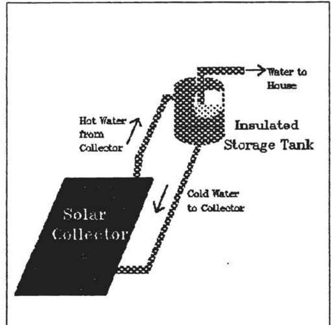
In a climate as cold as Colorado's, a passive solar water heater is best suited to preheat water. As shown in the figure on the left, the water is
