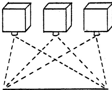
Full color images can be produced when each of the separate images is processed and superimposed in its respective color on a single frame. Technical malfunctions forced the RBV systems to be shut down shortly after launch.
