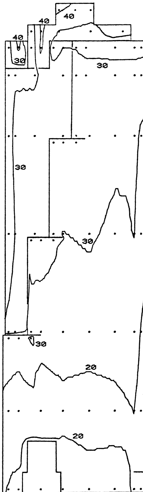
Figure 10h. Peak Pressure Contours on the Building for Cladding Loads
