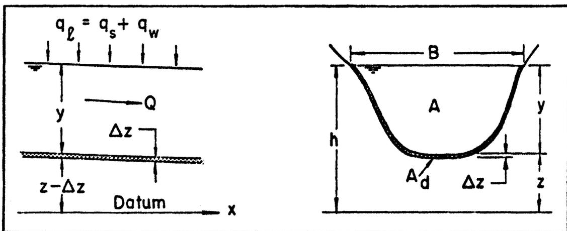
Figure 2. Definition sketch of an alluvial channel
