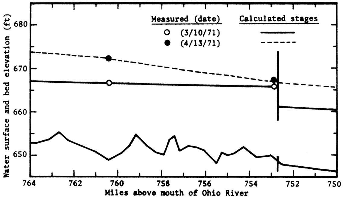
Figure 11. Mathematical model reproduction of 1971 water surface hydrograph and profile in Pool 4 of the Upper Mississippi River
