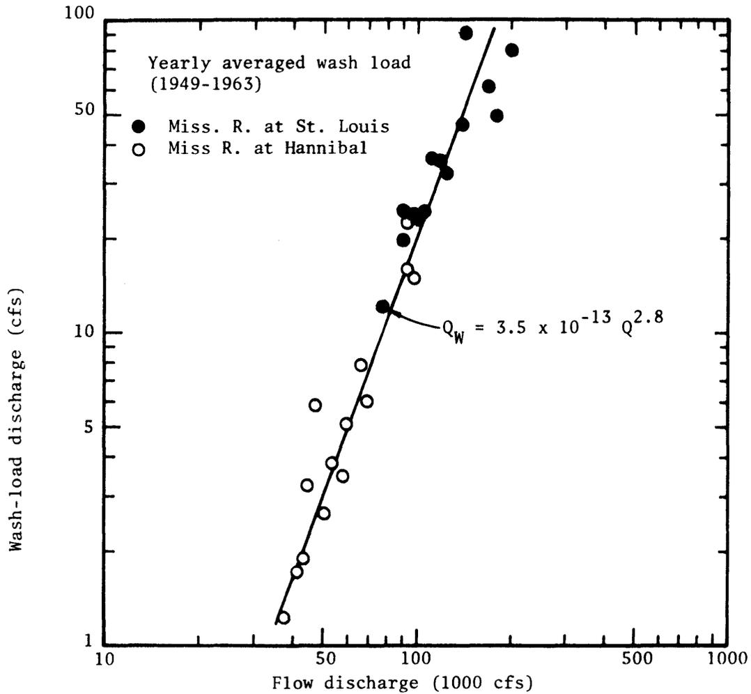
Figure 8. Relation between wash-load discharge and flow discharge (data obtained from "Summary and Analysis of Sediment Records in Relation to St. Louis Harbor Sediment Problem," by P. R. Jordan, U.S.G.S., Open-File Report, 1968)
