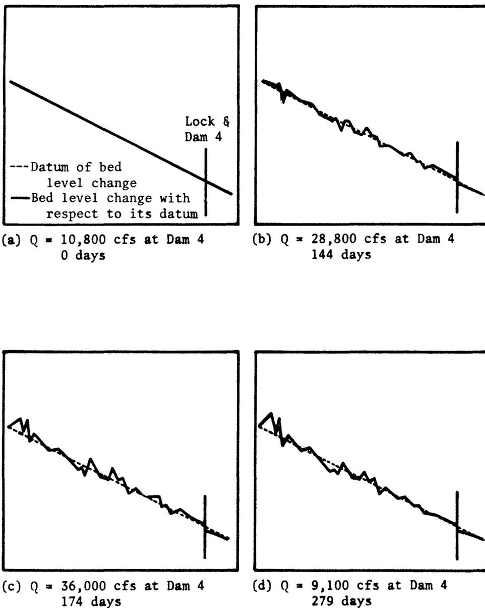
Figure 19. Bed elevation change in the Pool 4 reach of the Upper Mississippi River during a flood routing
