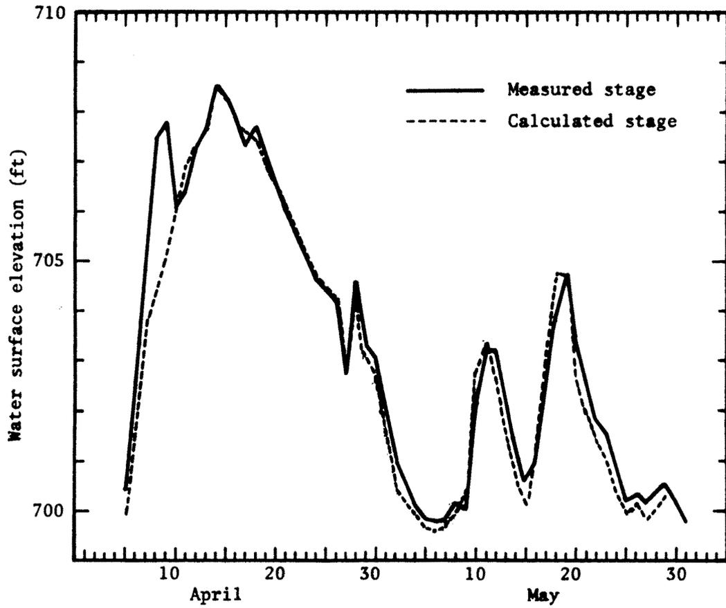
Figure 10. Mathematical model reproduction of 1965 stage hydrograph in the Chippewa River at Durand
