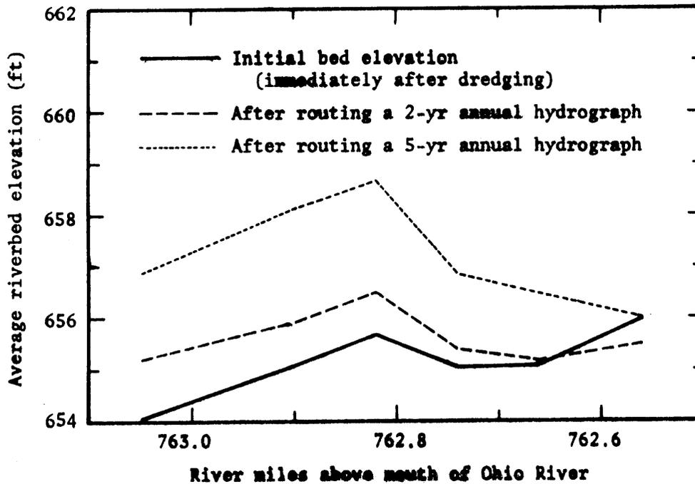
Figure 21. Riverbed elevation changes near Reads Landing after routing an annual hydrograph (with dredging)
