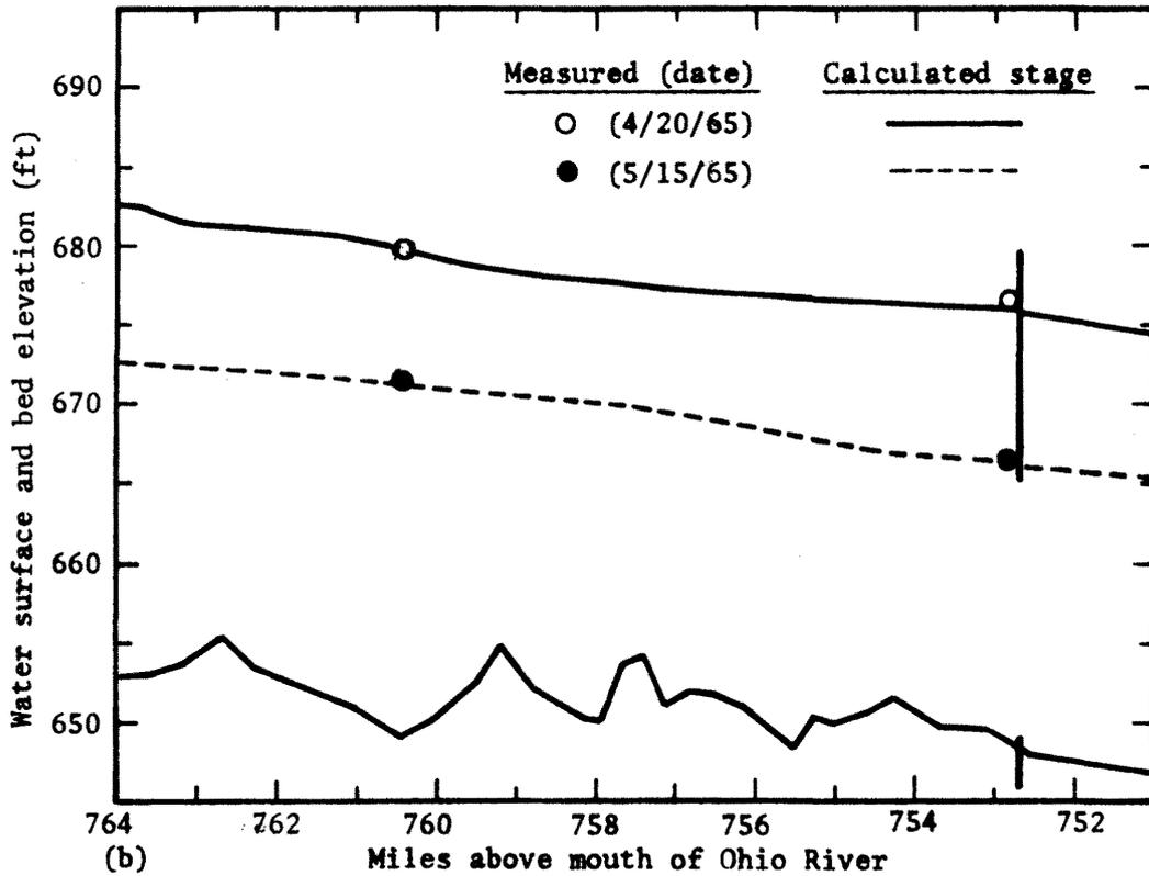
Figure 9. Mathematical model reproduction of 1965 water surface hydrograph and profile in Pool 4 of the Upper Mississippi River
