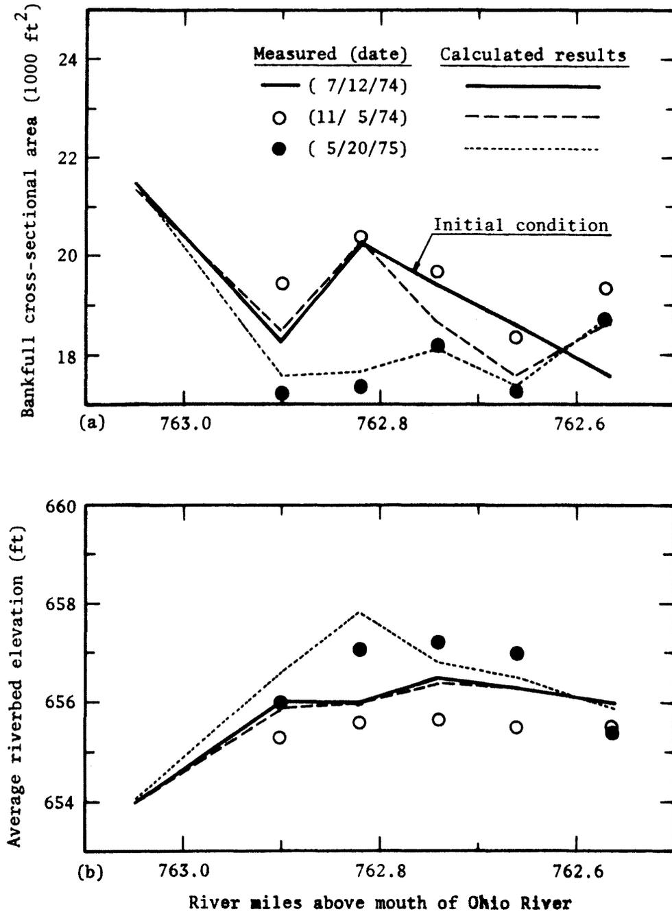
Figure 14. Mathematical model reproduction of the geomorphic changes in the Mississippi River near Readings Landing from 1974 to 1975
