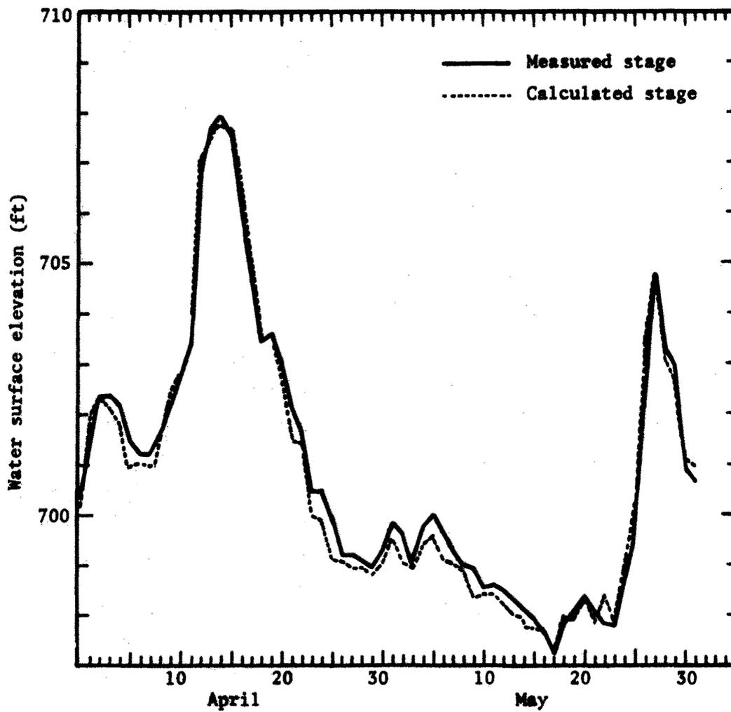
Figure 12. Mathematical model reproduction of 1971 stage hydrograph in the Chippewa River at Durand
