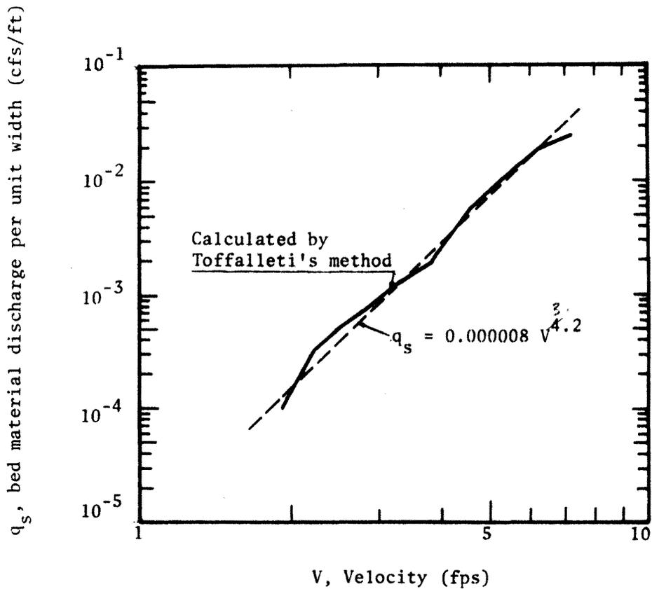
Figure 7. A typical relation between bed-material discharge and flow velocity
