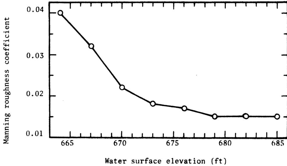
Figure 6. A typical relation between Manning roughness coefficient and stage
