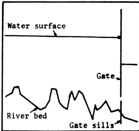
(a) Normal pool stages with control gates lowered close to gate sills
