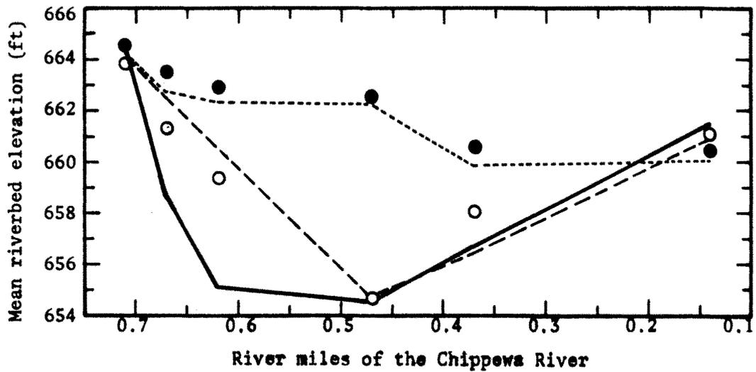
Figure 13. Mathematical model reproduction of the filling process of the 1965 dredged cut in the Lower Chippewa River
