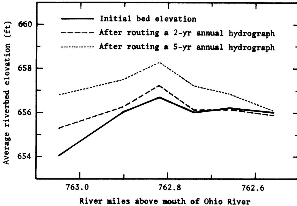
Figure 20. Riverbed elevation changes near Reads Landing after routing an annual hydrograph (without dredging)
