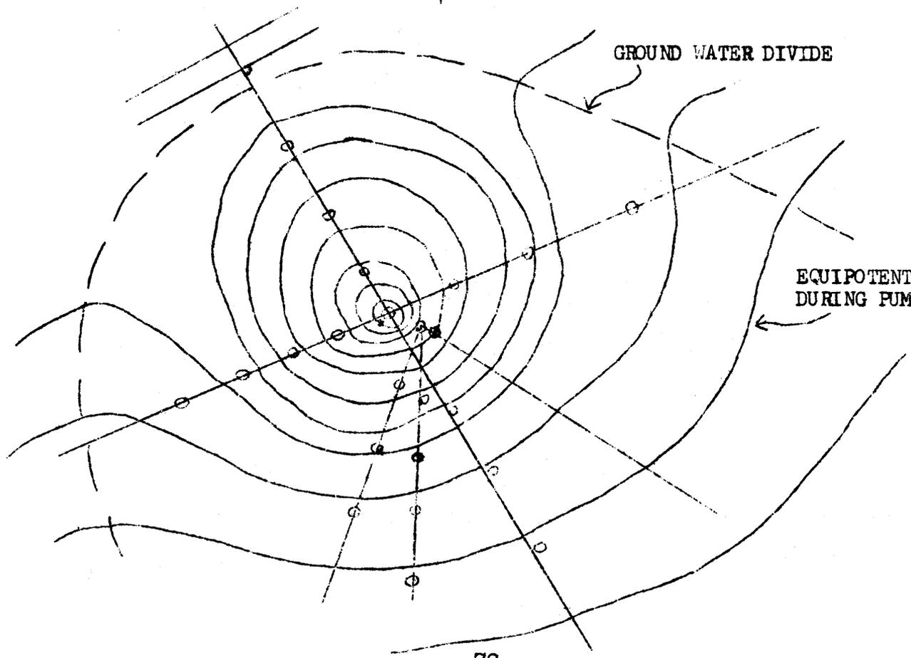
Equilibrium Conditions: Thiem formula found to apply provided  $s_1$  and  $s_2$  are averages of paired measurements, taken at equal distances,  $r_1$  and  $r_2$ , respectively, up and down the normal hydraulic slope from the well. It was accordingly developed that:
