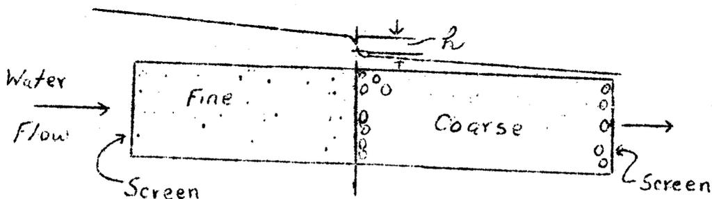
The head loss was taken as the vertical difference between tangents to the piezometric surface before and after passing through interface.
