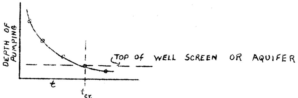
Note: Pumping below the top of the aquifer, reducing its saturated depth and consequently,  $T$ , would accelerate the rate of fall to complete failure. In the example given a 250 gpm rate would be pumping at 28' above the top of the screen when 300 gpm would be dewatering the aquifer.
