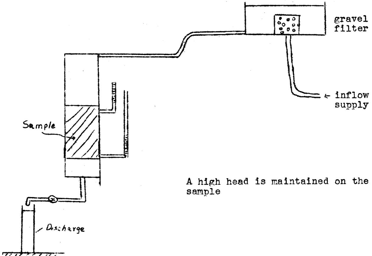
The soil sample tested ranged in height from 6" to 12".
