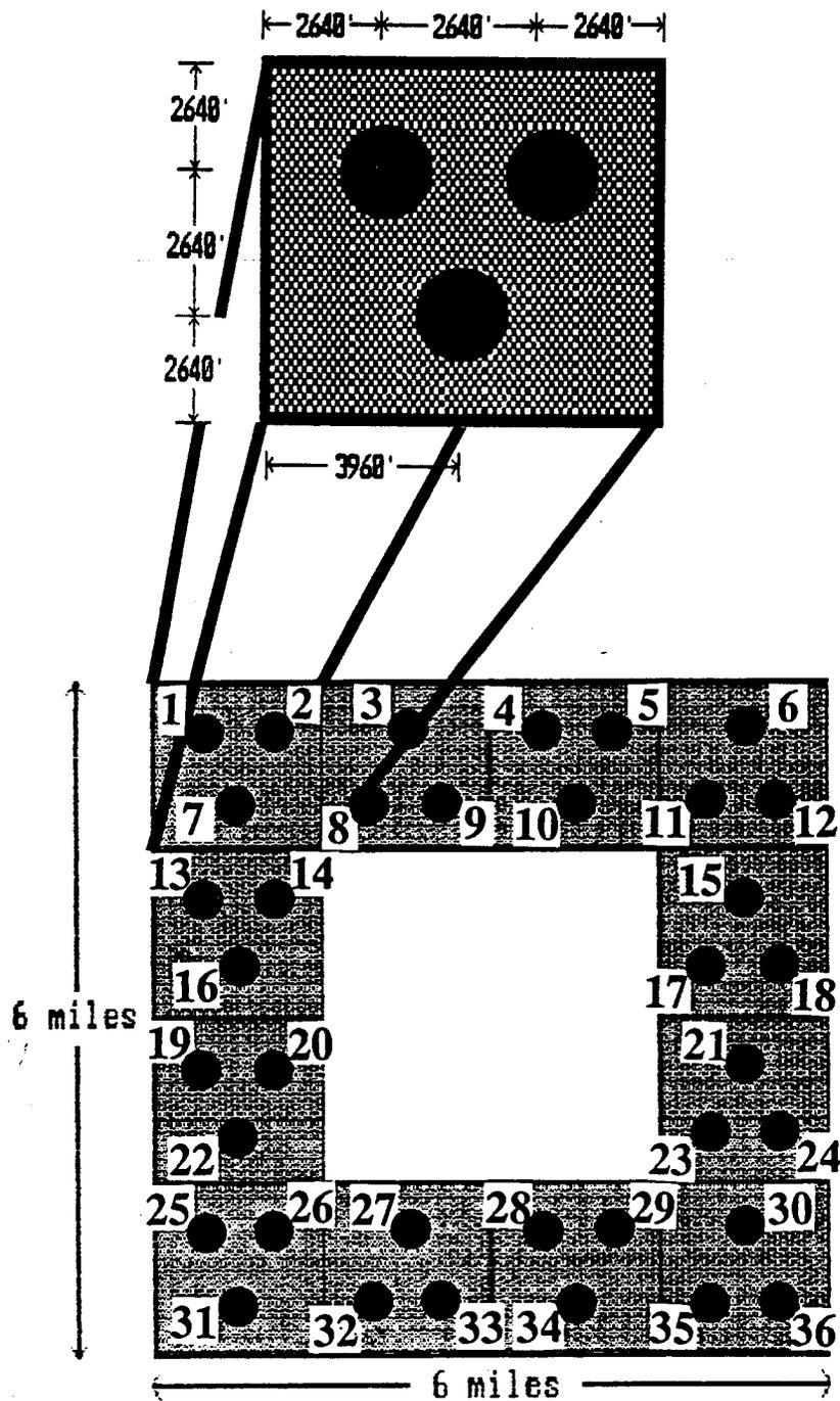
Figure 17. Well field configuration and dimensions
