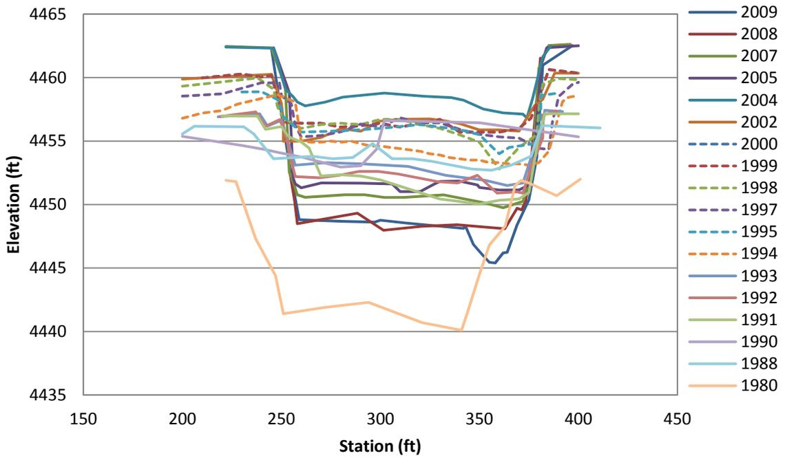
Figure 4.33 Subreach 5: EB-20 Surveyed Cross-Sections
