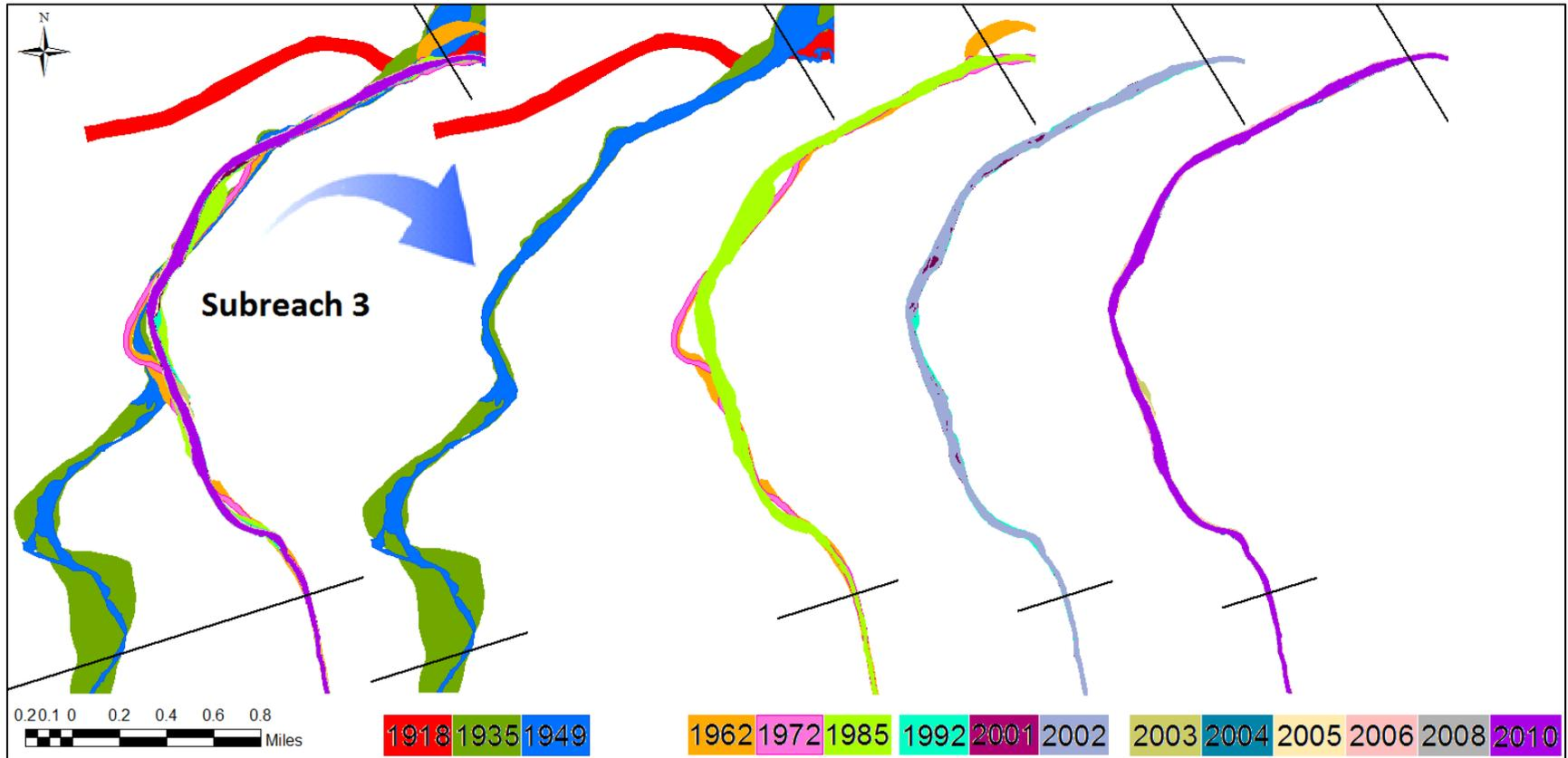
Figure 4.4 Subreach 3 Channel Planforms from Aerial Photography
