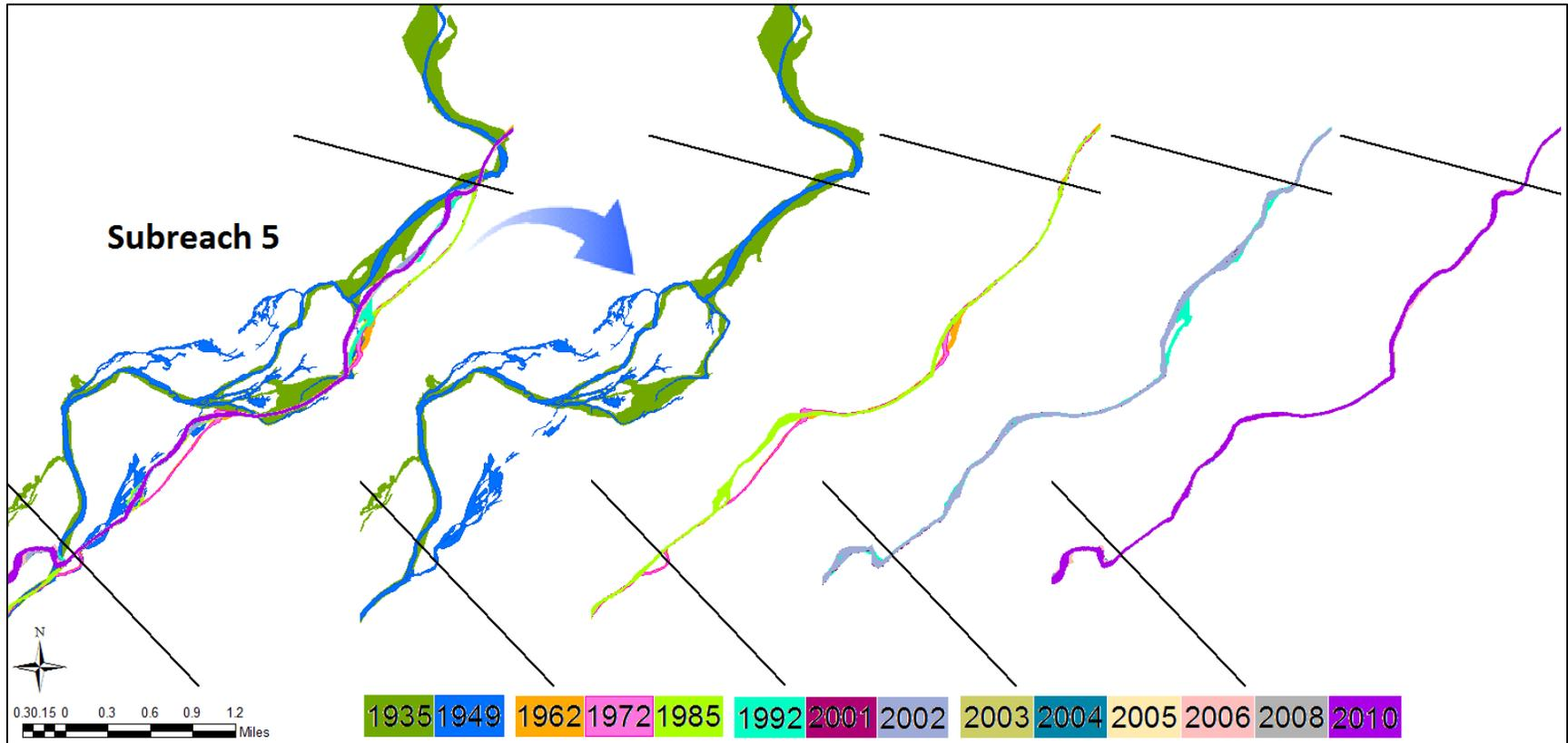
Figure 4.6 Subreach 5 Channel Planforms from Aerial Photography
