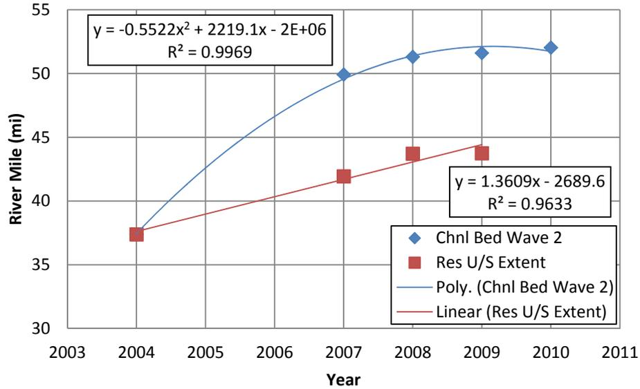
Figure 4.50 Rate of Wave 2 Propagation Upstream
