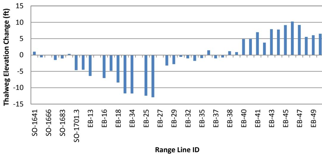
Figure 4.44 Change in Thalweg Elevation from 2004 to 2009
