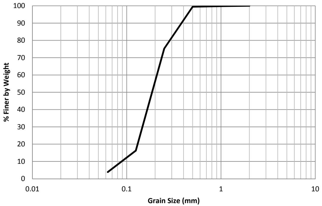
Figure H.35 EB-24 2002 Grain Size Distribution
