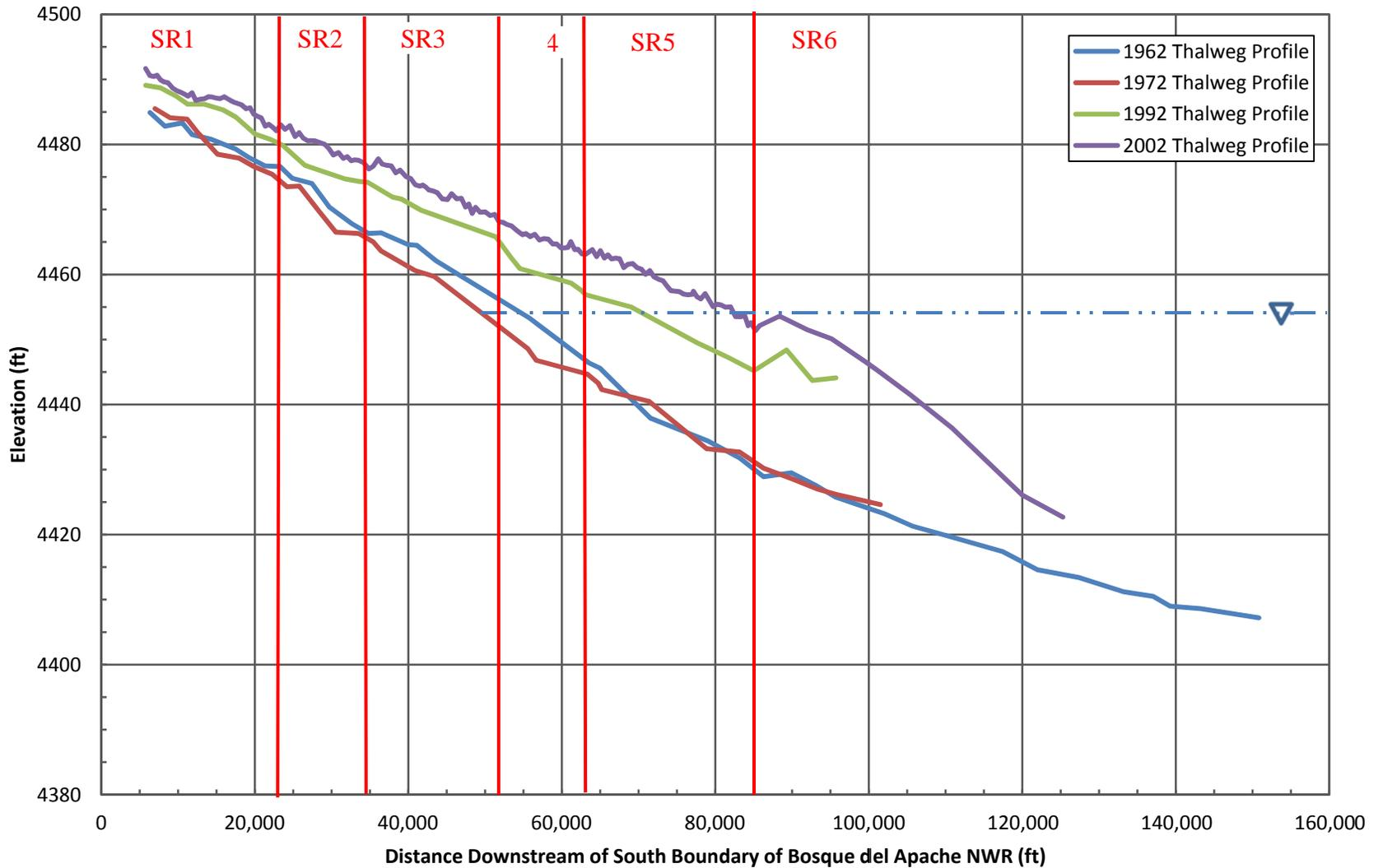
Figure 4.12 Thalweg Elevation Profile From Agg/Deg Surveys
