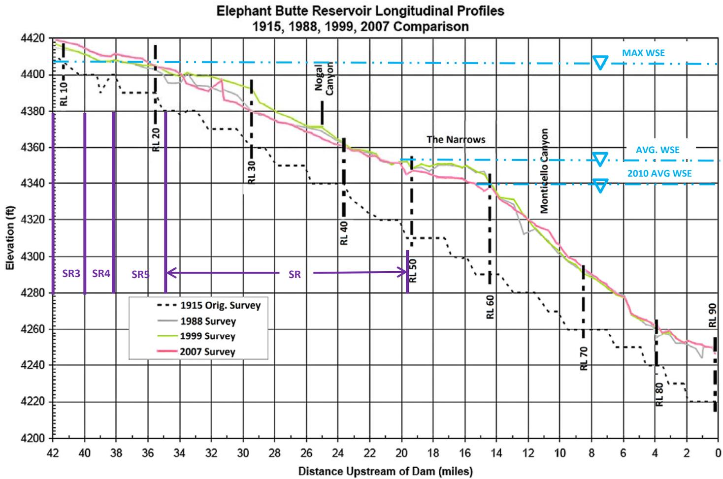
Figure 95 - Elephant Butte Reservoir Longitudinal Profiles
