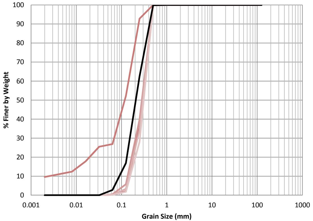
Figure H.30 EB-18 1999 Grain Size Distribution
