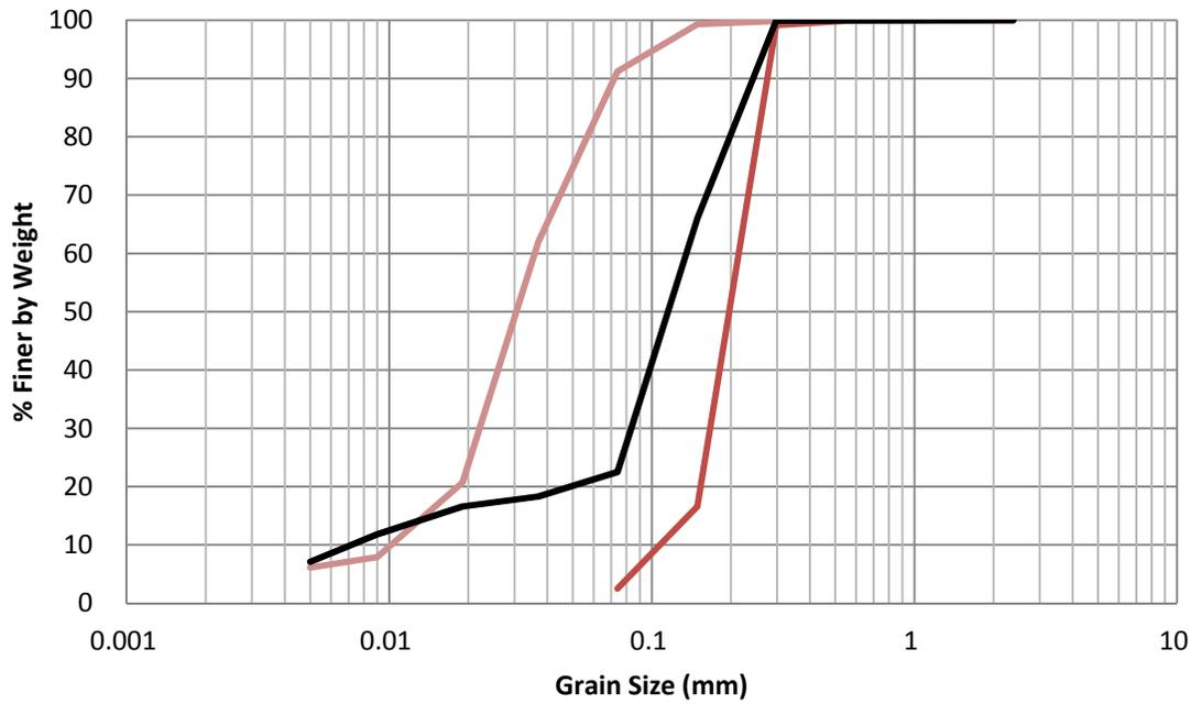
Figure H.20 EB-13 1990 Grain Size Distribution
