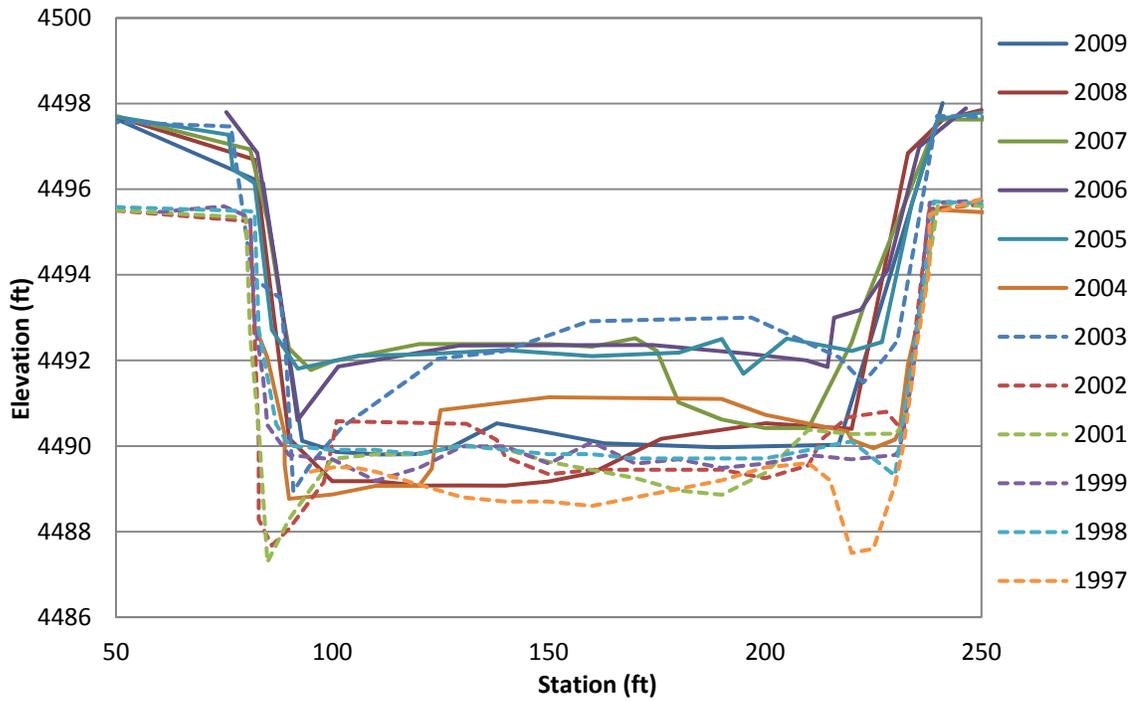
Figure 4.28 Subreach 1: SO-1641 Surveyed Cross-Sections
