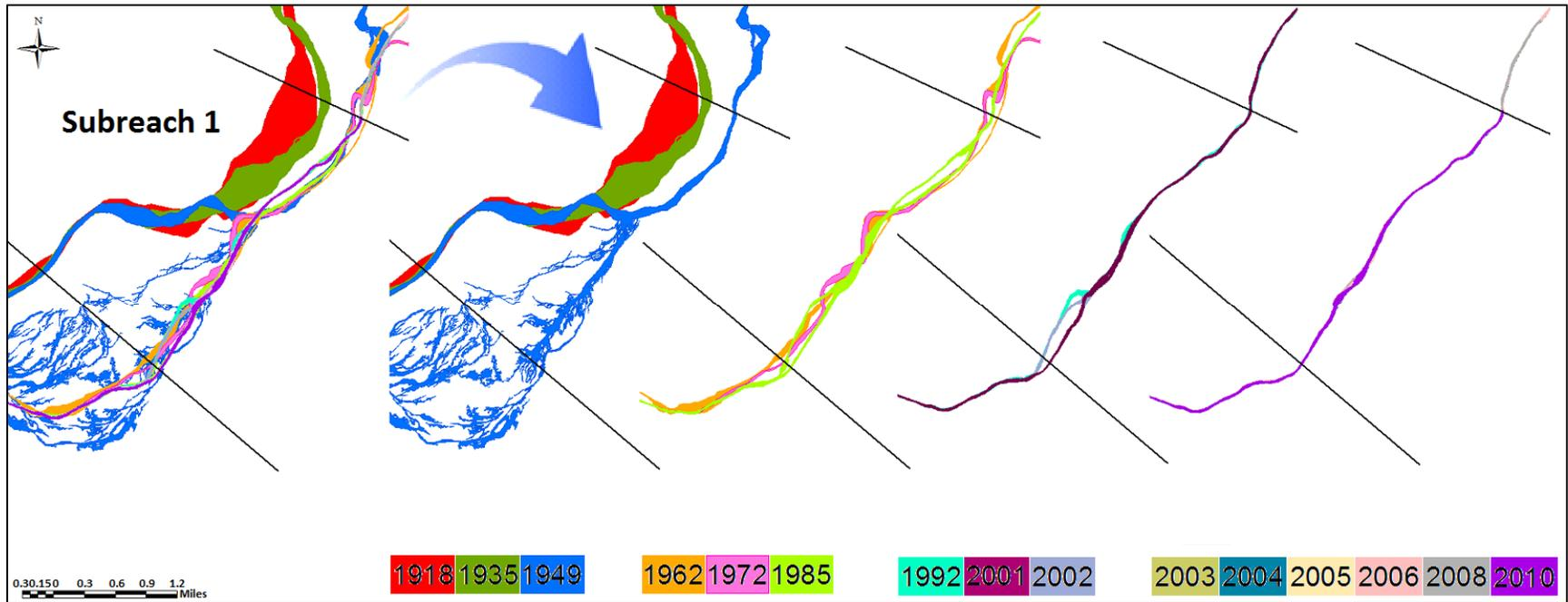
Figure 4.2 Subreach 1 Channel Planforms from Aerial Photography
