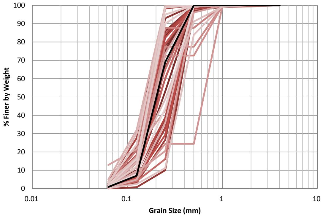
Figure H.11 EB-10 1993 Grain Size Distribution
