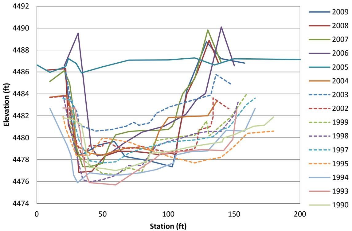
Figure 4.29 Subreach 2: SO-1683 Surveyed Cross-Sections
