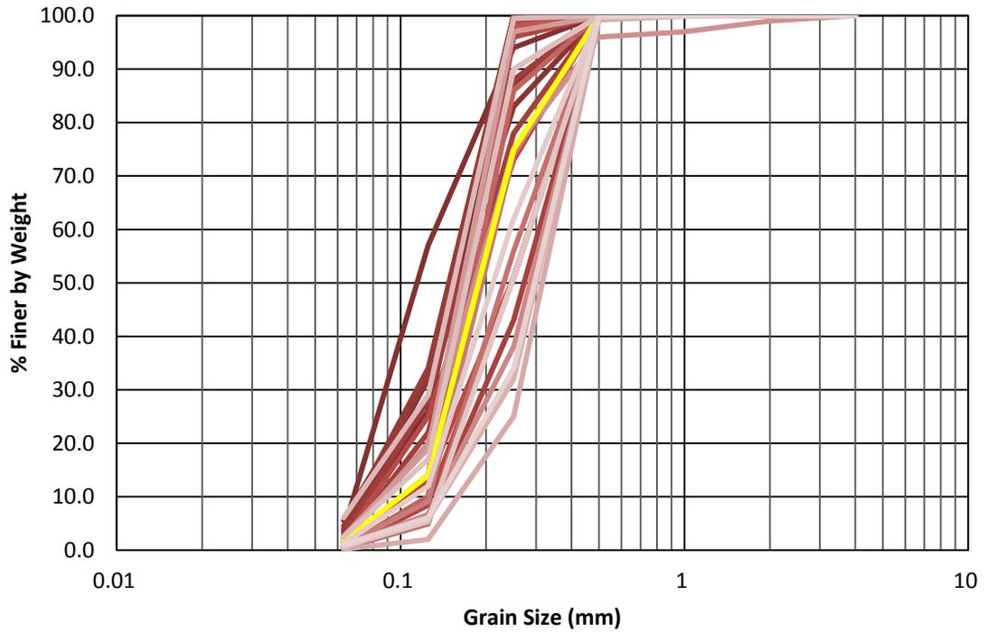
Figure 4.55 EB-10 1992 Bed Material Grain Size Distributions
