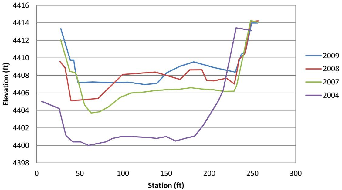
Figure 4.36 Subreach 6: EB-41 Surveyed Cross-Sections
