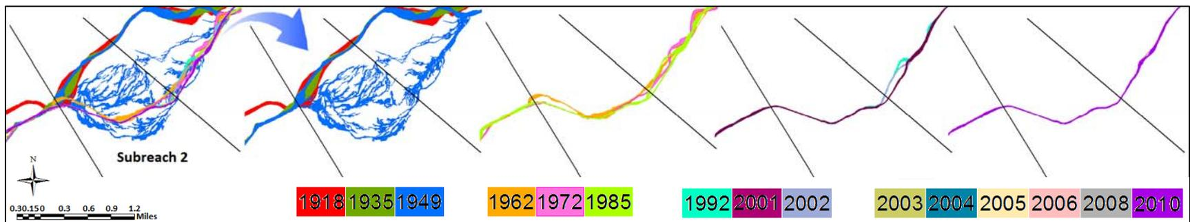
Figure 4.3 Subreach 2 Channel Planforms from Aerial Photography
