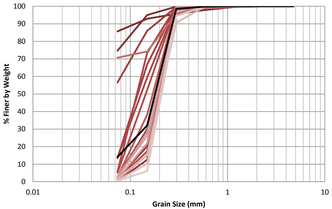
Figure H.18 EB-13 1987 Grain Size Distribution
