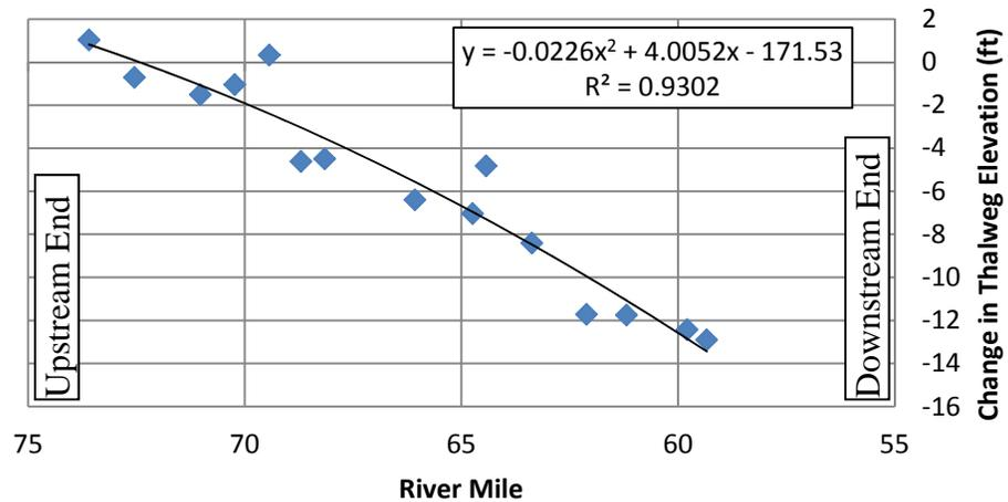
Figure 4.45 Magnitude of Degradation from 2004 to 2009
