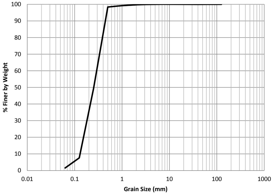
Figure H.31 EB-18 2002 Grain Size Distribution
