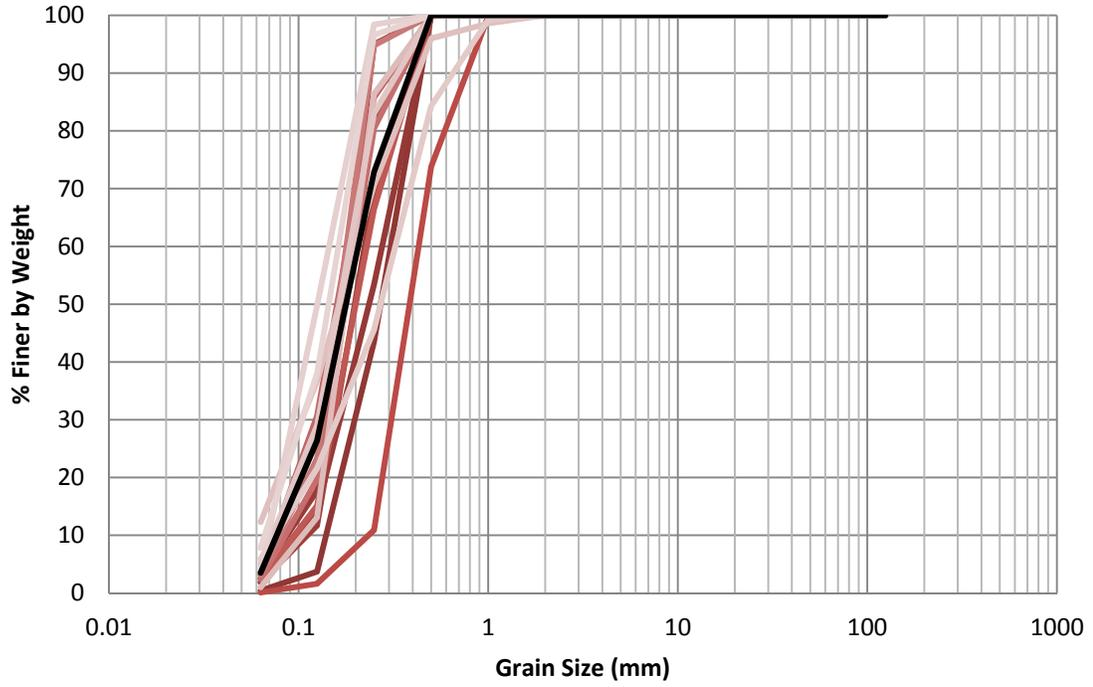
Figure H.27 EB-18 1993 Grain Size Distribution
