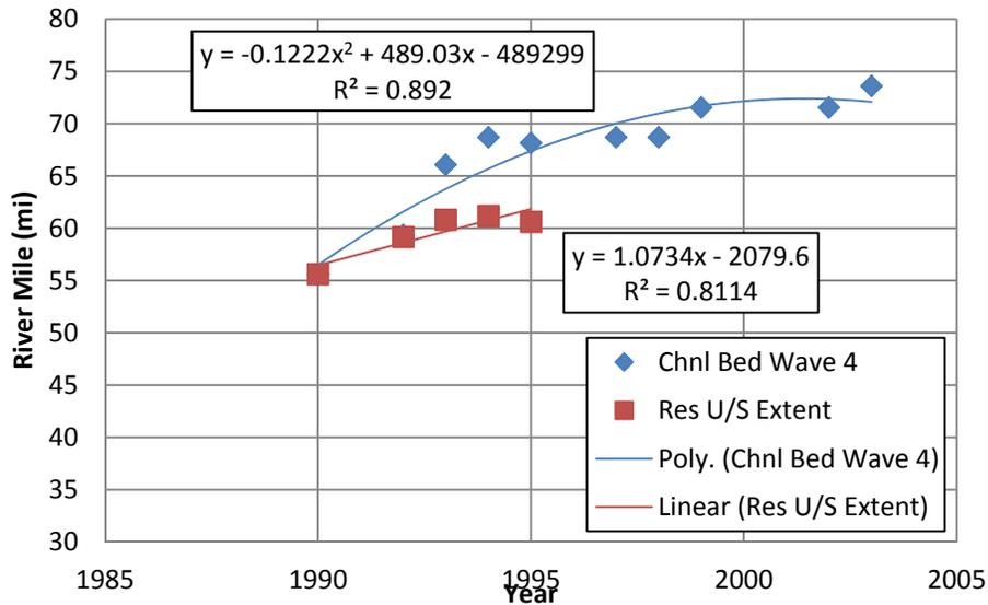
Figure 4.54 Rate of Wave 4 Propagation Upstream
