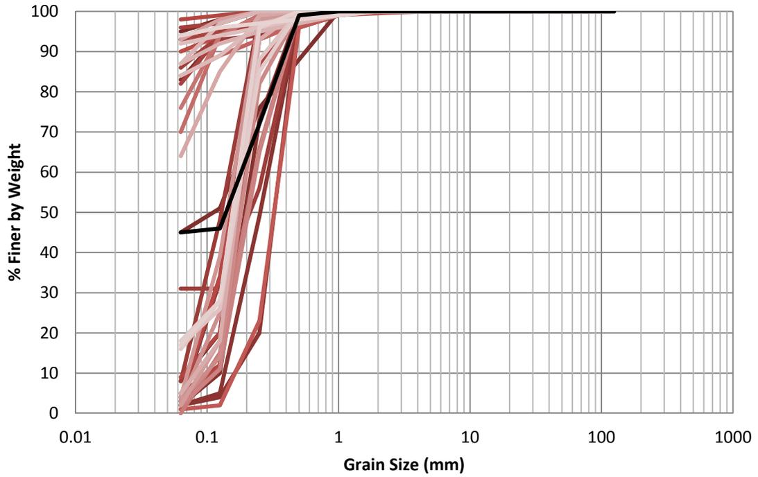
Figure H.28 EB-18 1994 Grain Size Distribution
