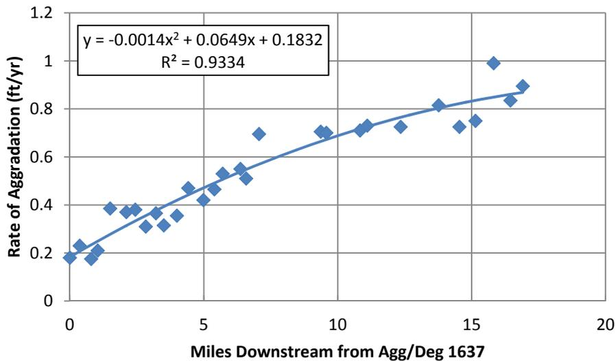
Figure 4.20 Rate of Channel Aggradation between 1972 and 1992
