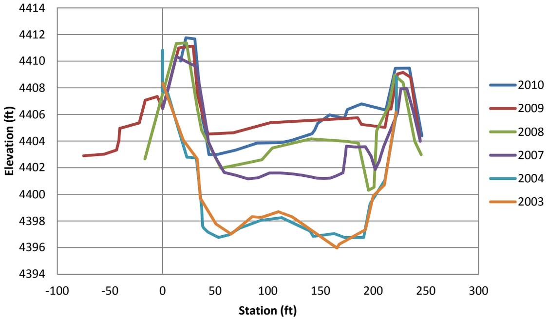
Figure F.42 EB-44 Cross-Section
