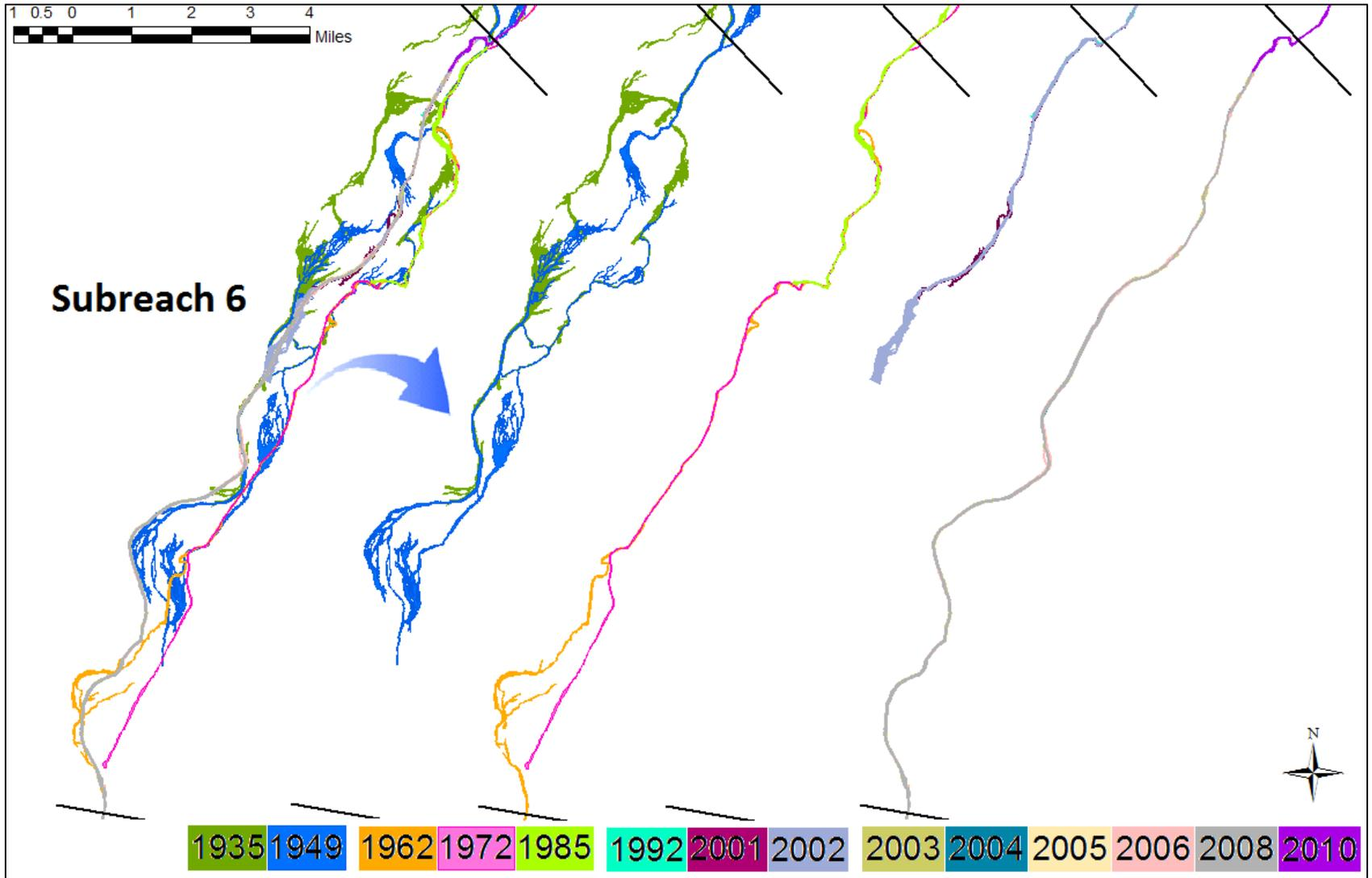
Figure 4.7 Subreach 6 Channel Planforms from Aerial Photography
