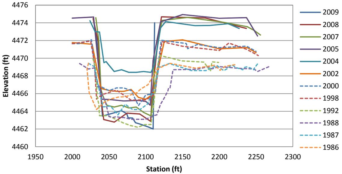
Figure 4.32 Subreach 4: EB-13 Surveyed Cross-Sections
