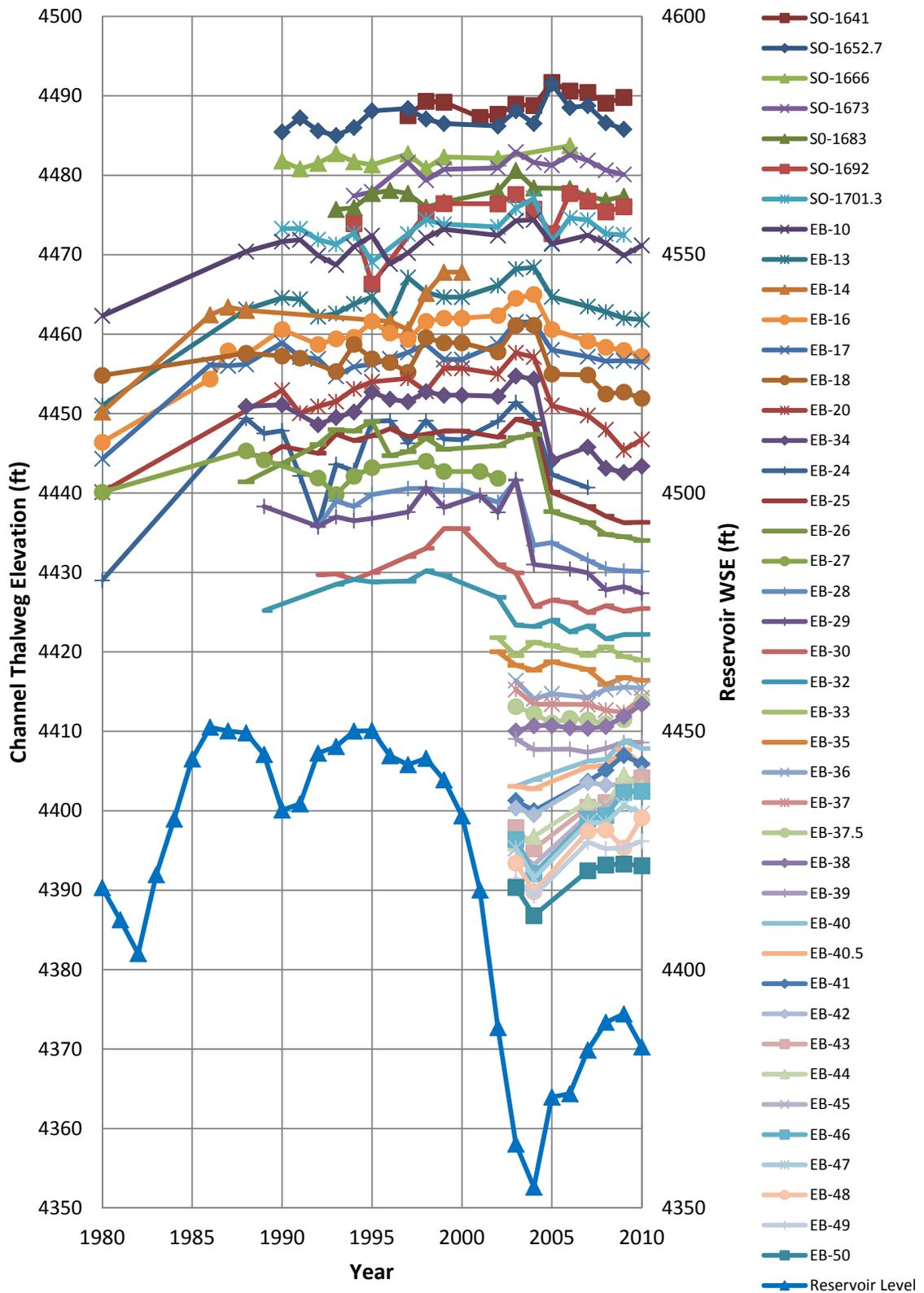
Figure 4.37 Change in Thalweg Elevation at Range Lines (1980 – 2010)
