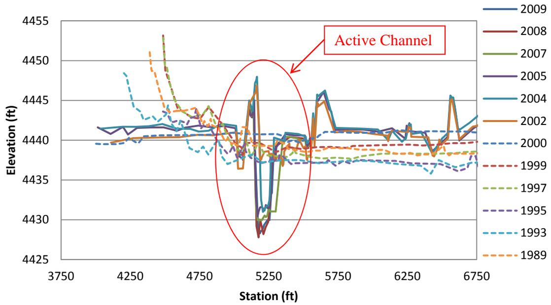
Figure 4.35 Subreach 6: EB-29 (w/Floodplain) Surveyed Cross-Sections
