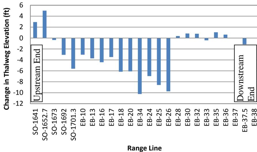
Figure 4.42 Magnitude of Aggradation and Degradation at Range Lines (2004-2005)
