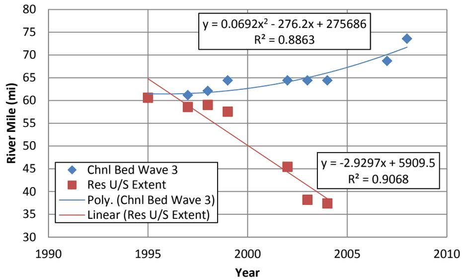
Figure 4.52 Rate of Wave 3 Propagation Upstream
