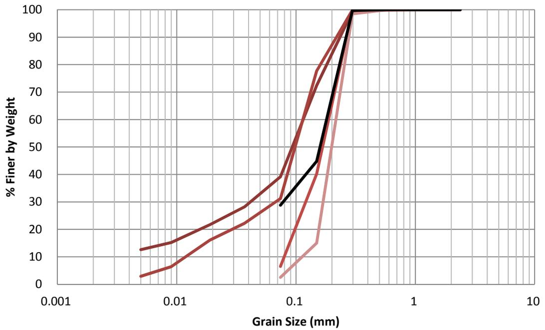
Figure H.26 EB-18 1990 Grain Size Distribution
