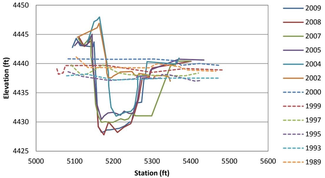
Figure 4.34 Subreach 6: EB-29 Surveyed Cross-Sections
