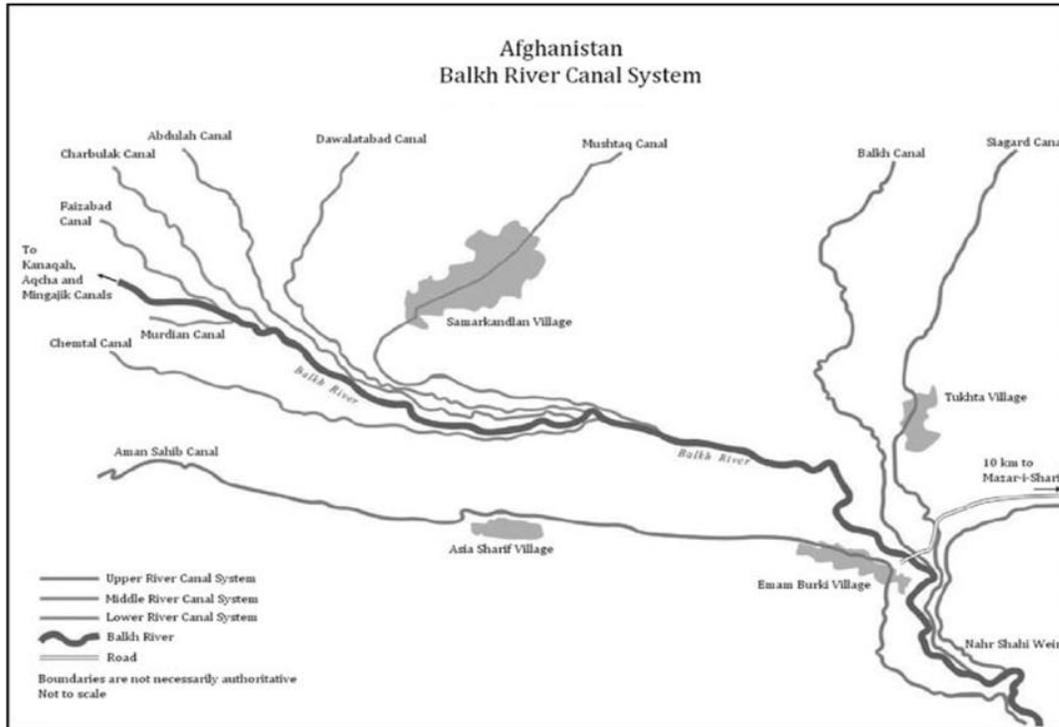
Figure 4.3: Schematic of the Balkh River Canal System, Afghanistan Source: Torrell and Ward, 2010
