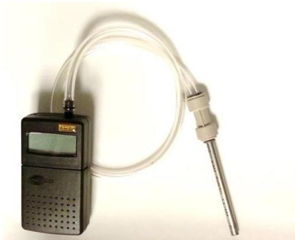
**Figure 1: Tenax TA sampling apparatus: a stainless steel tube filled with Tenax TA sorbent media and connected to a personal sampling pump with a push-to-connect adapter**
