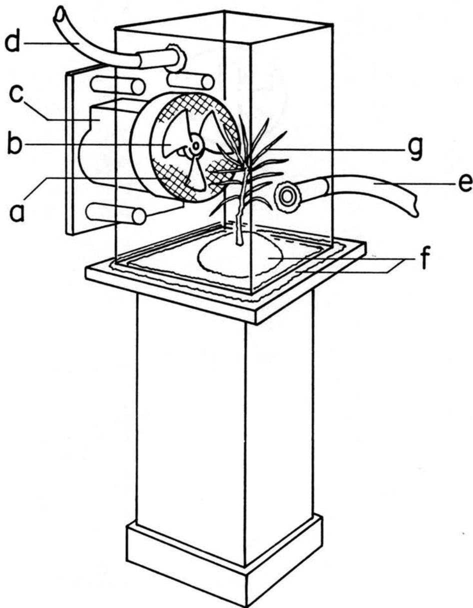
Figure 2. Diagrammatic representation of the assimilation chamber used to measure  $\text{CO}_2$  exchange in an open system of infrared gas analysis (IRGA). (a) Nylon mesh. (b) Fan. (c) Magnetic motor. (d) Inlet tygon tube. (e) Outlet tygon tube. (f) Terostat sealant. (g) Pine seedling.
