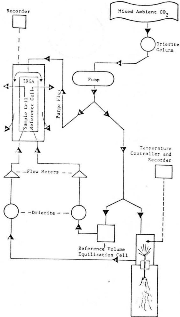
Figure 1. Schematic drawing of the open system of infrared gas analysis (IRGA) used to measure CO<sub>2</sub> exchange of pine seedlings.
