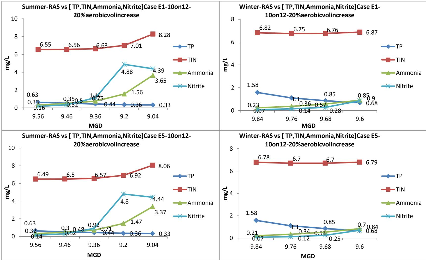
Figure B-12: Effluent concentrations for 10 MGD influent flow in reactors with 10% increase in anaerobic, anoxic and 20 % increase in aerator volume for summer and winter conditions, 10 MGD internal recycle Cases E1 and E5
