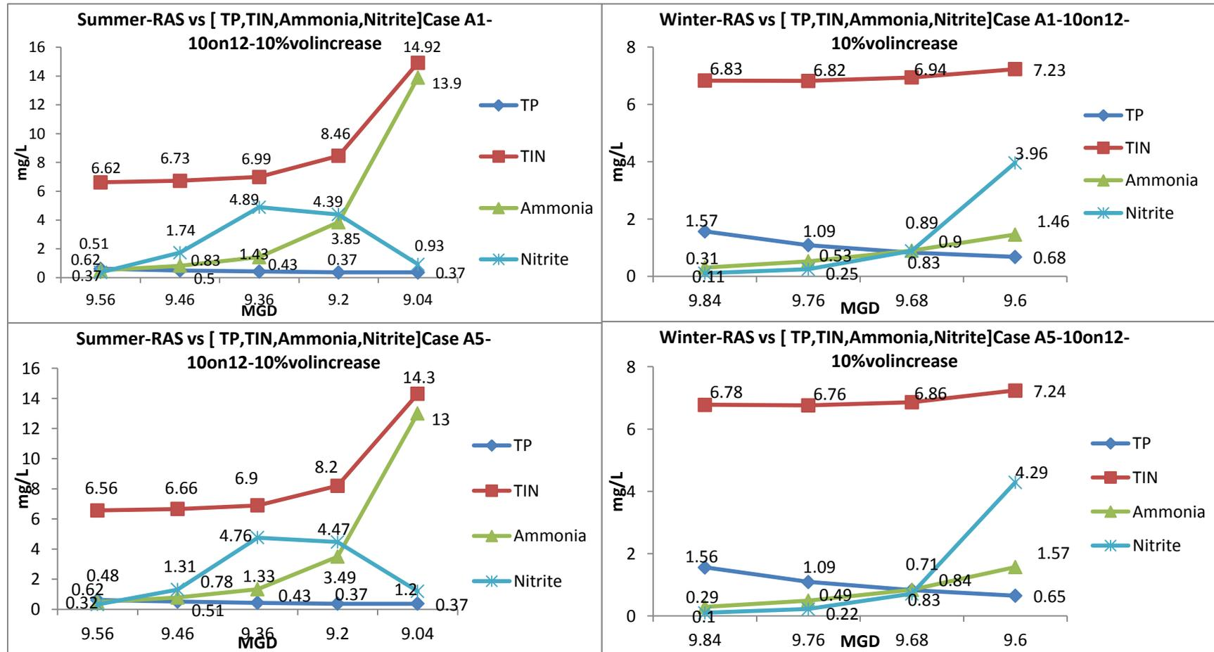
Figure B-1: Effluent concentrations for 10 MGD influent flow in reactors with 10 % increase in volume for summer and winter conditions, 10 MGD internal recycle Cases A1 and A5
