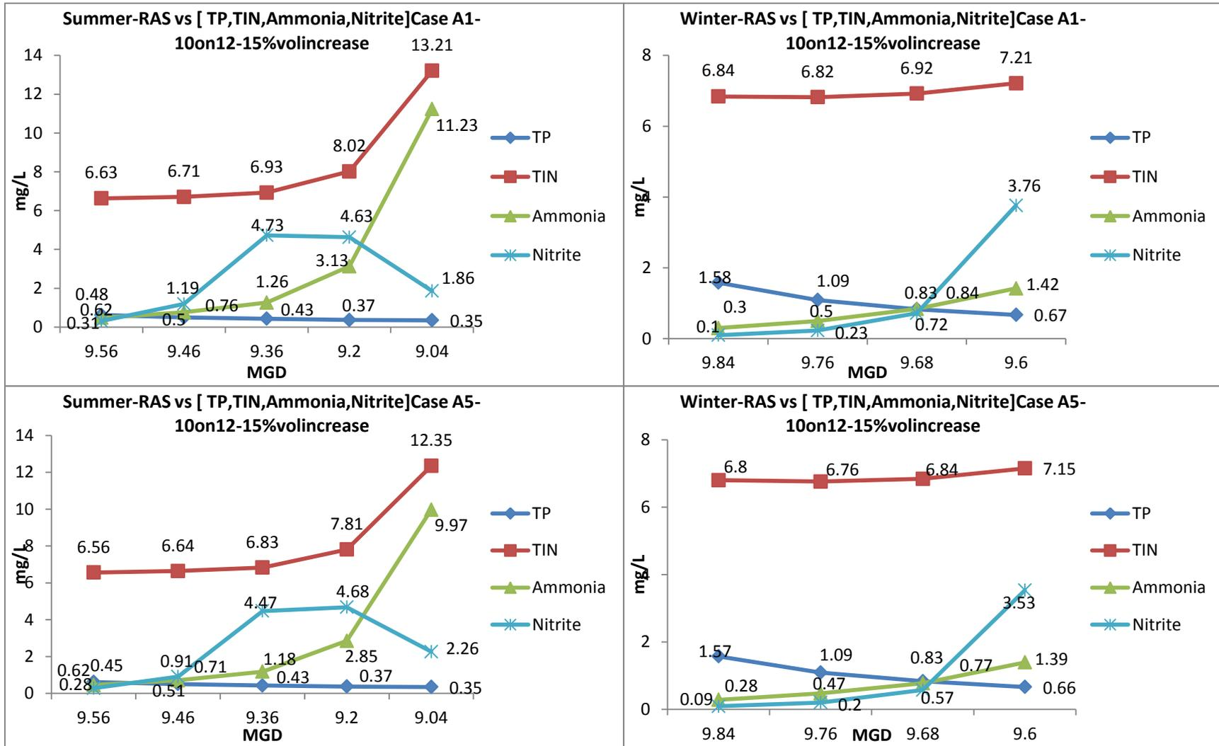
Figure B-4: Effluent concentrations for 10 MGD influent flow in reactors with 15 % increase in volume for summer and winter conditions, 10 MGD internal recycle Cases A1 and A5
