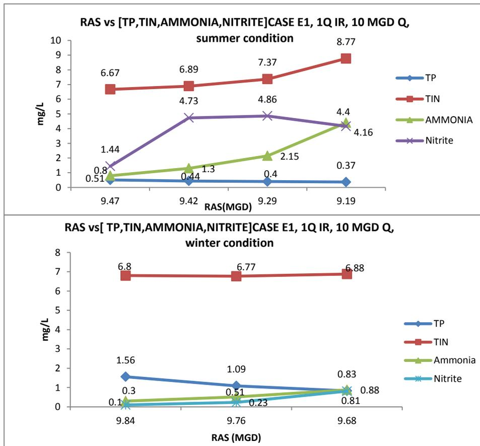
Figure 4.7: Effluent concentration for case E1 summer condition (top) and winter condition (bottom)
