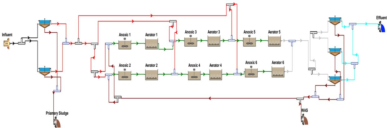
Figure 2.1. Wastewater treatment plant model in BioWin
