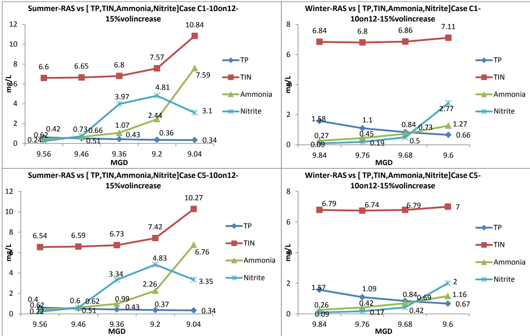
Figure B-5: Effluent concentrations for 10 MGD influent flow in reactors with 15 % increase in volume for summer and winter conditions, 10 MGD internal recycle Cases C1 and C5
