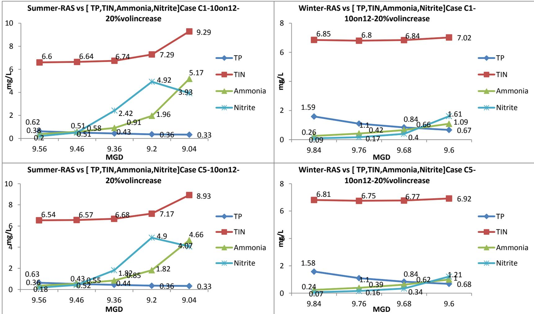
Figure B-8: Effluent concentrations for 10 MGD influent flow in reactors with 20 % increase in volume for summer and winter conditions, 10 MGD internal recycle Cases C1 and C5
