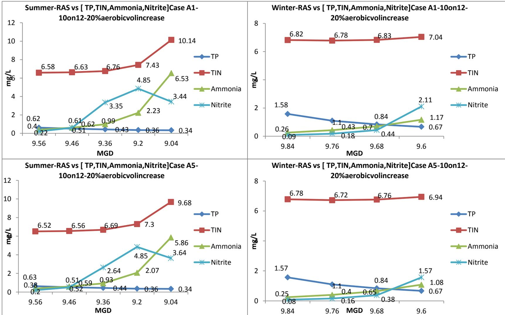
Figure B-10: Effluent concentrations for 10 MGD influent flow in reactors with 10% increase in anaerobic, anoxic and 20 % increase in aerator volume for summer and winter conditions, 10 MGD internal recycle Cases A1 and A5
