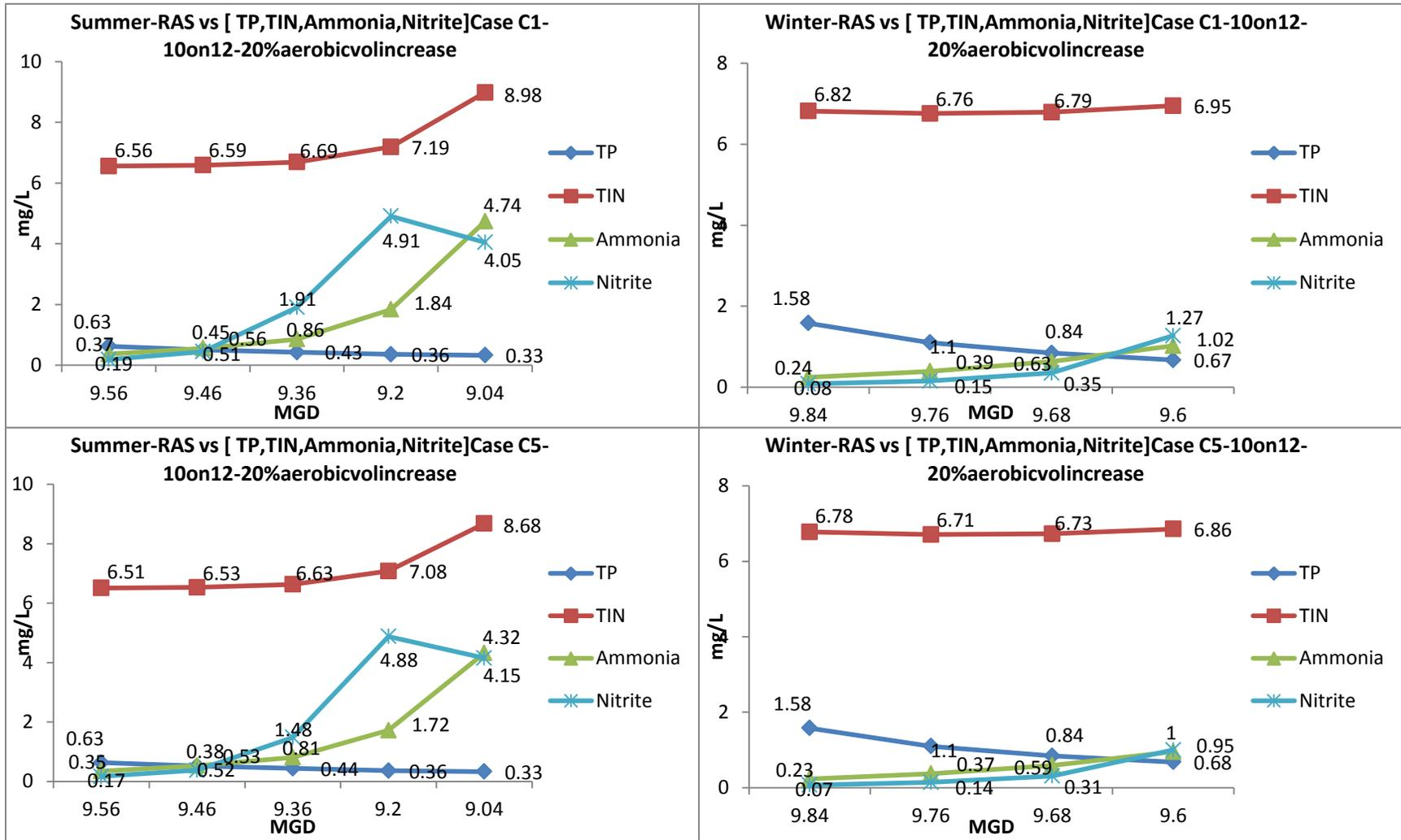
Figure B-11: Effluent concentrations for 10 MGD influent flow in reactors with 10% increase in anaerobic, anoxic and 20 % increase in aerator volume for summer and winter conditions, 10 MGD internal recycle Cases C1 and C5
