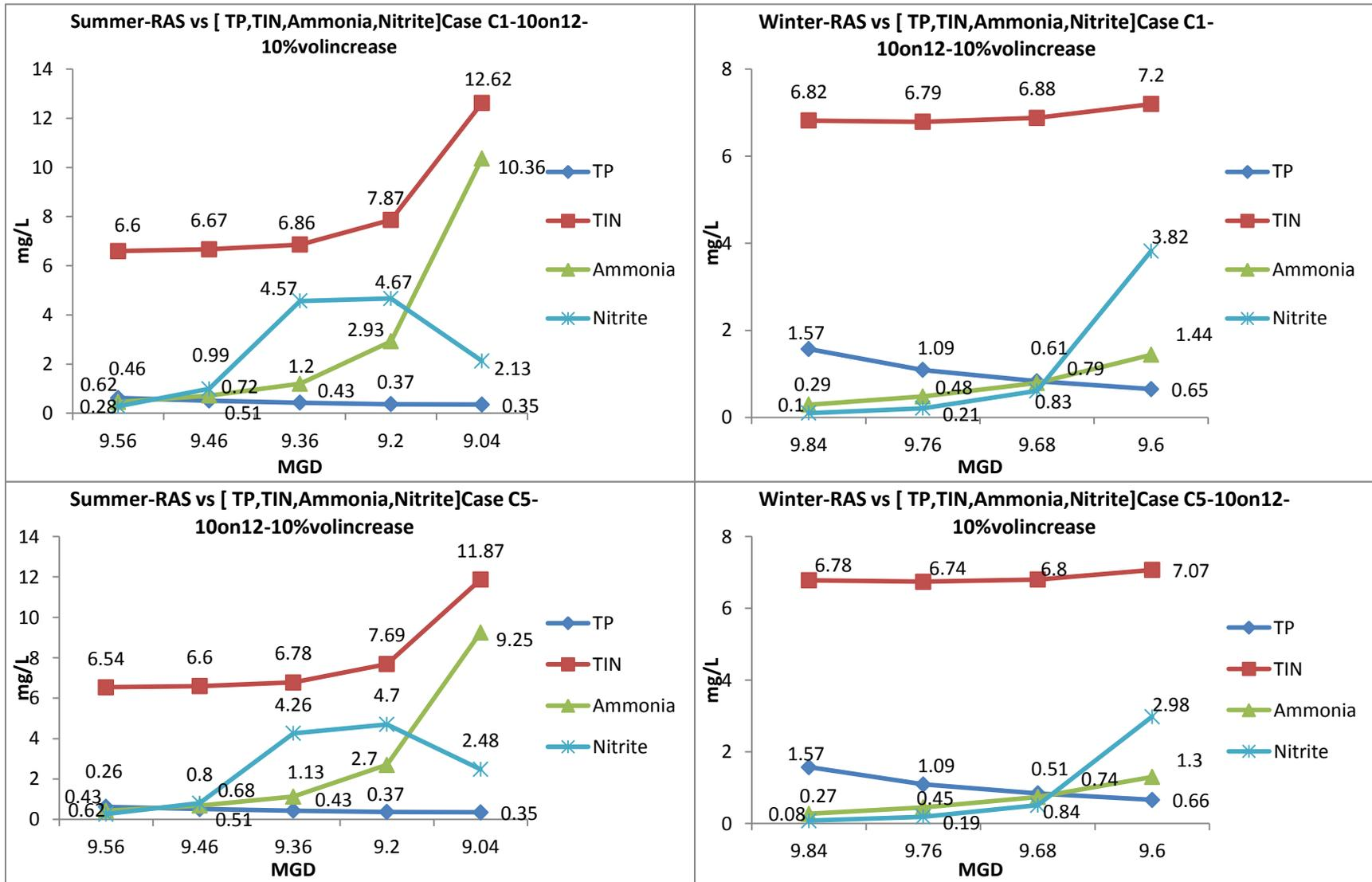
Figure B-2: Effluent concentrations for 10 MGD influent flow in reactors with 10 % increase in volume for summer and winter conditions, 10 MGD internal recycle Cases C1 and C5
