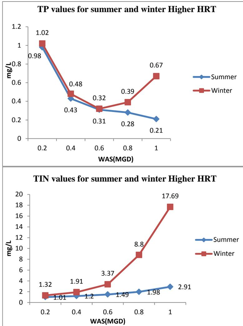
Figure 4.11: Effluent TP and TIN concentrations for higher design HRT
