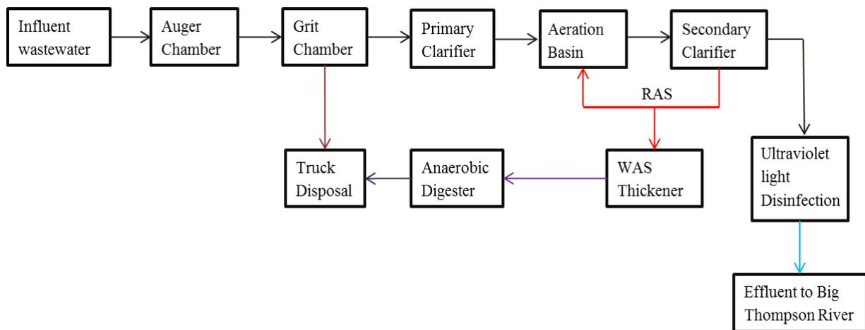
Figure 4.1: BioWin model of existing WWTP step feed activated sludge process
