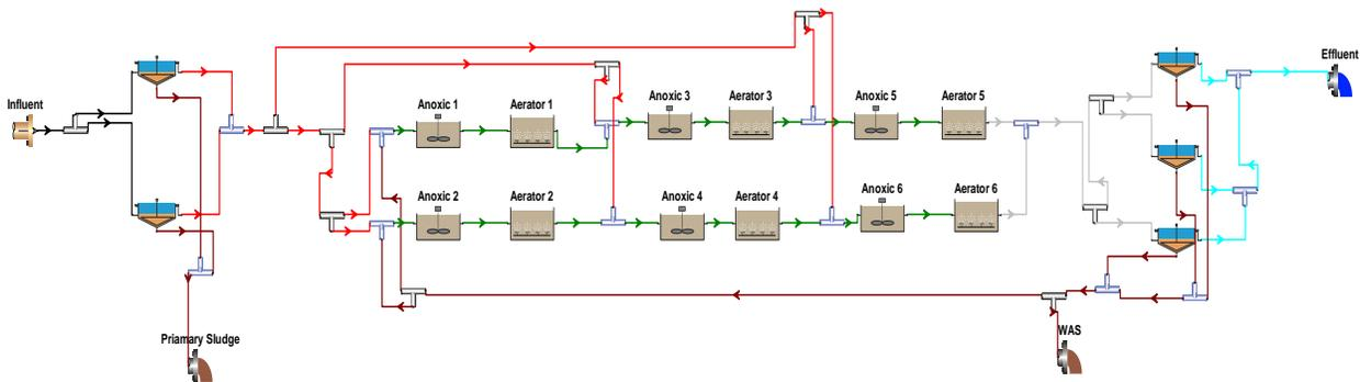
Figure 4.3: BioWin model of existing step feed activated sludge process
