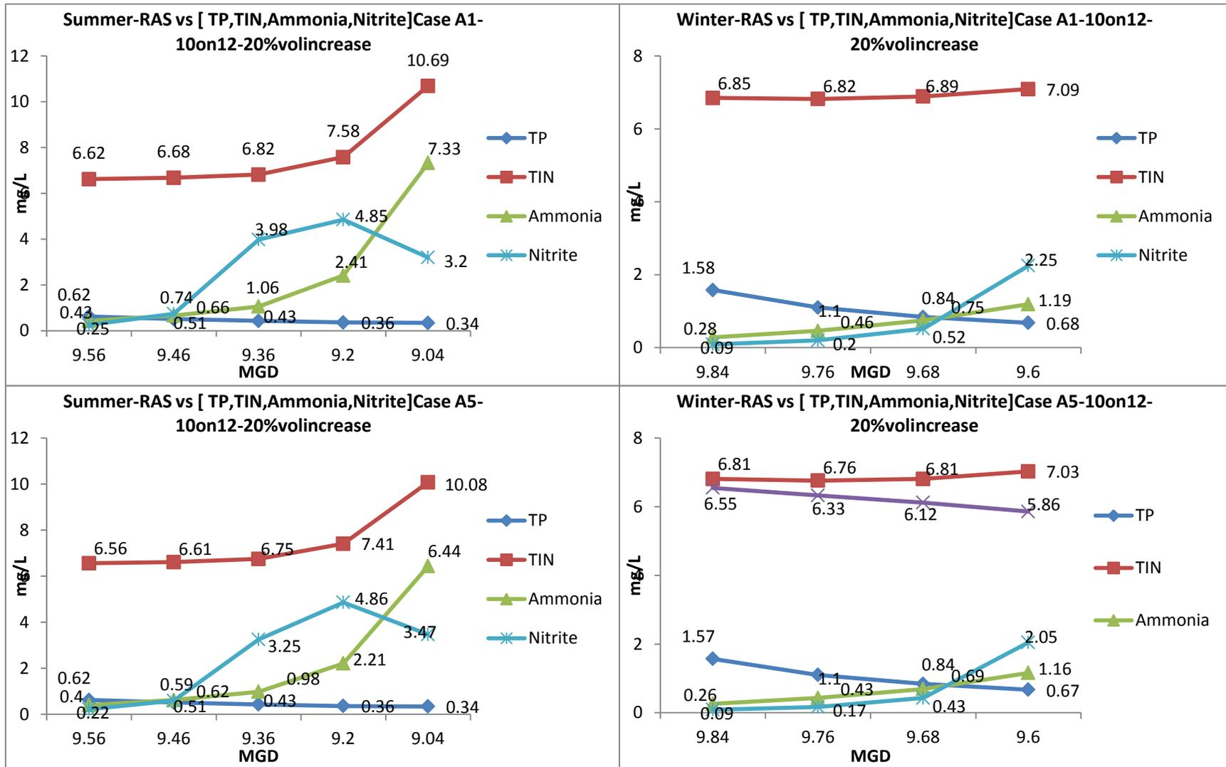
Figure B-7: Effluent concentrations for 10 MGD influent flow in reactors with 20 % increase in volume for summer and winter conditions, 10 MGD internal recycle Cases A1 and A5
