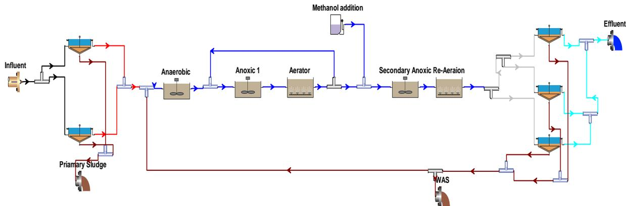
Figure 4.6: BioWin model of proposed 5-stage Bardenpho process
