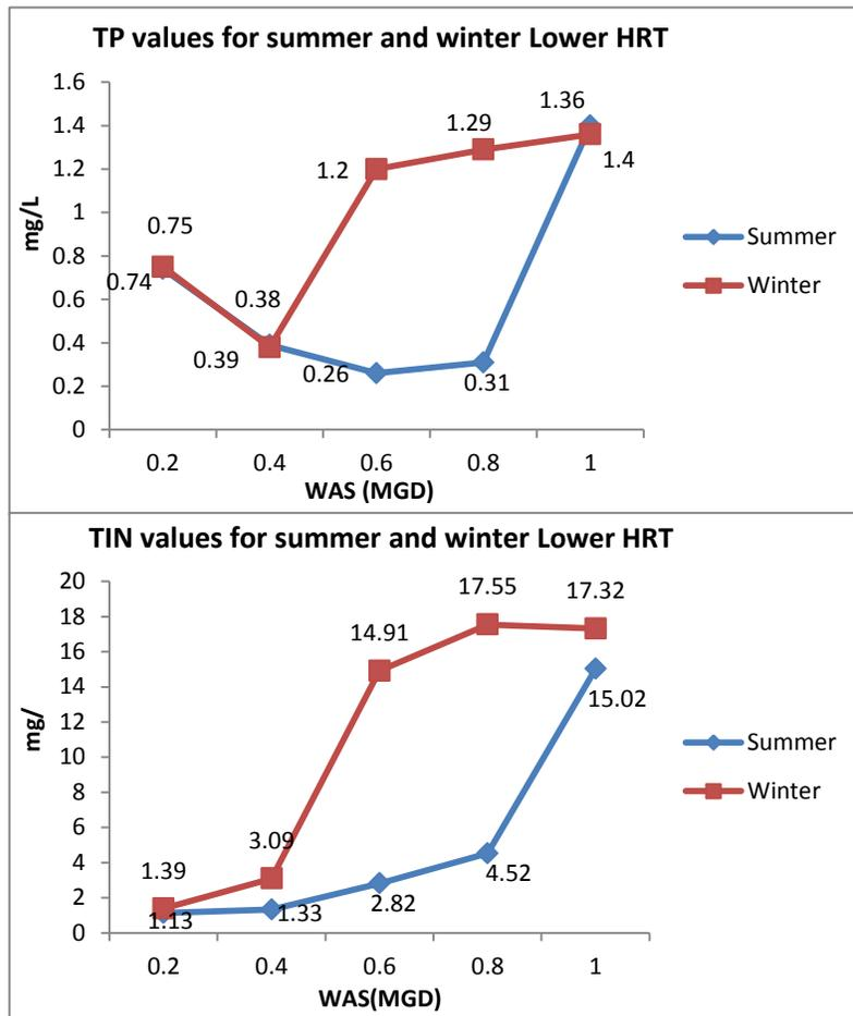
Figure 4.10: Effluent TP and TIN concentrations for lower design HRT
