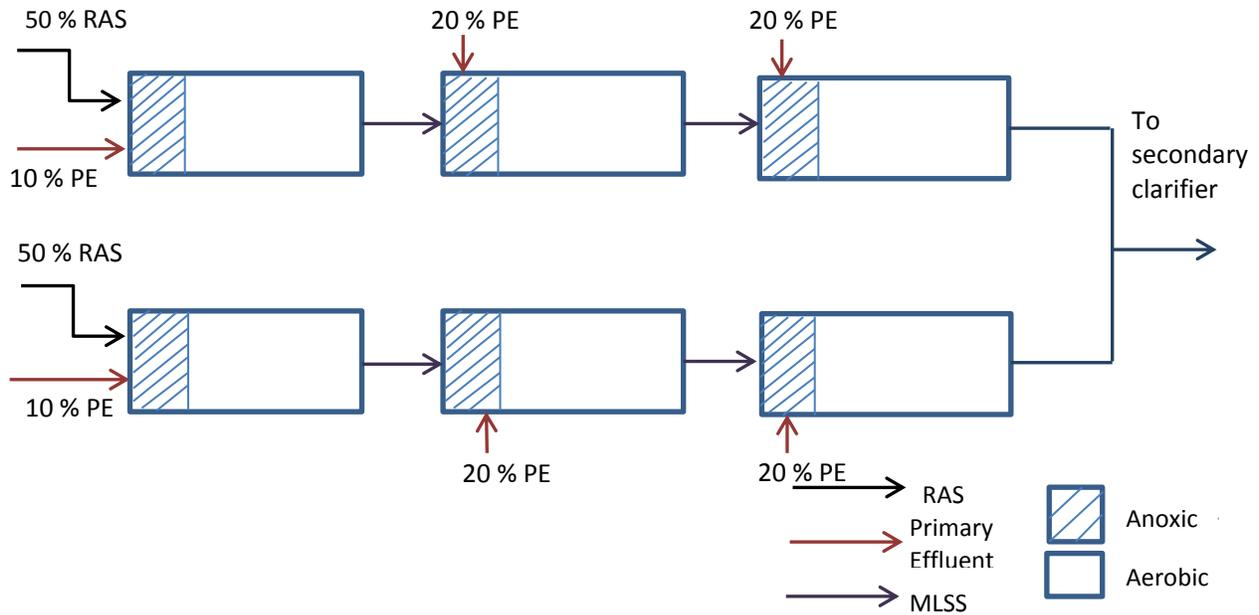
Figure 4.2: Step feed process configuration for City of Loveland WWTP
