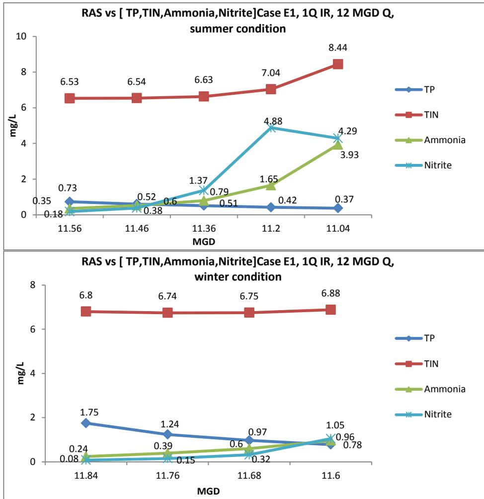
Figure 4.9: Case E1, 10 % anaerobic, anoxic volume increase, 20% aerobic volume increase, summer (top) and winter (bottom) condition
