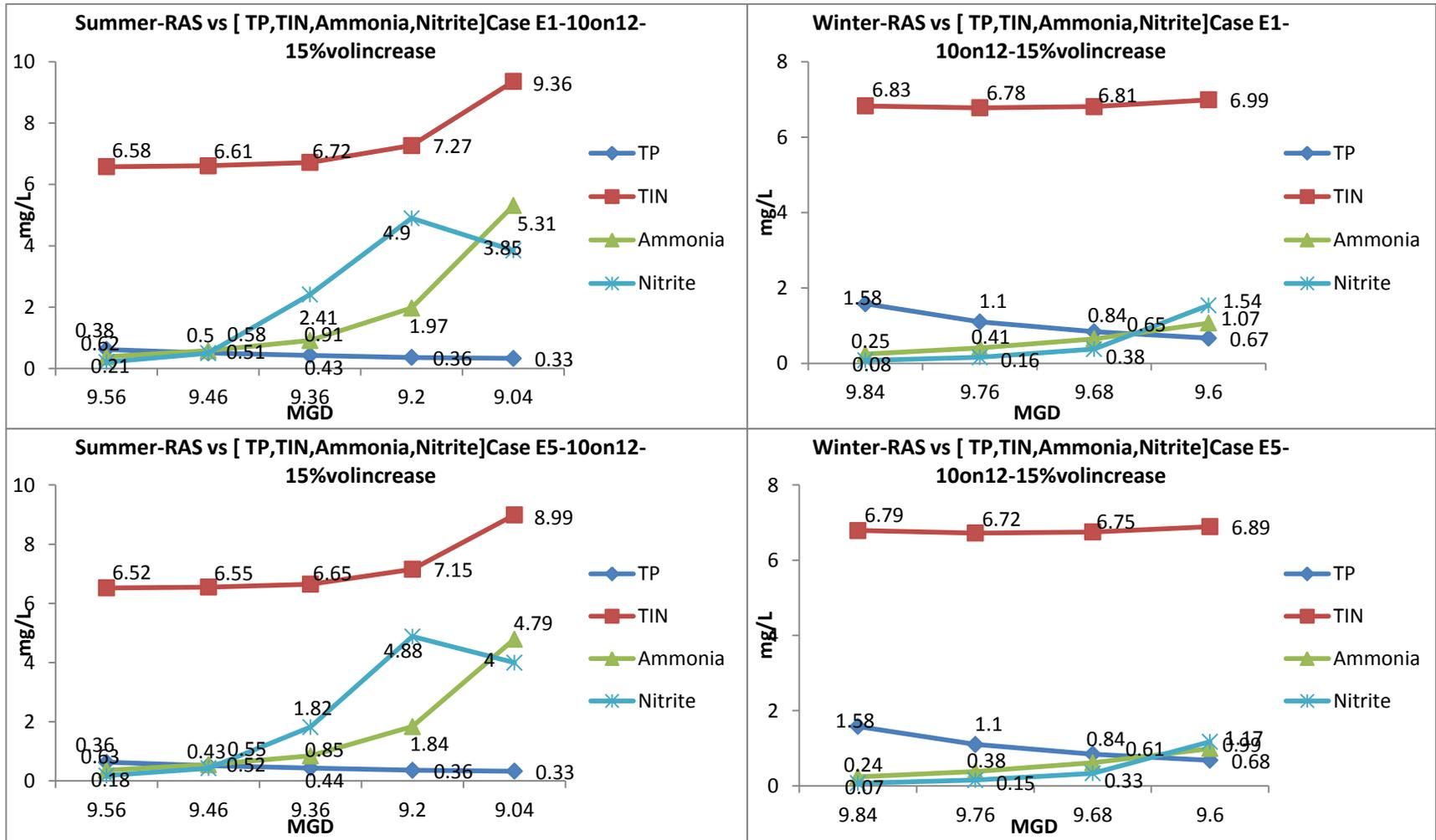
Figure B-6: Effluent concentrations for 10 MGD influent flow in reactors with 15 % increase in volume for summer and winter conditions, 10 MGD internal recycle Cases E1 and E5
