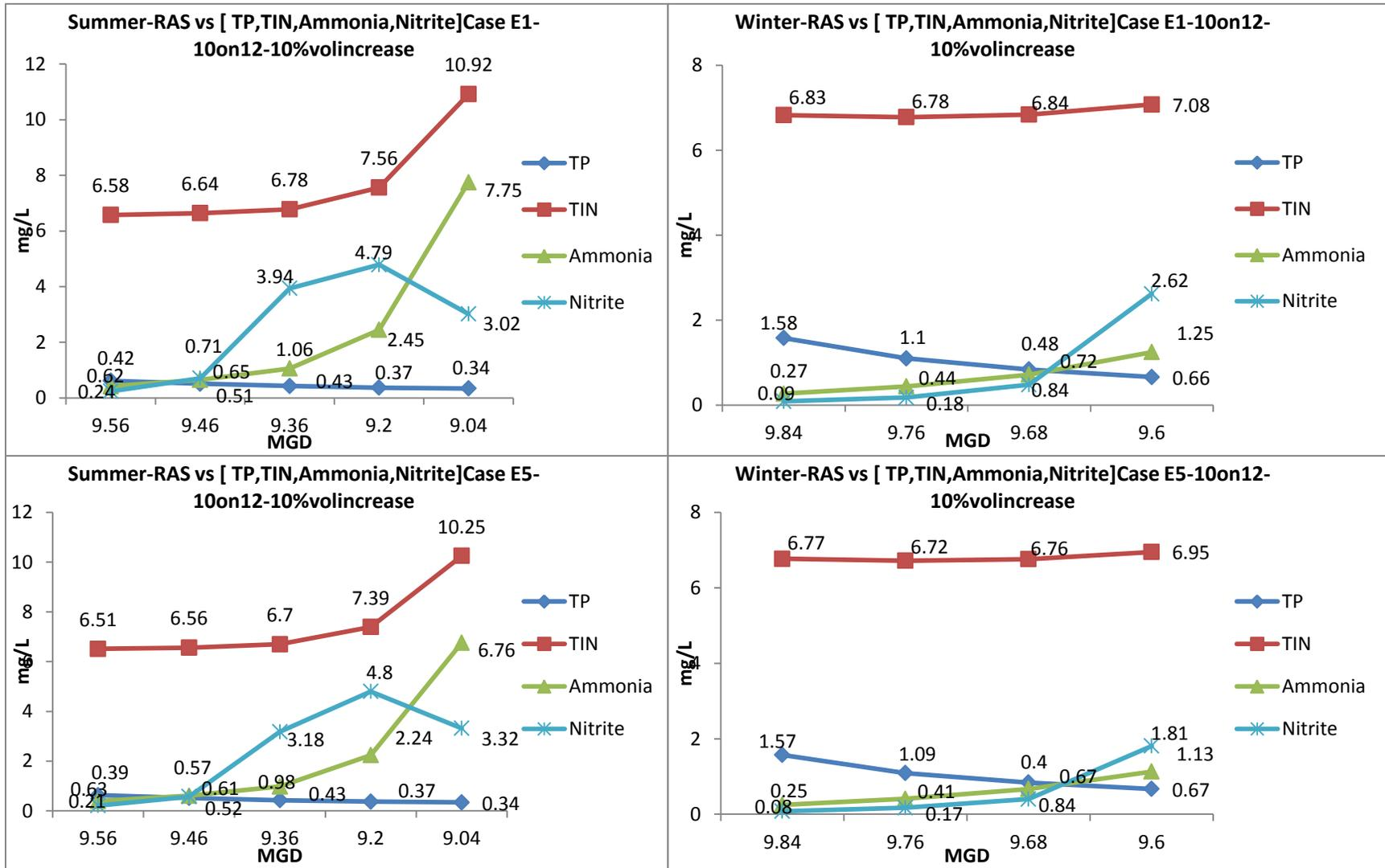
Figure B-3: Effluent concentrations for 10 MGD influent flow in reactors with 10 % increase in volume for summer and winter conditions, 10 MGD internal recycle Cases E1 and E5
