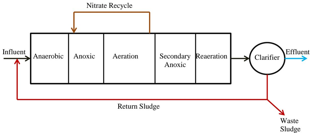
Figure 4.5: Flow diagram of 5-stage Bardenpho process
