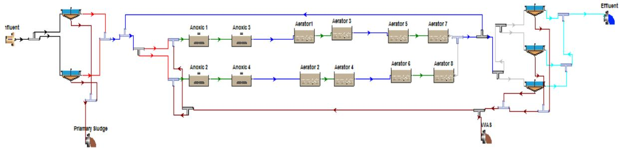
Figure A-1: BioWin model of A/O process configuration
