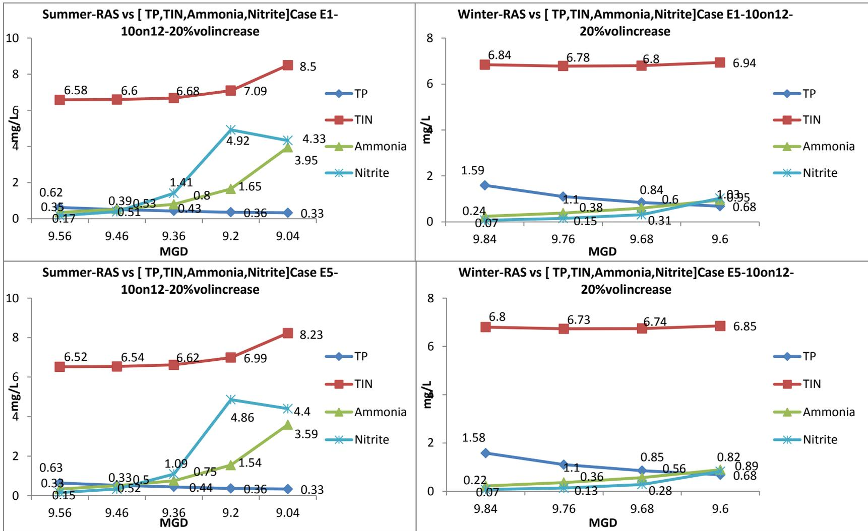
Figure B-9: Effluent concentrations for 10 MGD influent flow in reactors with 20 % increase in volume for summer and winter conditions, 10 MGD internal recycle Cases E1 and E5
