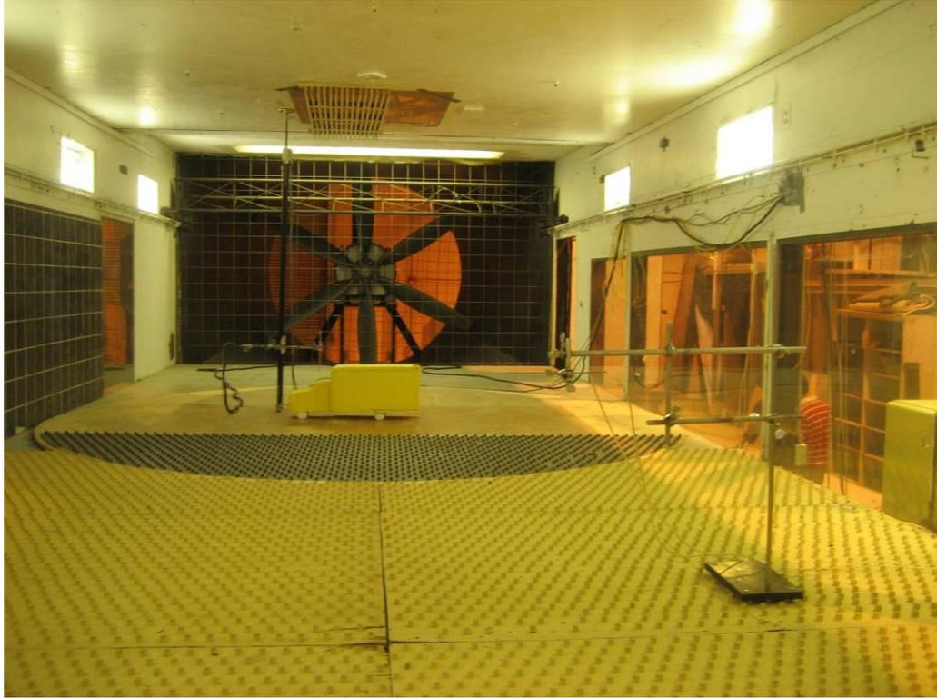
Fig. 2.8 Wind tunnel and the test section
