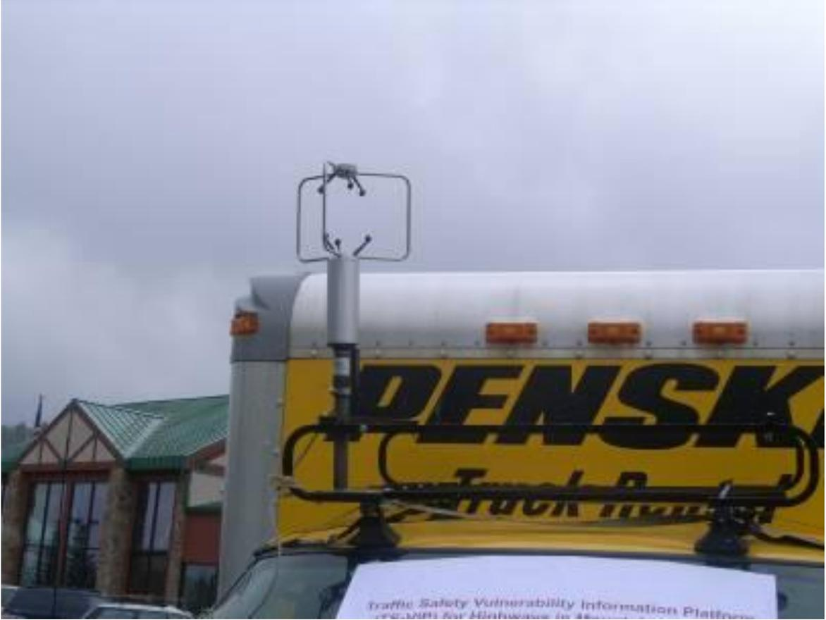
Fig. 2.1 3-D sonic anemometer installed on testing vehicle
