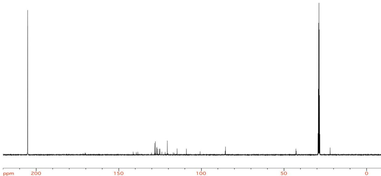
**Figure A1.1b**  $^{13}\text{C}$ -NMR spectrum (101 MHz; acetone- $\text{d}_6$ ) of compound **2.118a**
