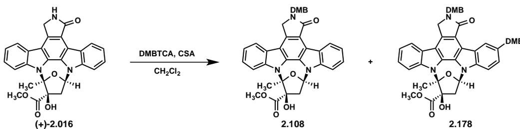
A 1 mL micro reaction vial with a septum cap was charged with (+)-**2.016** (0.0095 g, 0.02 mmol, 1 equiv) and CSA (0.0005 g, 0.002 mmol, 0.1 equiv) in  $\text{CH}_2\text{Cl}_2$  (0.3 mL, 0.07M). A solution of DMBTCA (0.0070 g, 0.022 mmol, 1.1 equiv) in  $\text{CH}_2\text{Cl}_2$  (0.1 mL) was added dropwise via syringe, followed by the remaining  $\text{CH}_2\text{Cl}_2$  (0.1 mL, 0.04 M). After being allowed
