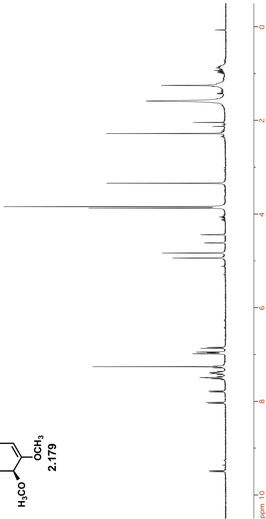
Figure A2.4a <sup>1</sup>H-NMR spectrum (400 MHz; CDCl<sub>3</sub>) of compound 2.179
