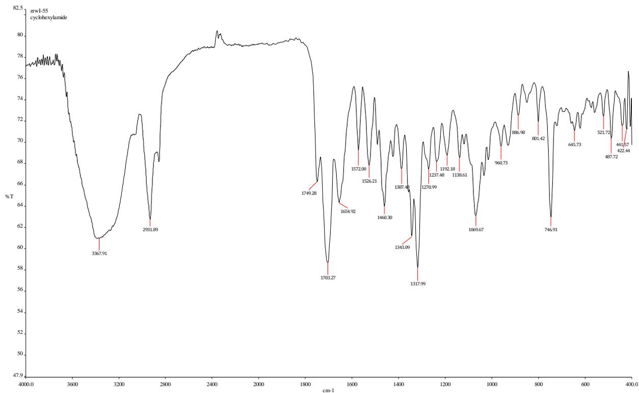
**Figure A1.2c** IR spectrum of compound **2.118d**
