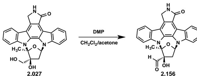
In a 25 mL, 2-neck, round-bottomed flask, **2.027** (0.0439 g, 0.1 mmol, 1 equiv) was dissolved in a mixture of  $\text{CH}_2\text{Cl}_2$  (5 mL, 0.02 M) and acetone (3 mL, 0.03M). The Dess-Martin
