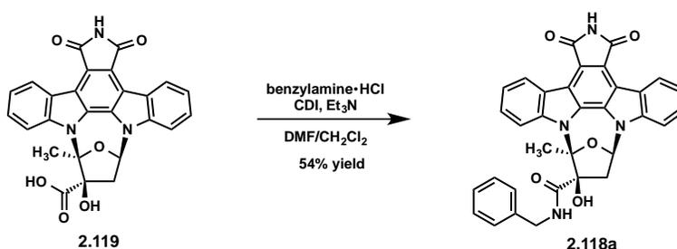
In a 2-neck 25 mL round bottom flask, **2.119** (0.0108 g, 0.023 mmol, 1 equiv) was dissolved in DMF (0.9 mL).  $\text{CH}_2\text{Cl}_2$  (2.6 mL) was then added, followed by CDI (0.0101 g, 0.062 mmol, 2.7 equiv). After 95 min  $\text{Et}_3\text{N}$  (0.036 mL, 0.26 mmol, 11.6 equiv) was added, followed by
