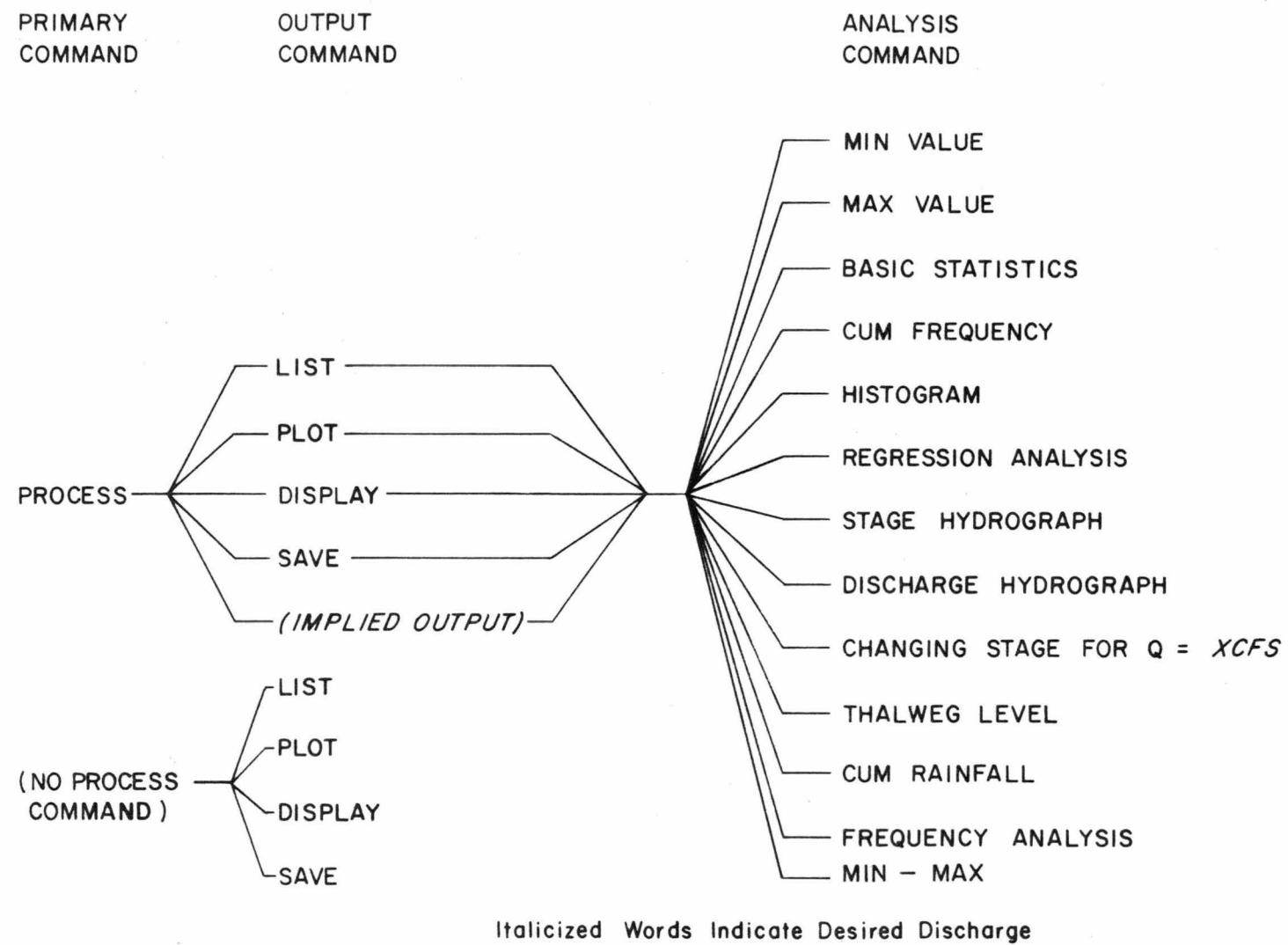
Figure 4. Flow chart for "PROCESS" and "OUTPUT" command
