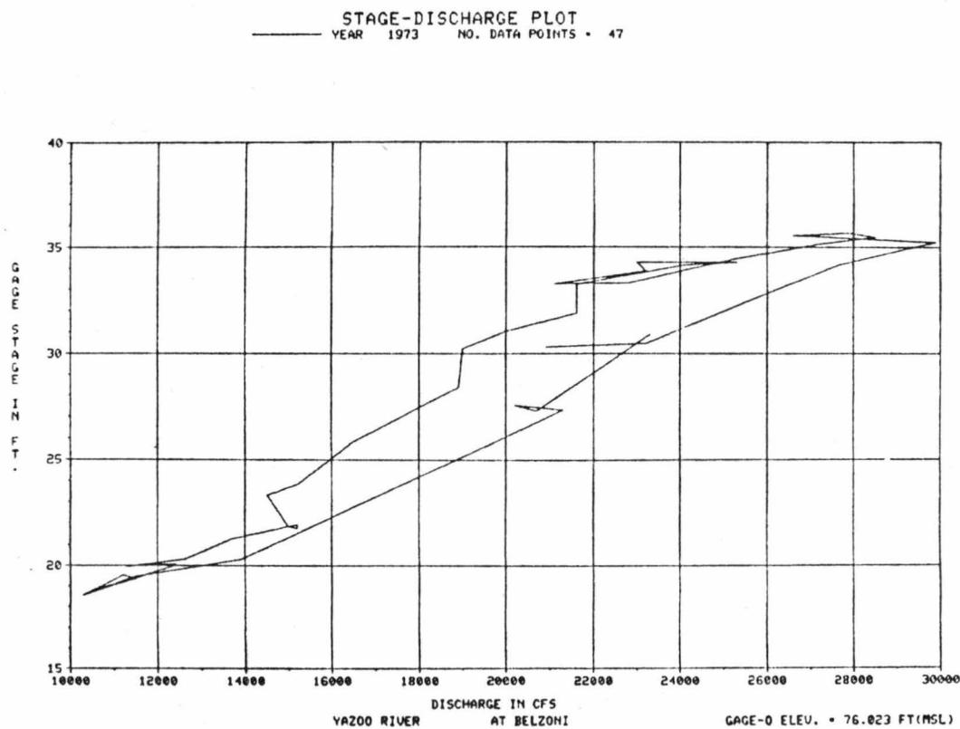
EXAMPLE 6: Stage-discharge plot for a gaging station for less than five years.
