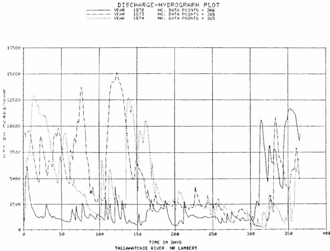
EXAMPLE 33: Discharge data for a gaging station for a specified date.
