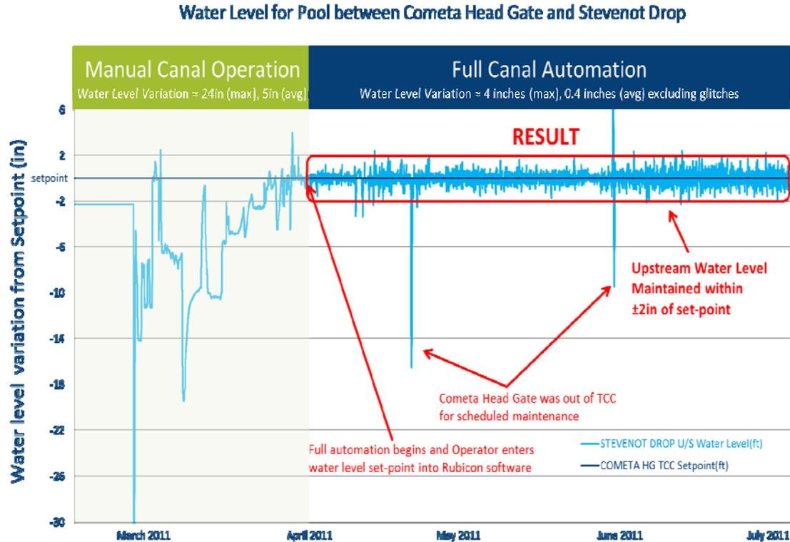
Figure 4. Water Level on the Cometa Canal after TCC Implementation
