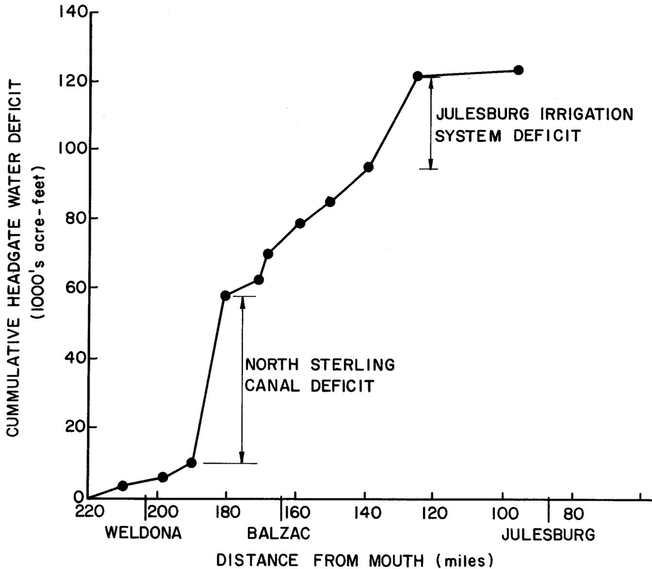
Figure 3-6. Cumulative headgate water deficiencies with distance along river in the Narrows service area (plotted from data in Table 3-8). Multiply abscissa scale in miles by 1.609 to obtain kilometers.
