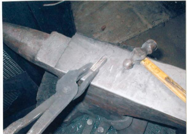
If forging by hammer is *focused* striking compression between two concentrated points (hammer and anvil), then the use of the hydraulic press is the *consistent* overall compression within two planes.
