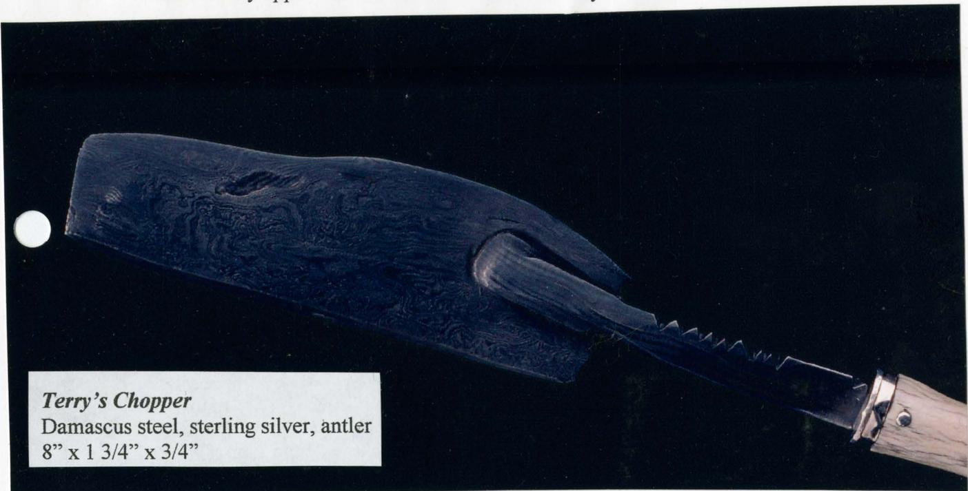
Acids like nitric or ferric play an important role in the development and final appearance of Damascus steel. The steel with the higher amount of carbon tends to resist the acid, retaining its solid surface integrity. The steel with lesser carbon receives an acid “bite” and gets eaten away at its surface level. The undulating surface is the result of the various rates of steel resistance.
