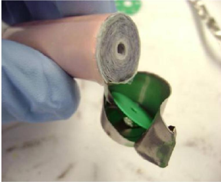
**Figure 10: Tightly wound electrodes in 18650 cells**
