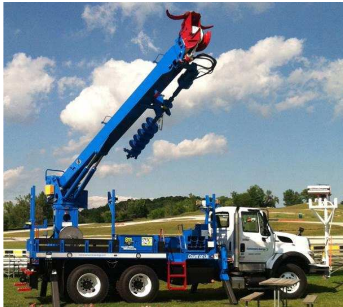
Figure 1.4 – Odyne Truck in Digger Derrick Configuration (from EPRI Report) [15]
