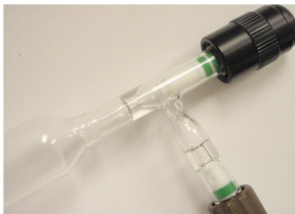
**Figure 2.1.** Glass reactor used for homogeneous reactions with  $C_{60}$  with capability to monitor reaction progress via sampling through side arm.
