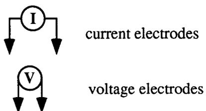
A Schlumberger array consists of two voltage electrodes placed a distance 'a' apart, and two current electrodes, one on either side of, and a distance 'na' (some multiple 'n' of 'a') from of the voltage electrodes. A Schlumberger depth sounding entails changing the position of the current electrodes (changing 'n'); the farther they are apart, the deeper the measurement, the closer they are together, the shallower the measurement.
