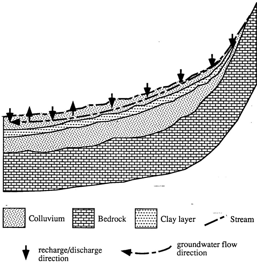
This conceptual model of the area is similar to the previous two with the exception of the existence of layering within the colluvium. Here, there is an impermeable clay layer a few feet down in the colluvium, causing the recharge from precipitation to form a perched aquifer in the colluvium that feeds the stream when it becomes saturated to the ground surface.
