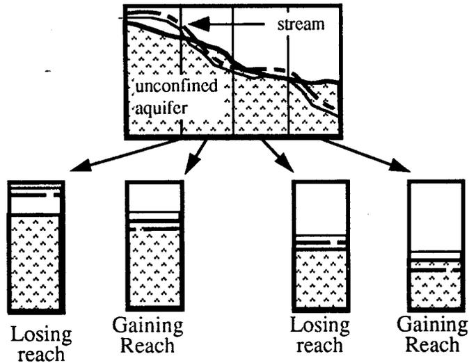
narrower cells reduce axial averaging, decreasing the amount of blending of losing and gaining reaches
