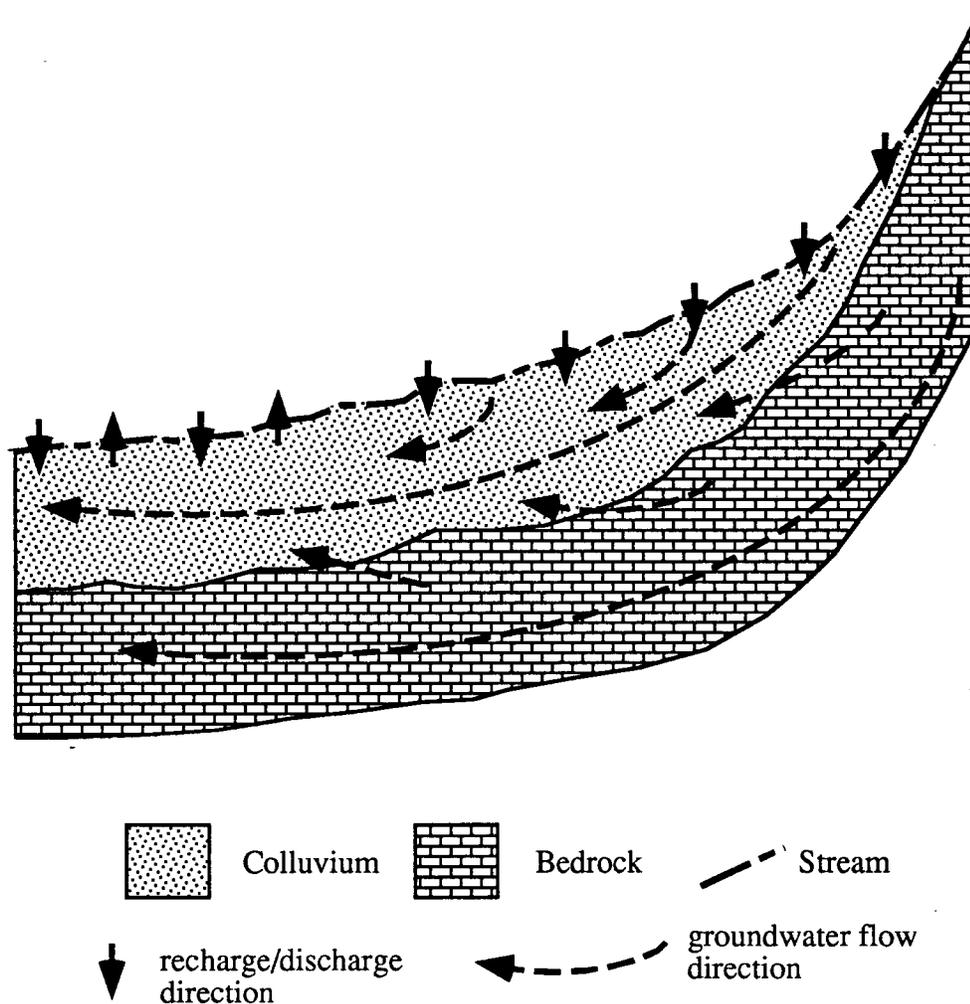
This conception of the area is the same as that of conceptual model #1, except that in this case the bedrock is not assumed to be impermeable so recharge can enter the colluvium from the bedrock (as shown), or recharge can leave the colluvium via the bedrock.
