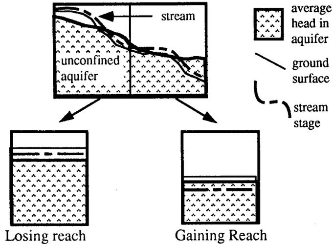
wide grid cells average actual field conditions, with the possibility of blending losing and gaining portions of a stream together in one reach
