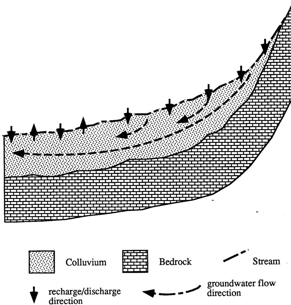
This conceptual model was the one used in the modeling of this project. It assumes an impermeable boundary at the bedrock surface, thus all recharge originates from precipitation. Water flows down the mountain side through the colluvium, and when the aquifer becomes saturated and the water table reaches the ground surface, water from the aquifer discharges into the streambed causing flow through in the stream.
