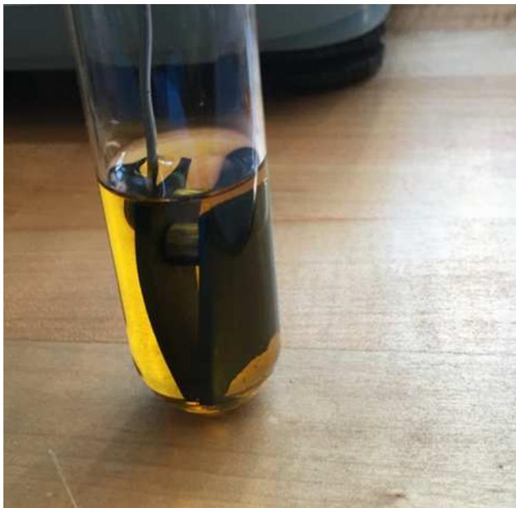
**Figure 3.10:** Discoloration of iP-1-iP due to NBR leaching
