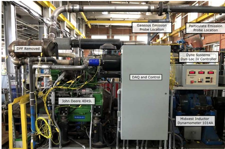
**Figure 3.13:** Deere 4045 4.5L Tier 3 diesel engine used in this testing
