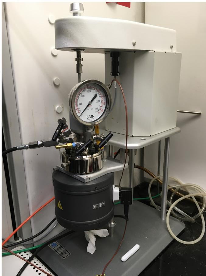
**Figure 2.1:** Parr reactor used for this work
