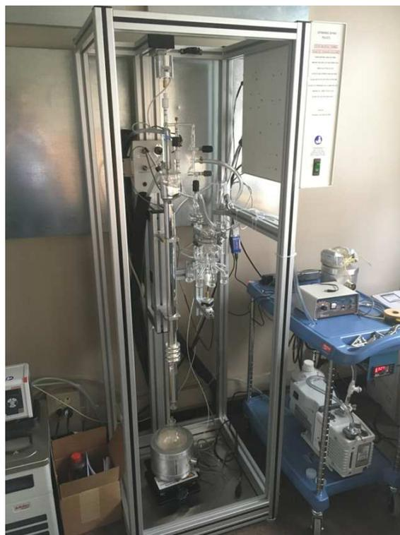
**Figure 2.15:** B/R Instruments 36/100 spinning band distillation column
