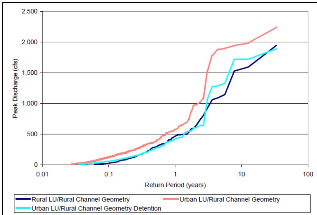
**Figure 2-8: Effects of detention on peak flow frequency exceedance curves in Morgan Watershed with rural channels. (Source: Pomeroy, 2007)**
