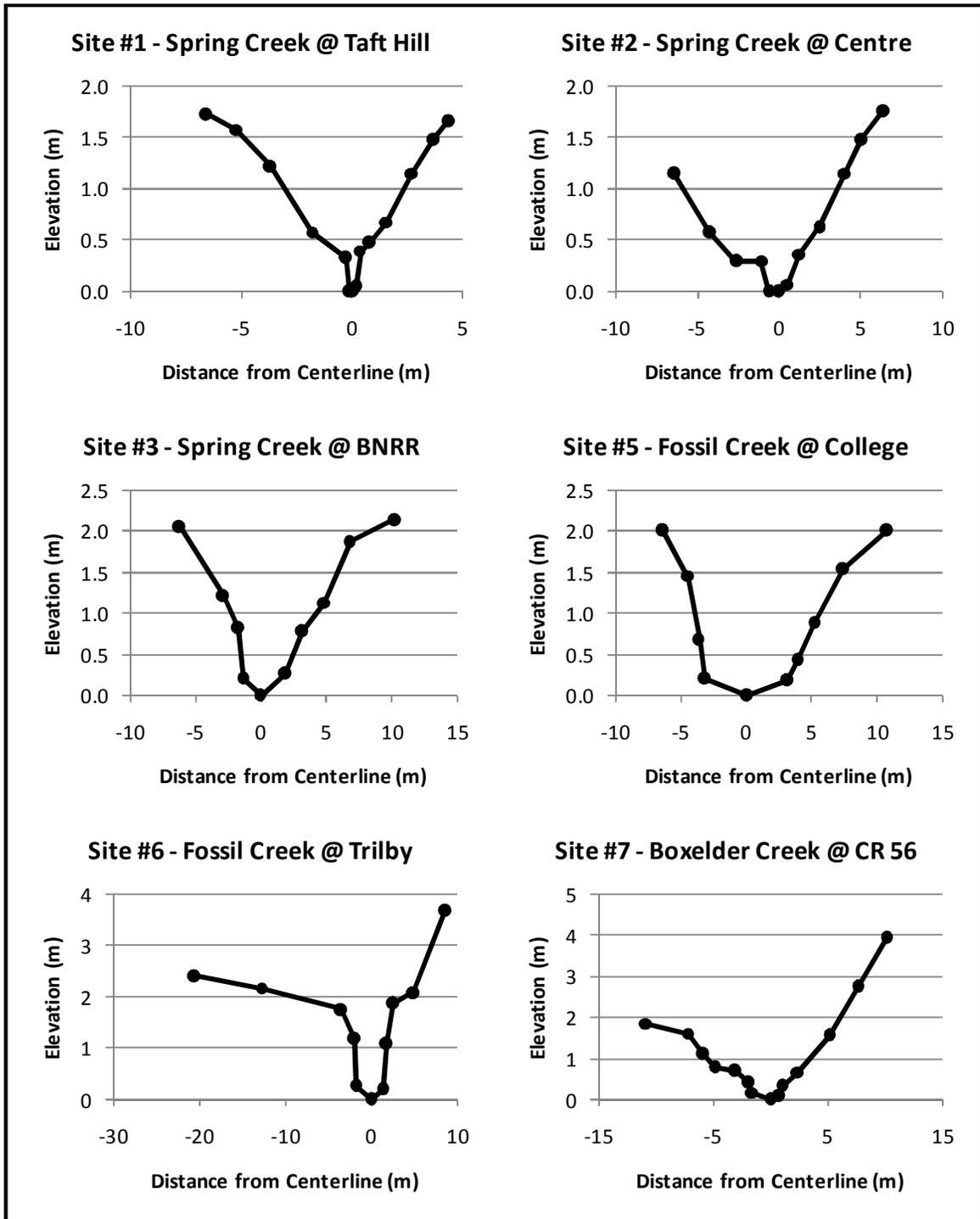
Figure 8-1: Surveyed channel cross-sections for calculation of boundary shear stress at stream gage locations in Fort Collins, Colorado.
