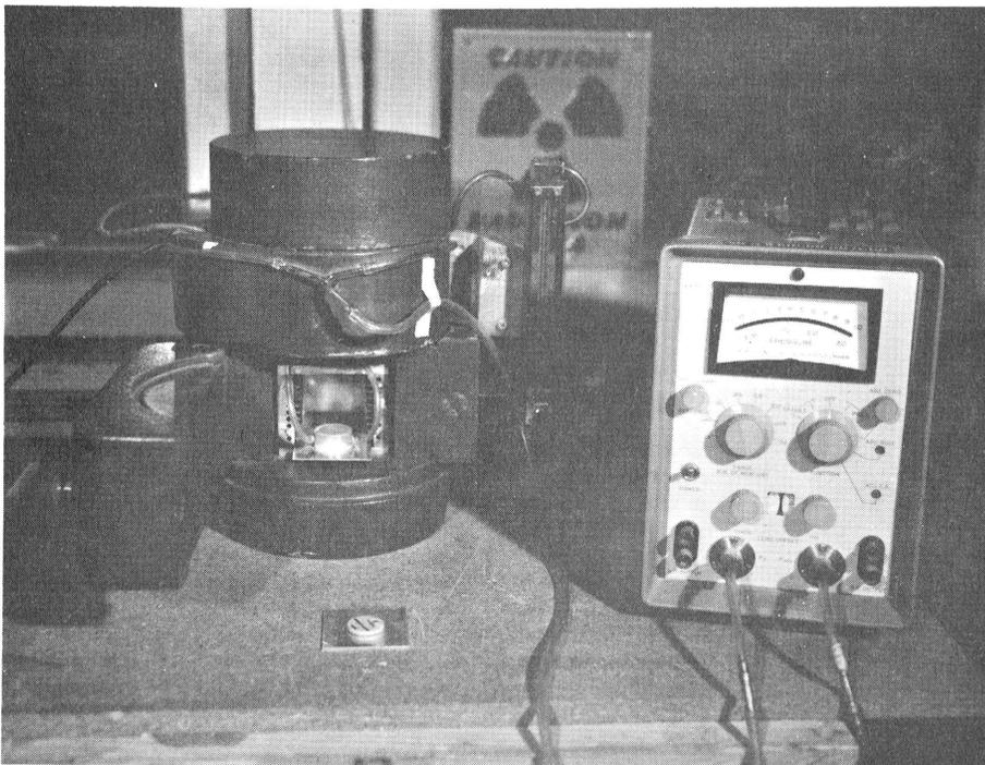
Figure 8 Krypton-85 calibration arrangement.
