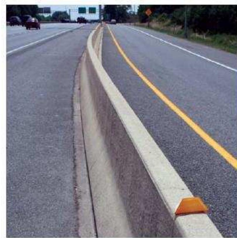
**Figure 6: Rigid Barrier System: Concrete (Source: [safety.fhwa.dot.gov](http://safety.fhwa.dot.gov))**
