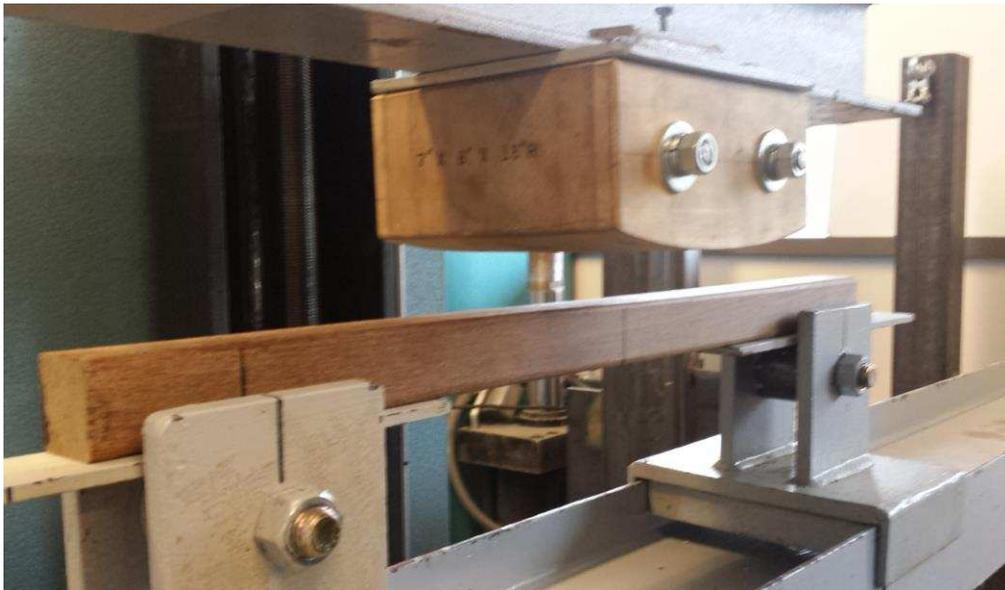
**Figure 12: Instron UTM with Loading Mechanism and Ipe Specimen**
