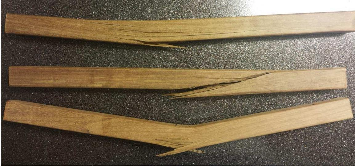
**Figure 14: Ipe 3-pt Bending Specimens. (1 on top, 3 on bottom)**
